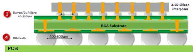
Cross-section: w/ BGA substrate
