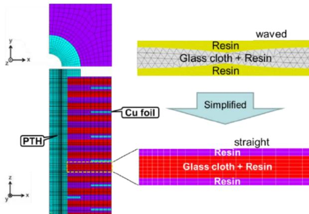
Figure 2 – Simplified model of PWB material
