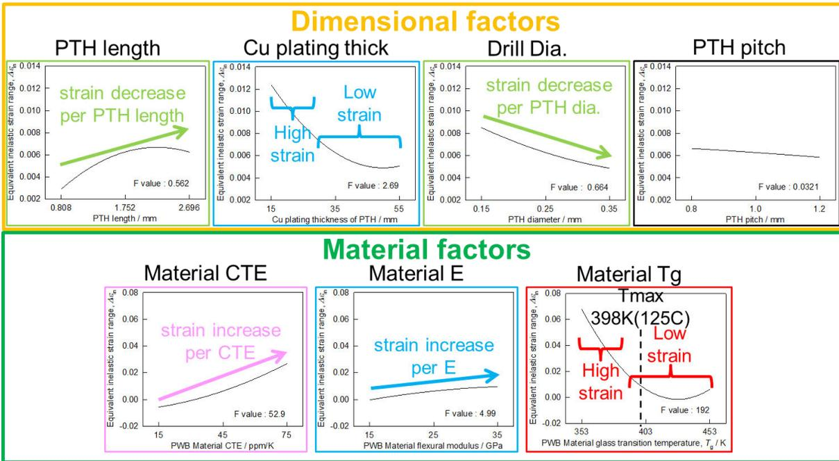
Figure 9 – 1<sup>st</sup> investigation single factor effect results (Temp. condition 2)
