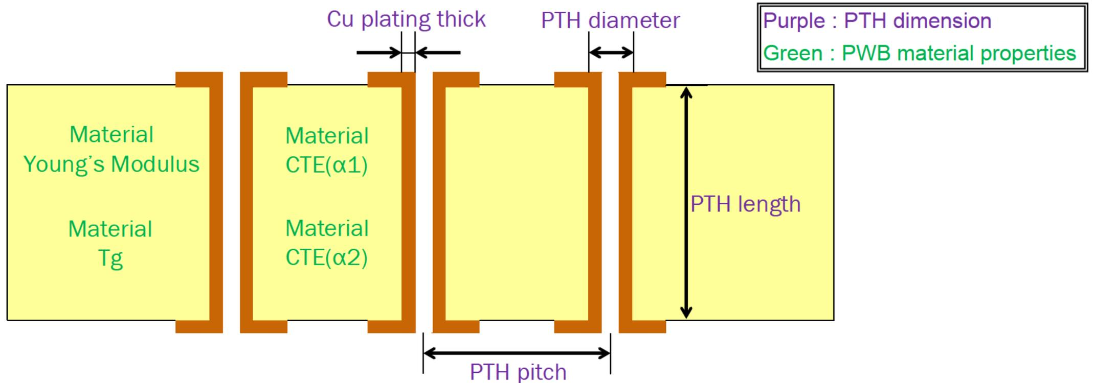
Objective : calculate the number of cycles to failure from these factors
