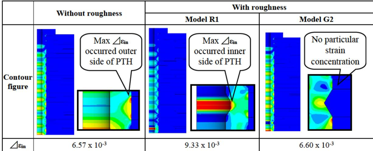
Figure 16 – Contour figures according to roughness shape
