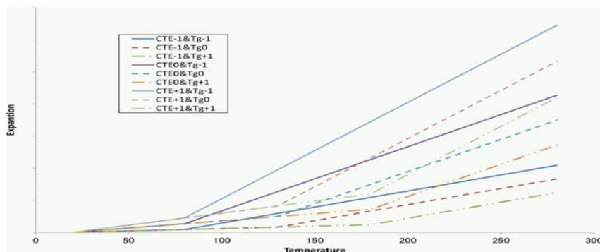
Figure 5 – 9 levels of PWB material CTE and Tg
