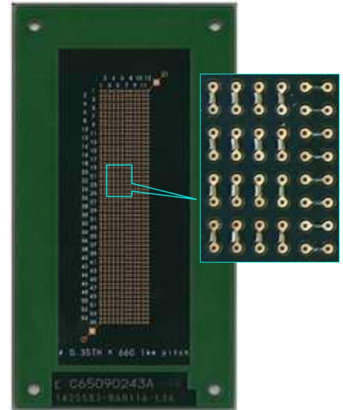
660 PTHs connected in daisy chain for monitoring loop resistance during test
