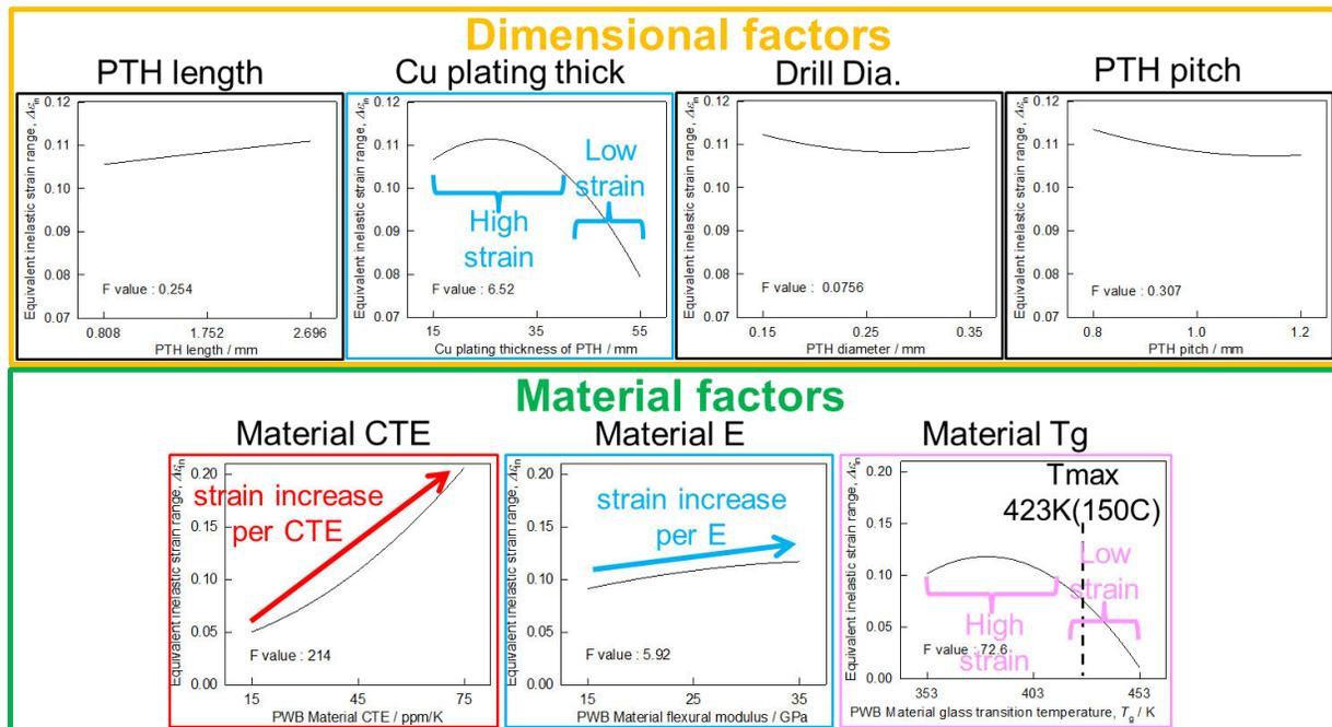
Figure 8 – 1<sup>st</sup> investigation single factor effect results (Temp. condition 1)
