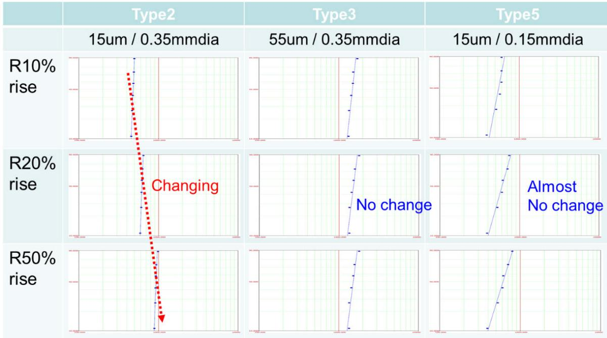
Figure 24 – Weibull Plot for Harsh Condition TCT
