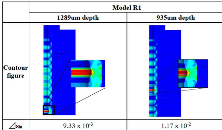
Figure 17 – Contour figures according to roughness position
