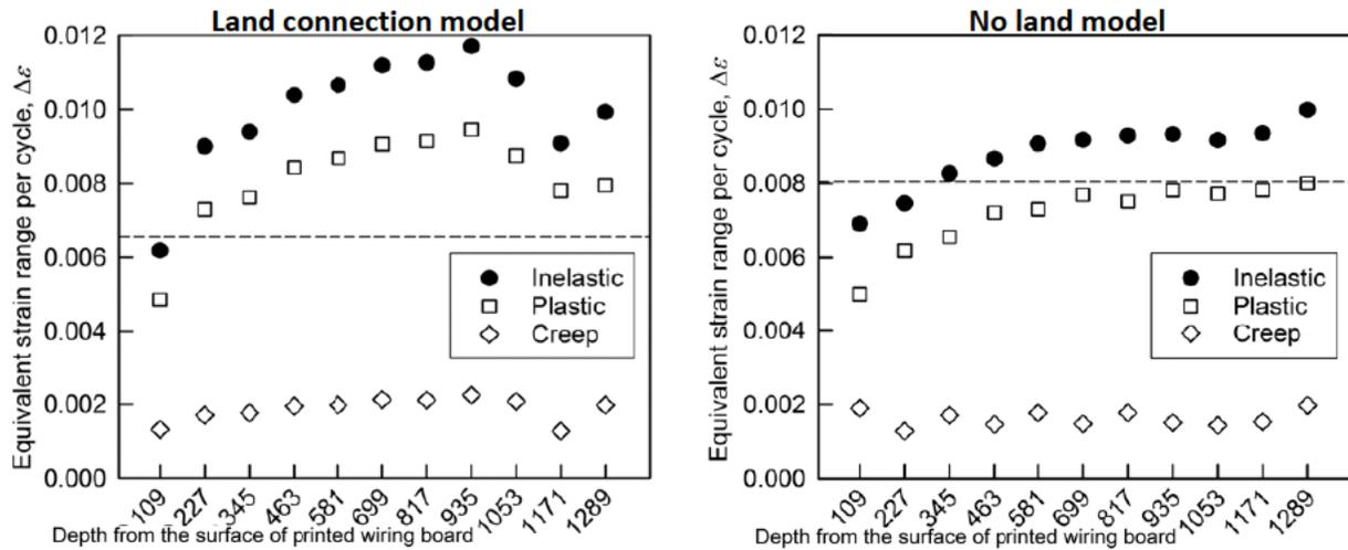
Figure 18 –  $\Delta\epsilon_{in}$  according to position with/without land connection
