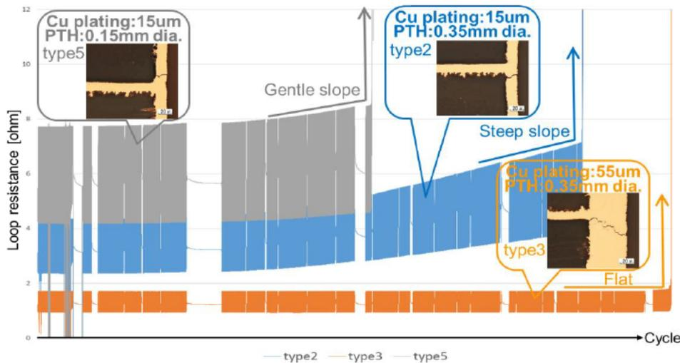
**Figure 23 – Monitored resistance profiles**
