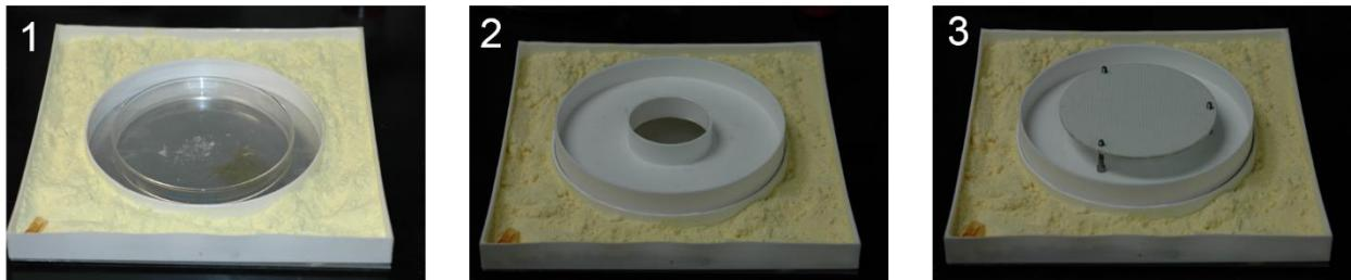
**Figure 2: Bleach setup in cross section and in pictorial format. The moisture coming off the bleach is forced to flow through a 1-mm gap and then over a saturated salt solution so that the air exiting the setup is in equilibrium with the saturated salt solution. The saturated salt solution, thus, controls the humidity of the air in the chamber**
