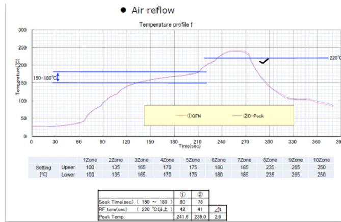
**Figure 6 Air reflow thermal couple readout (i.e. reflow profile) that was attached to one solder joint of each component (QFN and DPAK) on the TV-2 circuit board.**
