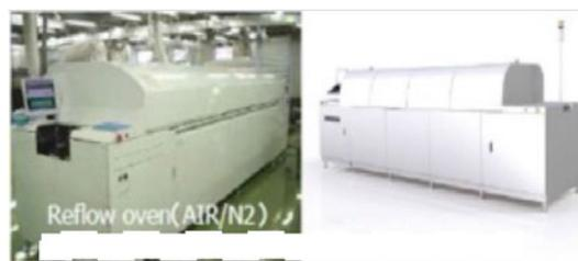
**Figure 11 Production convection air reflow oven (left) and production vacuum reflow oven (right) used for the DOE.**
