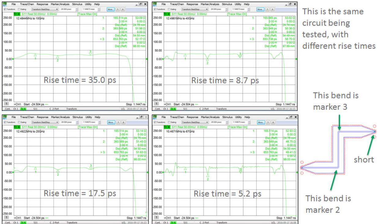
Figure 7. Impedance curves (green curves) for a stripline circuit with two right-angle bends in the conductor routing made using vector analyzers with different rise times.
