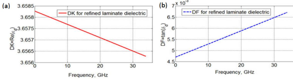
Figure 3–DK (a) and DF (b) of PCB Substrate (PPO Blend) Dielectric.
