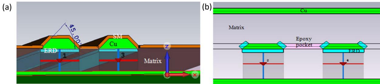
**Figure 2 - Cross-sections of Modeled Microstrip (a) and Stripline (b) Differential Pairs**
