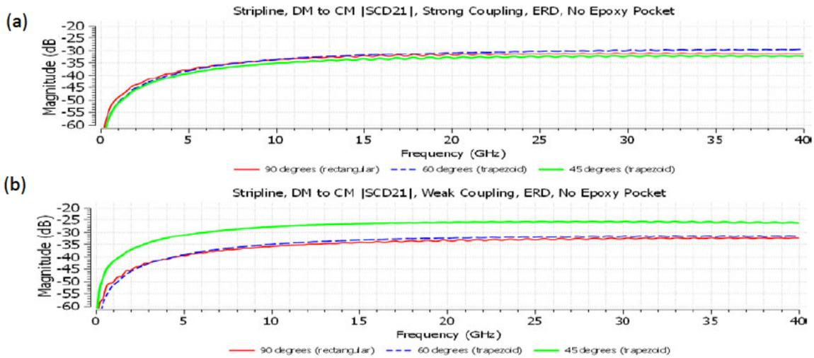
**Figure 17– Insertion Loss for Mode Conversion in an Imbalanced (5 mil) Stripline Pair with 90°, 60°, and 45° Traces at Strong (a) and Weak (b) Coupling.**
