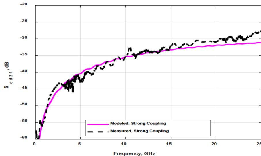
**Line lengths are 80 mm and 80.127 mm (5 mil length imbalance)**
