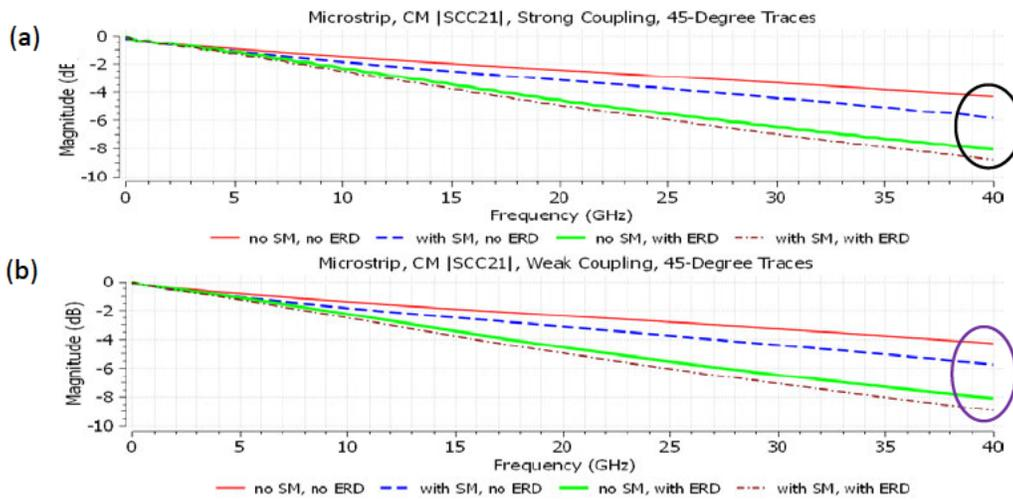
**Figure 10– Insertion Loss for Common Mode in an Imbalanced (5 mil) Microstrip Pair with 45° Traces at Strong (a) and Weak (b) Coupling**
