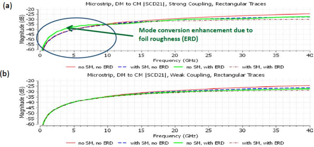
**Figure 6– Insertion Loss for Mode Conversion in an Imbalanced (5 mil) Microstrip Pair with Rectangular Traces at Strong (a) and Weak (b) Coupling**
