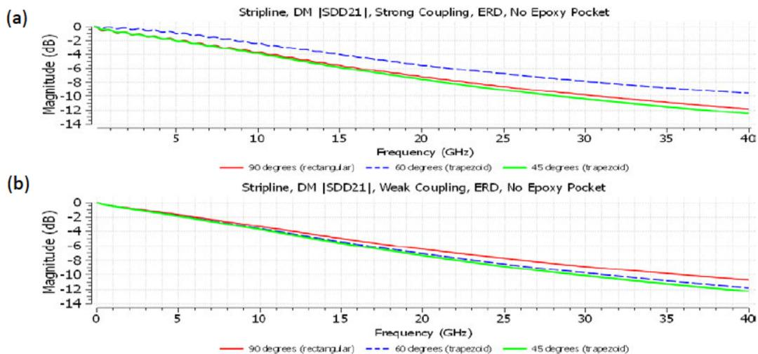
**Figure 15– Insertion Loss for Differential mode in an Imbalanced (5 mil) Stripline Pair with 90<sup>0</sup>, 60<sup>0</sup>, and 45<sup>0</sup> Traces at Strong (a) and Weak (b) Coupling.**
