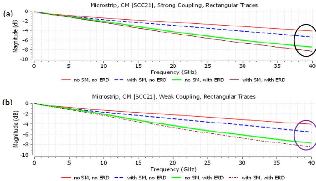
**Figure 4– Insertion Loss for Common Mode in an Imbalanced (5 mil) Microstrip Pair with Rectangular Traces at Strong (a) and Weak (b) Coupling**
