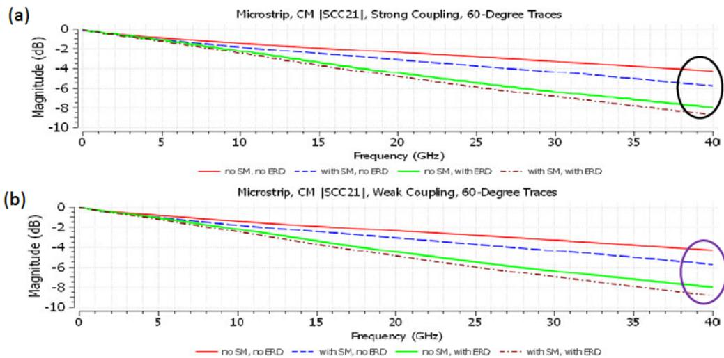
**Figure 7– Insertion Loss for Common Mode in an Imbalanced (5 mil) Microstrip Pair with 60° Traces at Strong and Weak Coupling**
