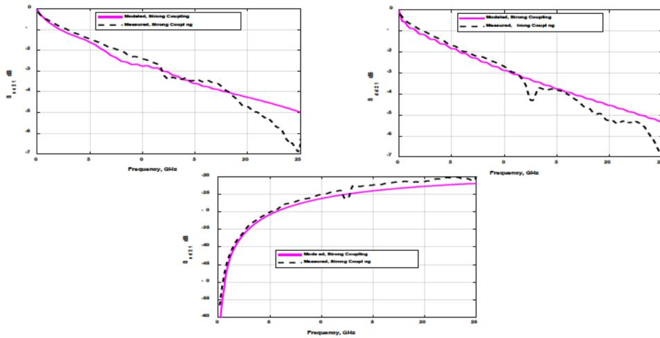
**Figure 22– Measured and Modeled Insertion Loss for CM, DM, and Mode Conversion in an Imbalanced (5 mil) Stripline Pair with 60° Traces at Strong Coupling (ERD and SM Modeled).**
