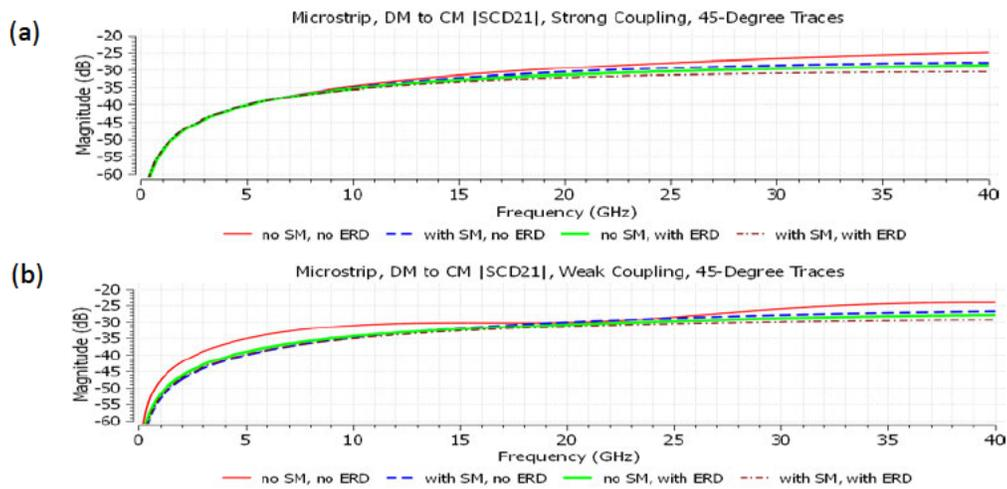
**Figure 12– Insertion Loss for Mode Conversion in an Imbalanced (5 mil) Microstrip Pair with 45° Traces at Strong (a) and Weak (b) Coupling**
