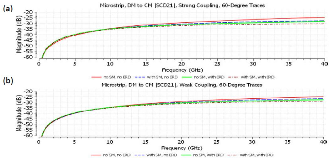
Figure 9– Insertion Loss for Mode Conversion in an Imbalanced (5 mil) Microstrip Pair with 60° Traces at Strong (a) and Weak (b) Coupling
