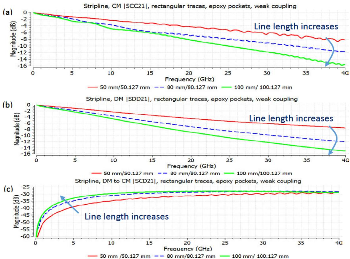
**Figure 19– Insertion Loss for CM (a), DM (b), and Mode Conversion(c) in an Imbalanced (5 mil) Stripline Pair with Rectangular Traces at Weak Coupling. ERD and Epoxy pocket are Modeled.**
