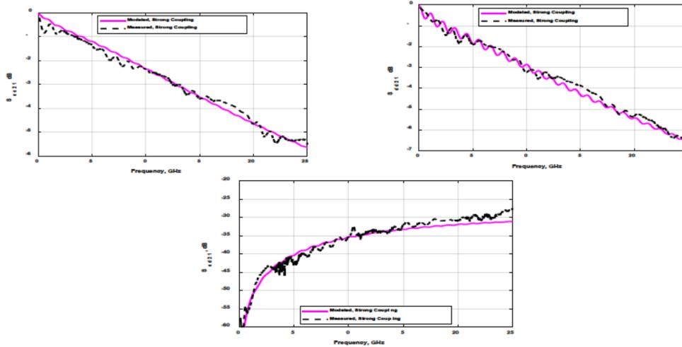
**Figure 20– Measured and Modeled Insertion Loss for CM, DM, and Mode Conversion in an Imbalanced (5 mil) Microstrip Pair with 45° Traces at Strong Coupling (ERD and SM Modeled).**
