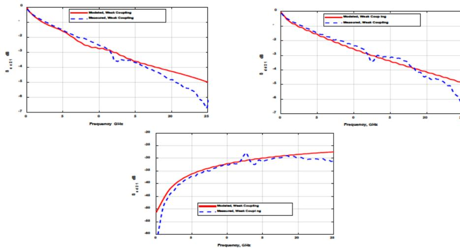
**Figure 23– Measured and Modeled Insertion Loss for CM, DM, and Mode Conversion in an Imbalanced (5 mil) Stripline Pair with 60° Traces at Weak Coupling (ERD and SM Modeled).**
