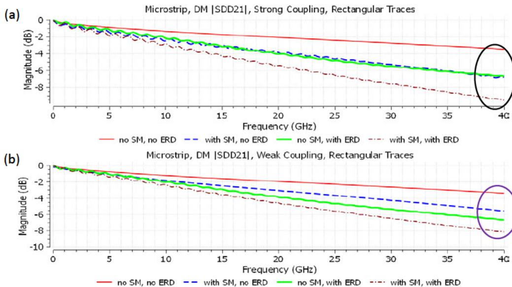
**Figure 5– Insertion Loss for Differential Mode in an Imbalanced (5 mil) Microstrip Pair with Rectangular Traces at Strong (a) and Weak (b) Coupling**
