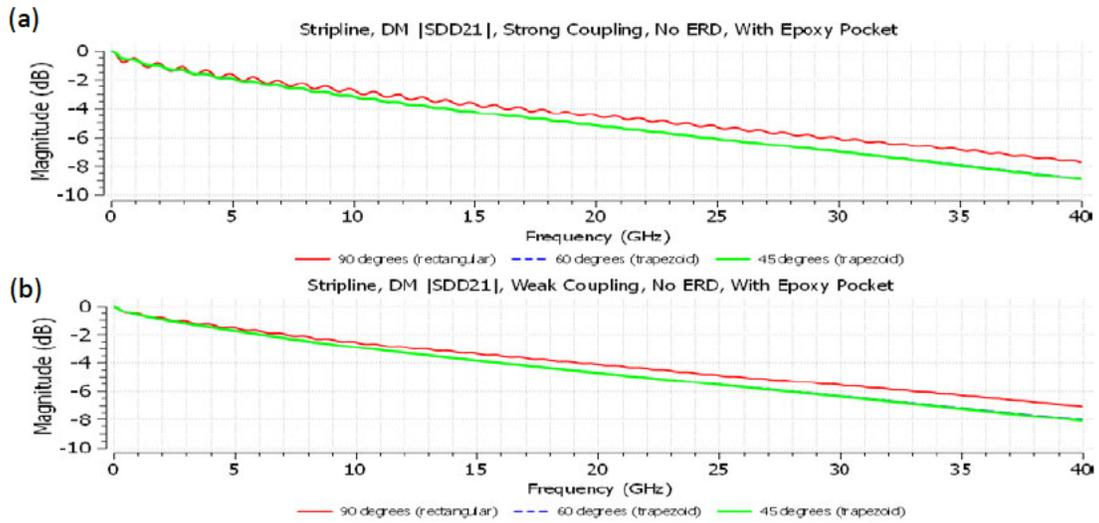
**Figure 16– Insertion Loss for Differential mode in an Imbalanced (5 mil) Stripline Pair with 90°, 60°, and 45° Traces at Strong (a) and Weak (b) Coupling.**
