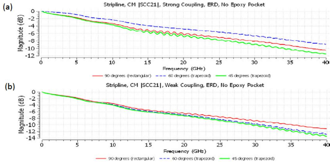
**Figure 13– Insertion Loss for Common mode in an Imbalanced (5 mil) Stripline Pair with 90<sup>0</sup>, 60<sup>0</sup>, and 45<sup>0</sup> Traces at Strong (a) and Weak (b) Coupling.**
