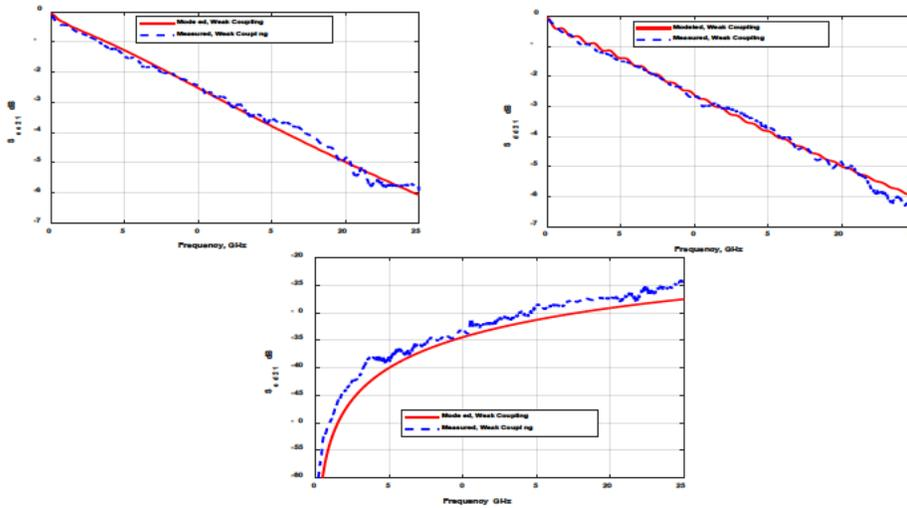
**Figure 21– Measured and Modeled Insertion Loss for CM, DM, and Mode Conversion in an Imbalanced (5 mil) Microstrip Pair with 45° Traces at Weak Coupling (ERD and SM Modeled).**
