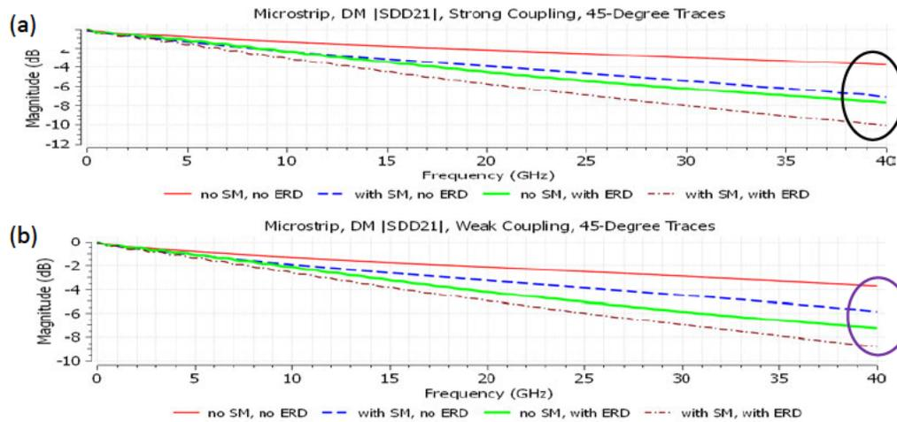
**Figure 11– Insertion Loss for Differential Mode in an Imbalanced (5 mil) Microstrip Pair with 45° Traces at Strong (a) and Weak (b) Coupling**
