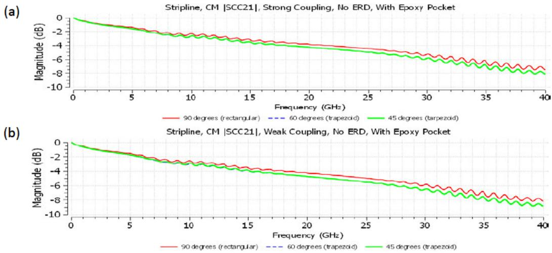
**Figure 14– Insertion Loss for Common mode in an Imbalanced (5 mil) Stripline Pair with 90<sup>0</sup>, 60<sup>0</sup>, and 45<sup>0</sup> Traces at Strong (a) and Weak (b) Coupling.**
