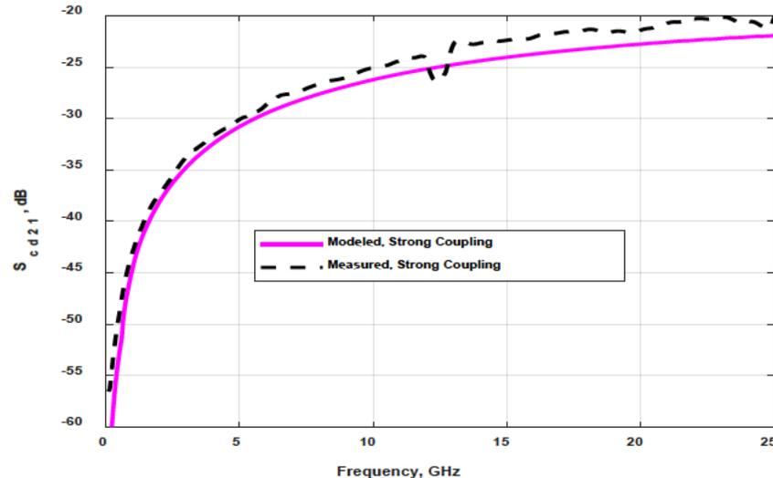
Modeled technological effects: dispersive PPO Blend, ERD, epoxy resin pocket, 60° trapezoid traces
