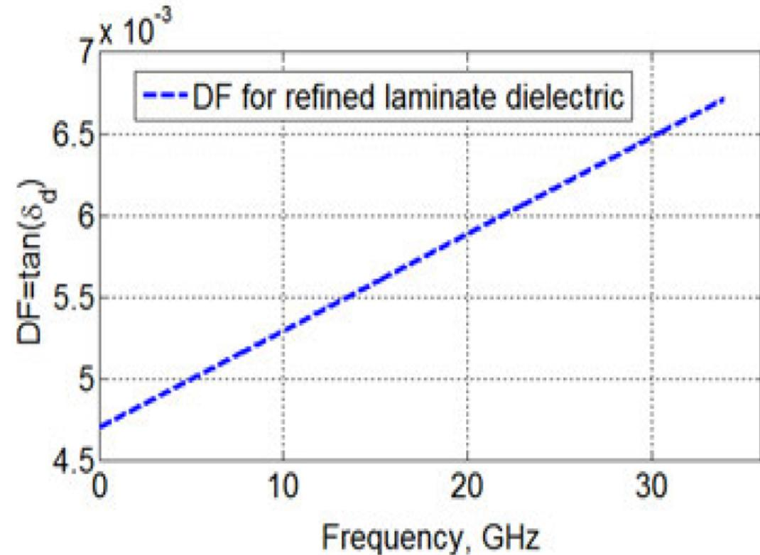
DK and DF of PPO Blend Dielectric extracted using DERM technique
