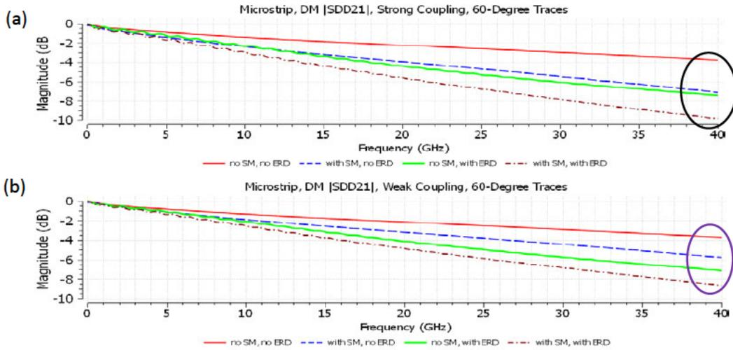
Figure 8– Insertion Loss for Differential Mode in an Imbalanced (5 mil) Microstrip Pair with 60° Traces at Strong (a) and Weak (b) Coupling
