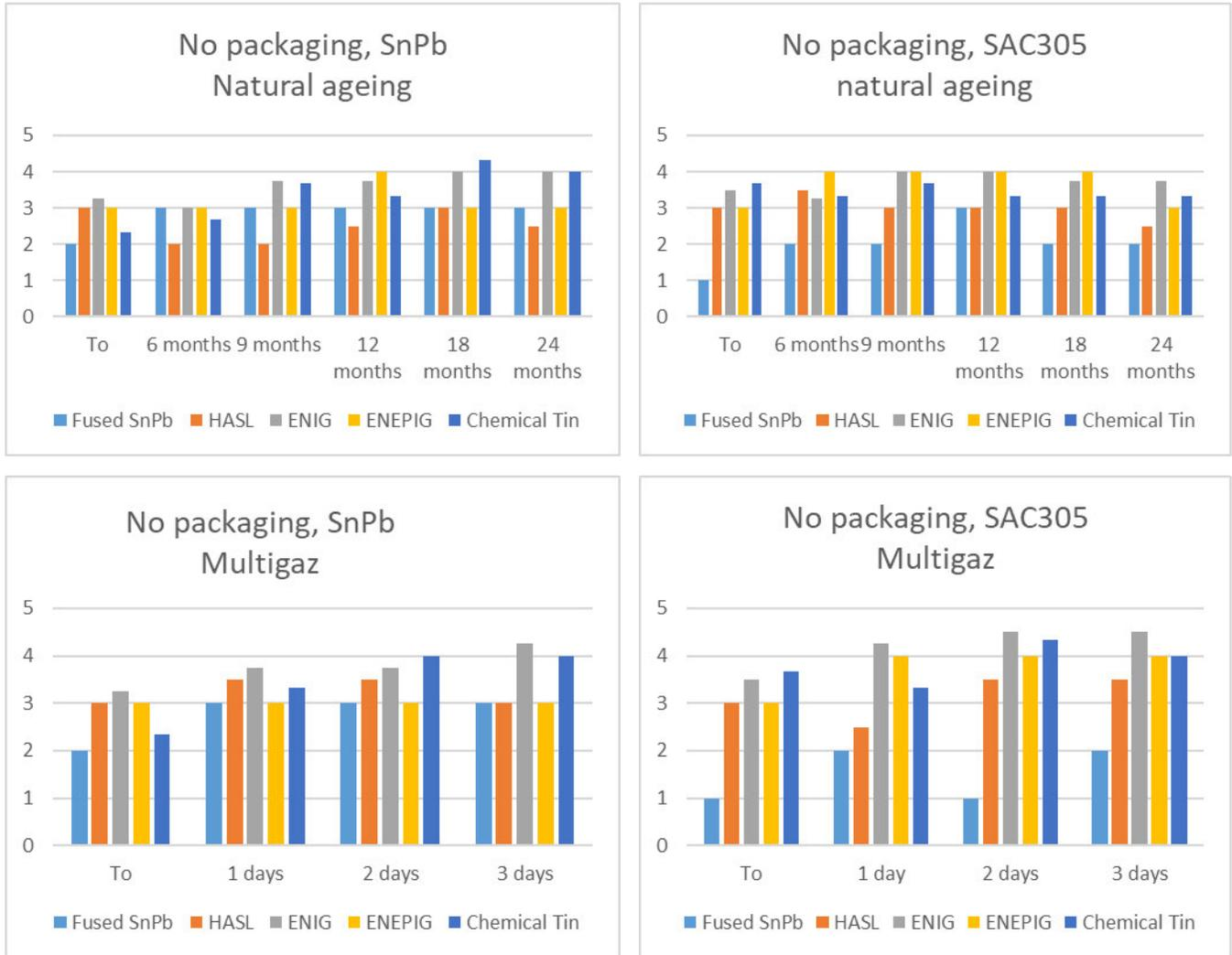
Fig. 11 : No packaging results (Natural ageing and Multi-gas tests). Low values are better solderability. (To= Initial time)
