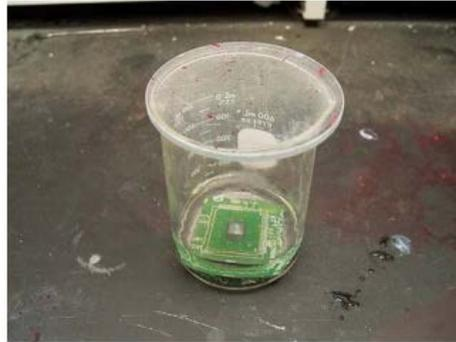
Clean Sample in Liquid Flux-Removing Solvent
