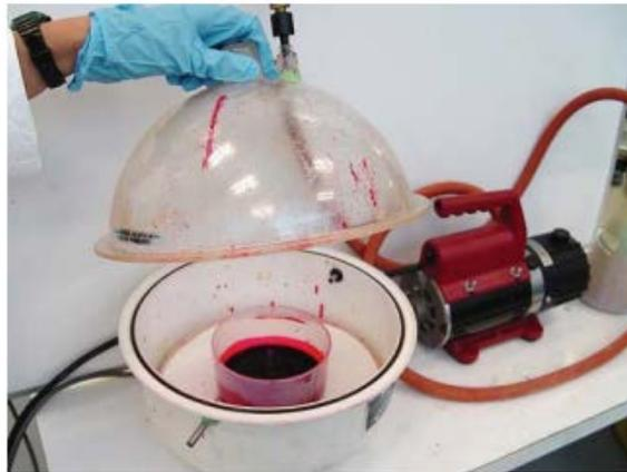
Sample Submerged in Dye
