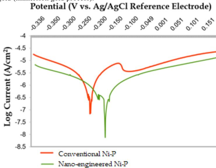
**Figure 5:**Tafel Plots of conventional Ni-P (ENIG) and nano-engineered Ni-P (novel ENIG) surfaces (Ag/AgCl reference electrode; sweeping potential from -400 to +200 mV versus open circuit potential at a scan rate of about 1 mV/sec)
