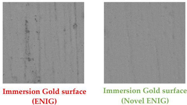
Figure 6: SEM Images (5000x) of gold surface of conventional ENIG and nano-engineered ENIG (Novel ENIG)
