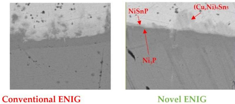
**Figure 8: SEM Images (5000x) of cross-section solder joints for conventional ENIG and novel ENIG**
