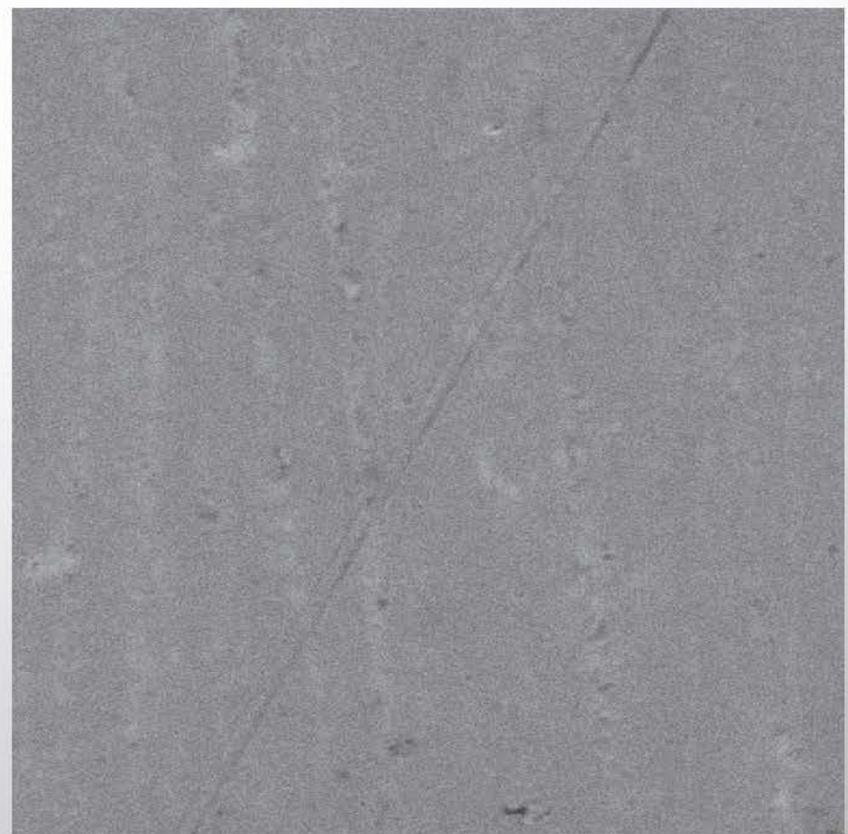
Rough & pitted Ni-P surface for ENIG vs. smooth Ni-P surface for Novel ENIG
