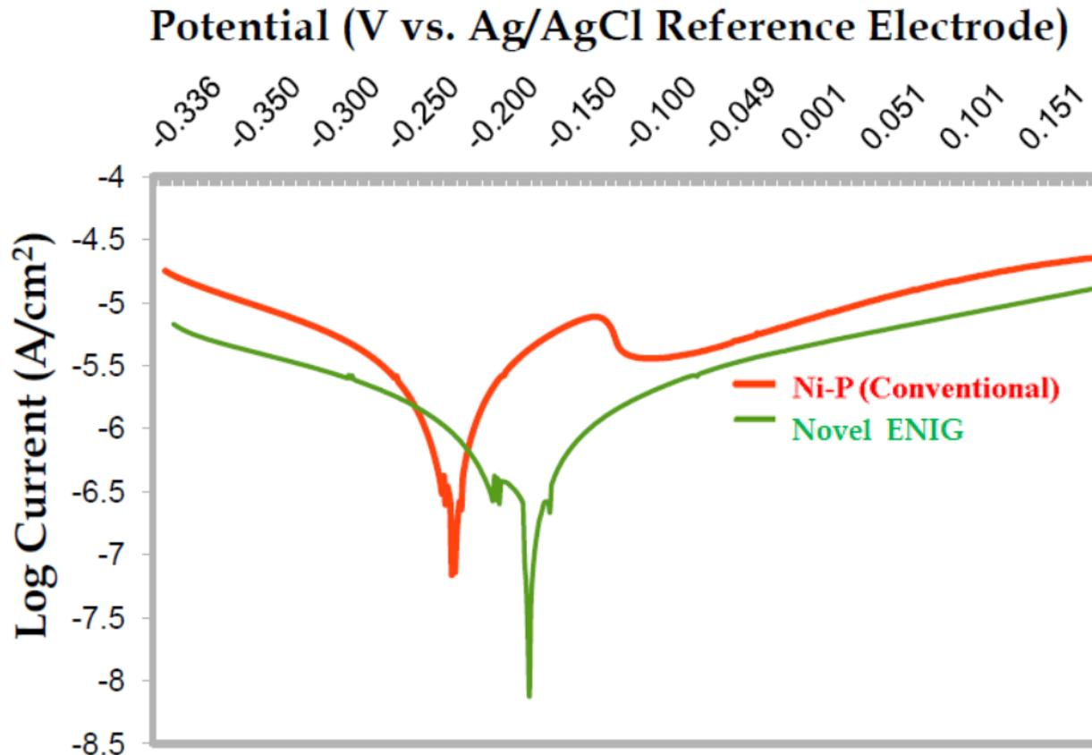
Corrosion current density of Electroless Ni layer of Novel ENIG is ~10X lower than conventional Electroless Ni layer (ENIG)
