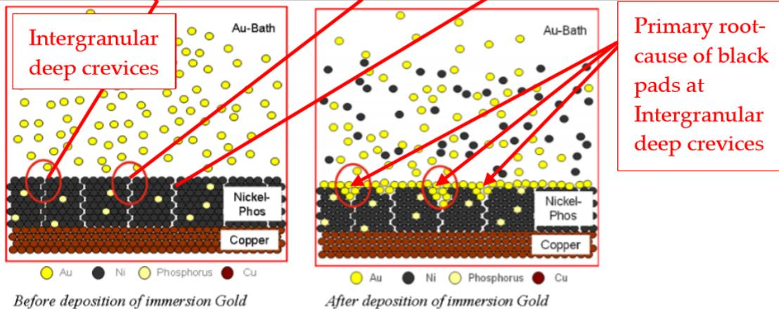
Interfacial nano-engineering at Ni-P surface smoothens and shield the intergranular deep crevices; black pads are eliminated for Novel ENIG
