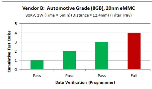
**Figure 8: 3 Cycles Data Pass, 4<sup>th</sup> Cycle Data Fail**
