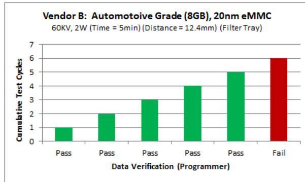
**Figure 9: 5 Cycles Data Pass, 6<sup>th</sup> Cycle Data Fail**
