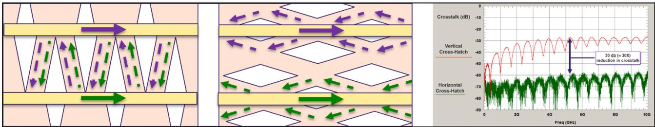
Figure 7: Example of How Changing the Orientation of the Cross-Hatch Pattern Can Significantly Reduce Crosstalk
