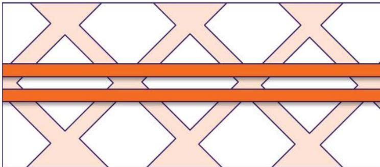
Properly Aligned Traces with Cross Hatch
