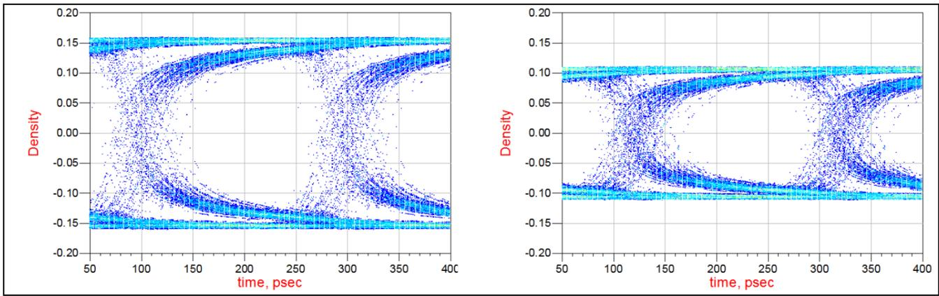
Figure 5: Signal Degradation Due to Trace-to-Cross-hatch Misregistration.
