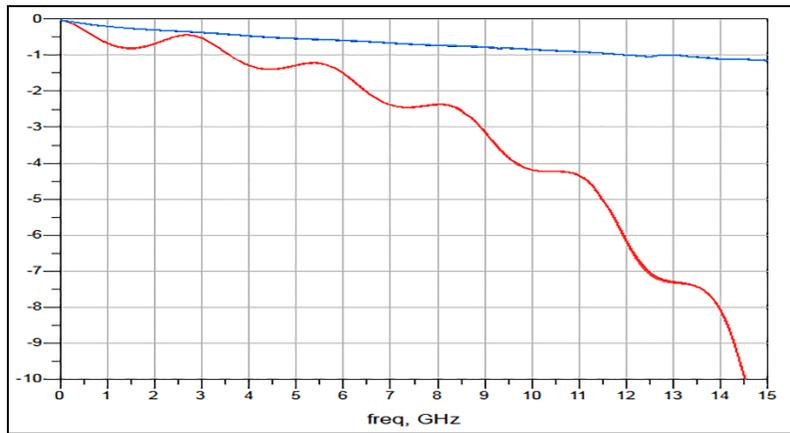
Figure 3: Impact of a Cross-Hatching on Interconnect Loss (dB/inch)
