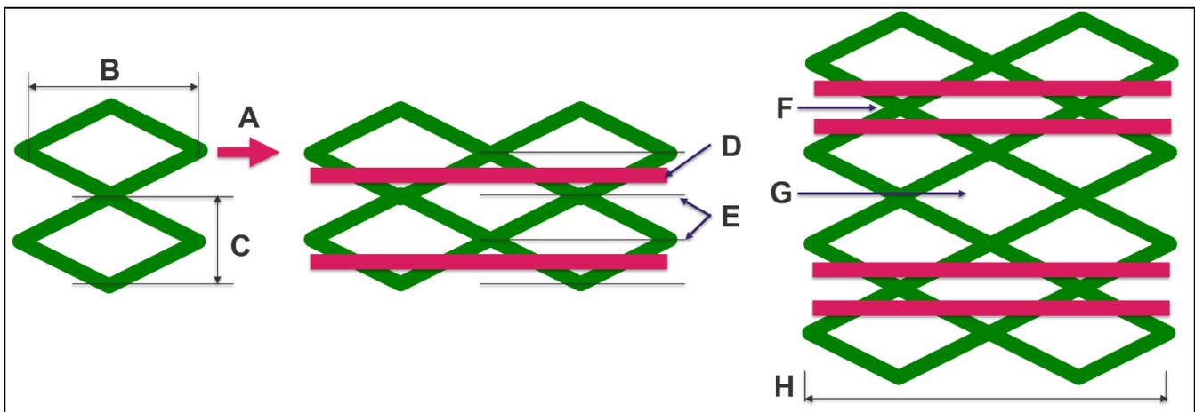
Figure 8: Cross-Hatching Design Guidelines
