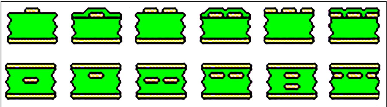
Figure 1: Examples of Micro-Strip-Based (Top Row) and Stripline-Based (Bottom Row) Transmission Line Geometries
