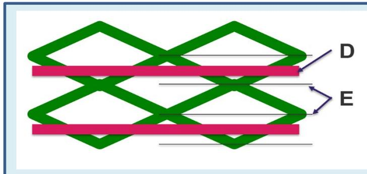
**D:** Single-ended traces should be centered between cross hatch intersections.
