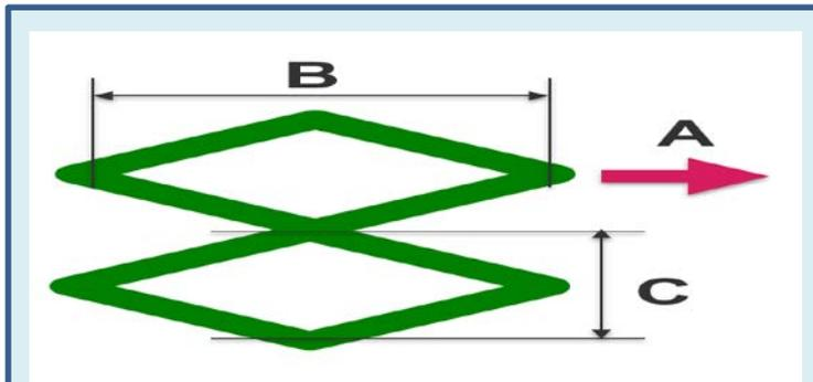
**A:** Diamond shaped cross-hatch patterns work better than square cross-hatch patterns. The longest length of the pattern should be parallel the signal traces.
