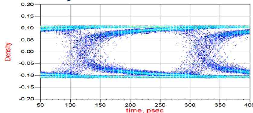
From the eye diagrams, we can see that the properly aligned traces have much better signal quality.
