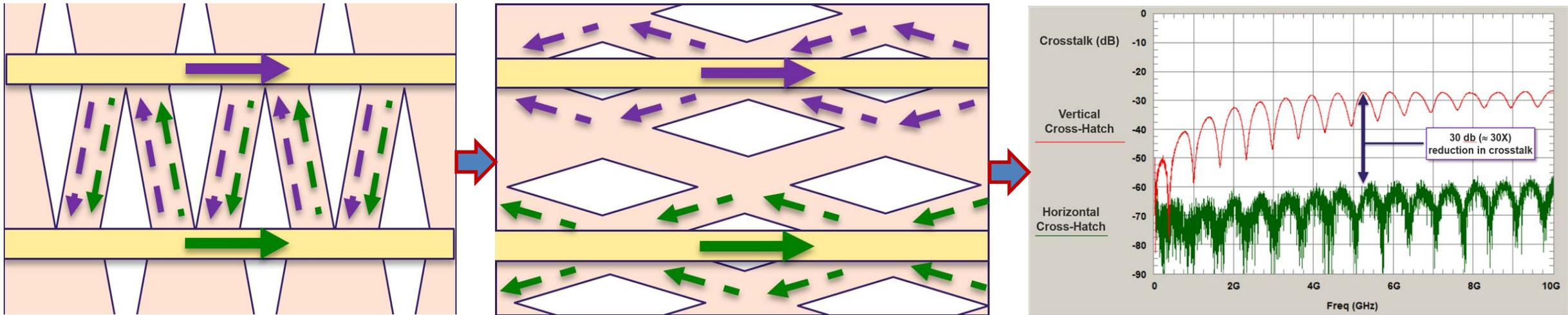
The above images show an example of how changing the orientation of the cross-hatched pattern from Vertical Cross-Hatch to Horizontal Cross-Hatch can significantly reduce crosstalk (In this case there was a 30 dB reduction in crosstalk)
