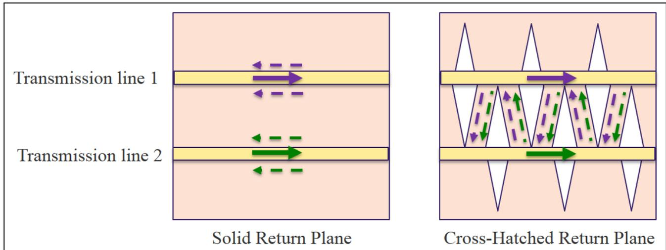
Figure 2: Comparison of Solid Return Plane and Cross-Hatched Return Plane Current Flow
