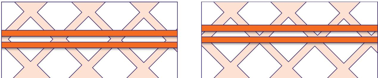
Figure 4: Examples of Ideal Registration (Left) and Poor Registration (Right)
