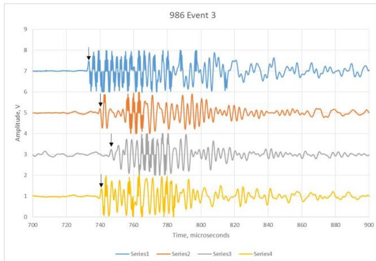
**Figure2 - A set of waveforms for an event. Black arrow marks the arrival time at each transducer.**
