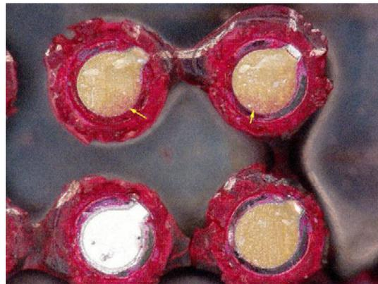
**Figure 12 - Dye stain (left) on the fourth PCA from the high rate test showing pad cratering**
