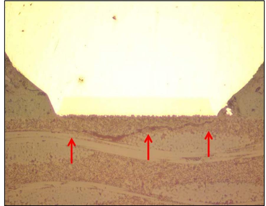
Cross-section showing pad crater under a BGA pad
