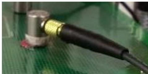
**Figure 3 - Acoustic transducer mounted to a PCB with accelerometer wax**
