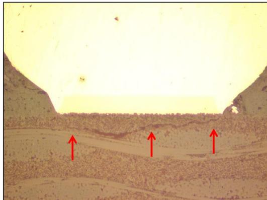
**Figure1 - Pad crater under a BGA pad, as observed in a cross-section**
