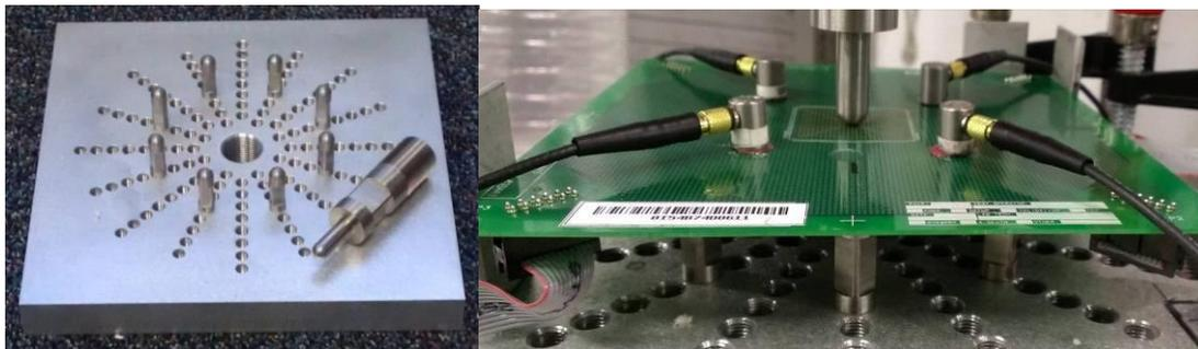
**Figure 8 - Spherical bend test fixture and setup**
