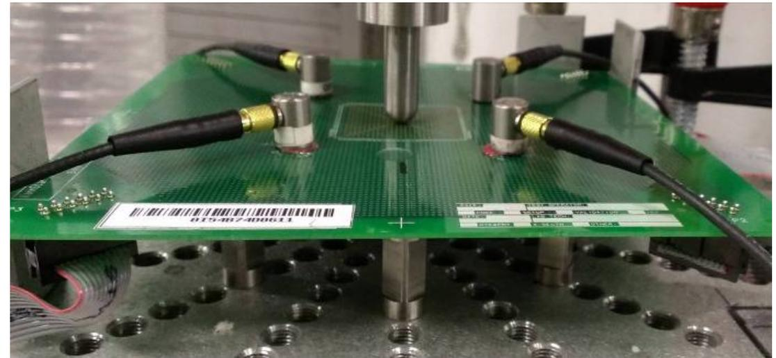
Wide-band transducers, sensitive to at least 100 kHz and up to 700 kHz, flat frequency response
