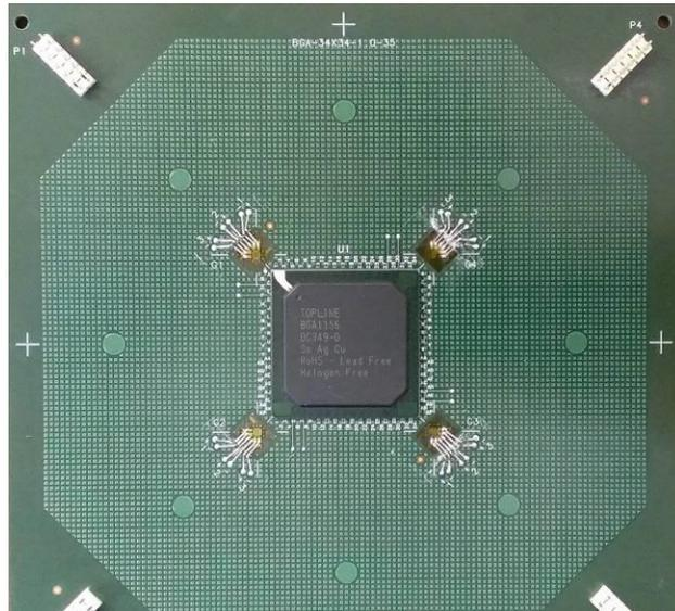
**Figure 7 - Test specimen for spherical bend**
