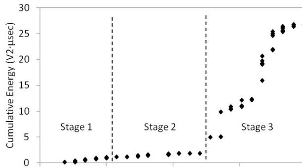
**Figure 9 - Typical cumulative energy plot showing three stages of acoustic activity**
