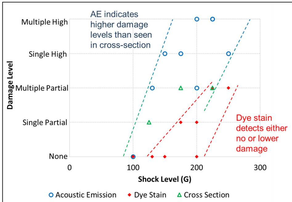
**Figure 15 – A Comparison of AE Damage Detection to Failure Analysis Results**
