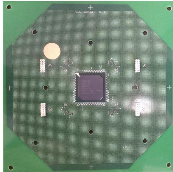
**Figure 13 - Shock Test Vehicle**
