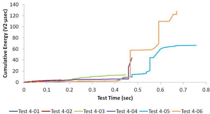
**Figure 11 – Cumulative Magnitude versus Time for High Rate Tests**
