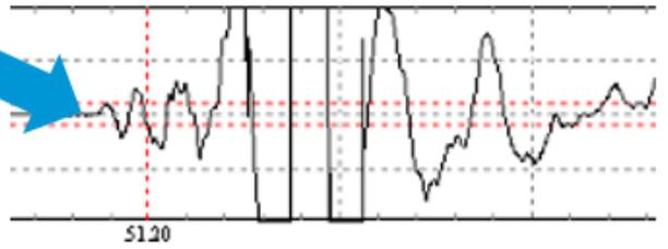
The method can detect pad crater initiation without destroying the sample. Testing can continue as damage and detection progress.
