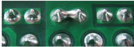
**Figure 1: Solder bridges are one of the most frequently experienced solder defects.**
