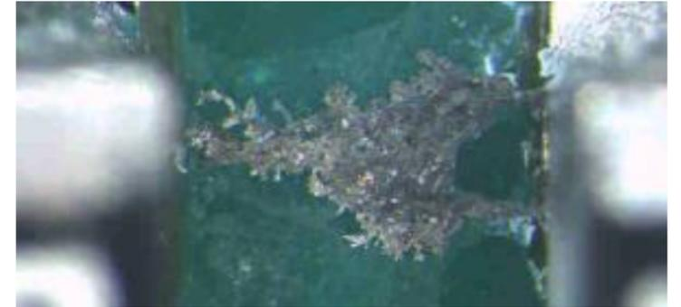
Insufficient solder hole fill
