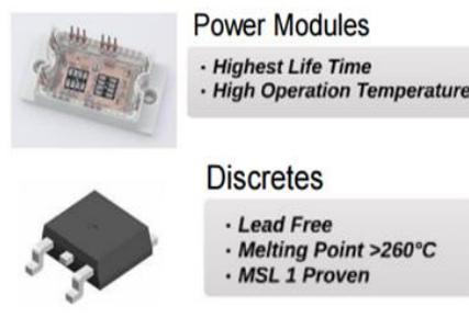
Figure 1. Typical applications for silver sintering
