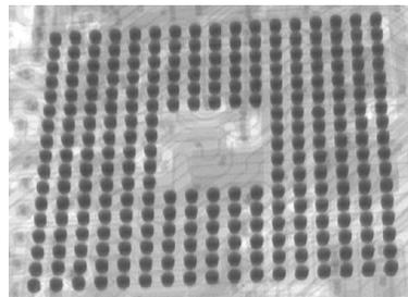
Figure 2 Example of a BGA area after SMT under X-ray inspection
