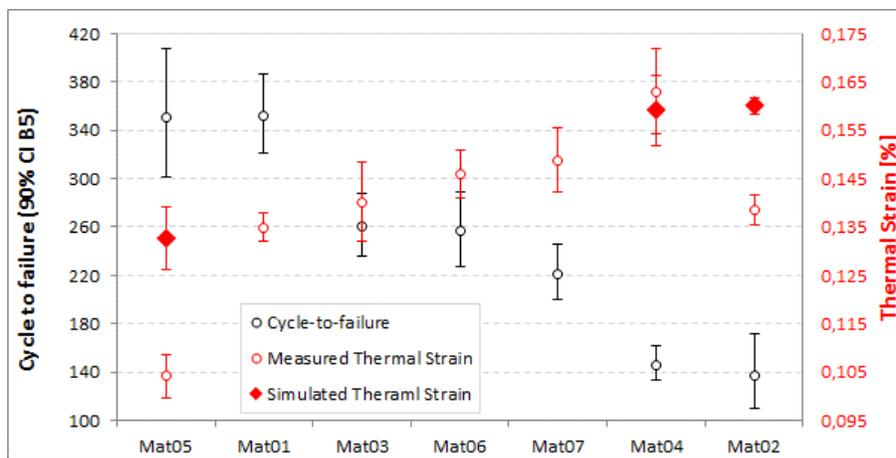
Figure 14 Relationship between cycle to failure and the thermal strain at 125°C
