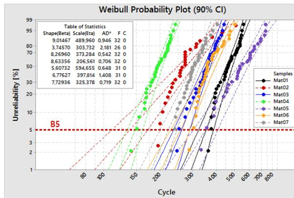
Figure 5 Weibull probability plot with 90% confidence interval
