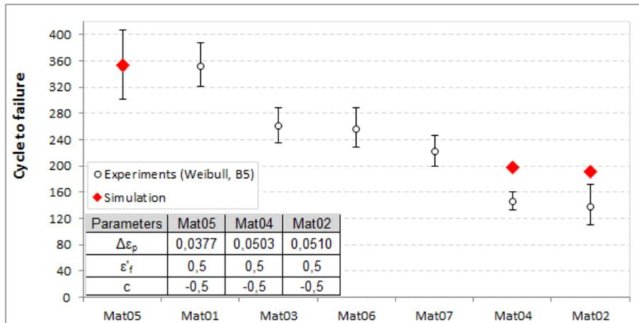
Figure 13 Comparison of the cycle to failure between the experiments and the simulation
