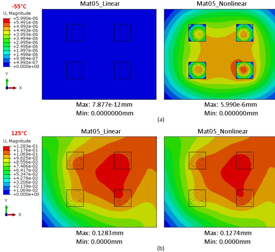
Figure 10 Top view of deformation comparisons between the linear and nonlinear procedures for Mat05 at the end (a) and at the middle (b) of one TST cycle
