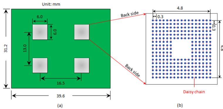
Figure 1 Setup and dimension of PCBA (a) and bottom view of the chip (b)
