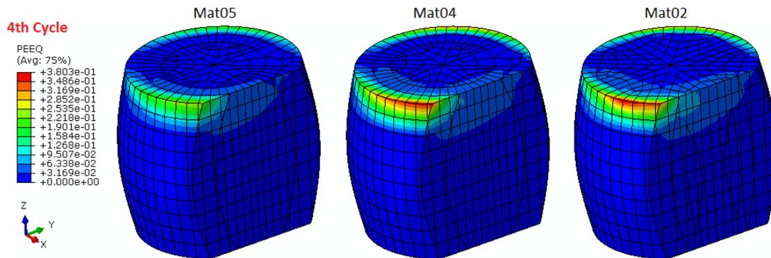
Figure 12 Accumulated plastic strain (PEEQ) of the solder joints at 125°C of the 4<sup>th</sup> cycle in the lower-right corner of the BGA area as shown in Figure 11 (chips are on the top side)
