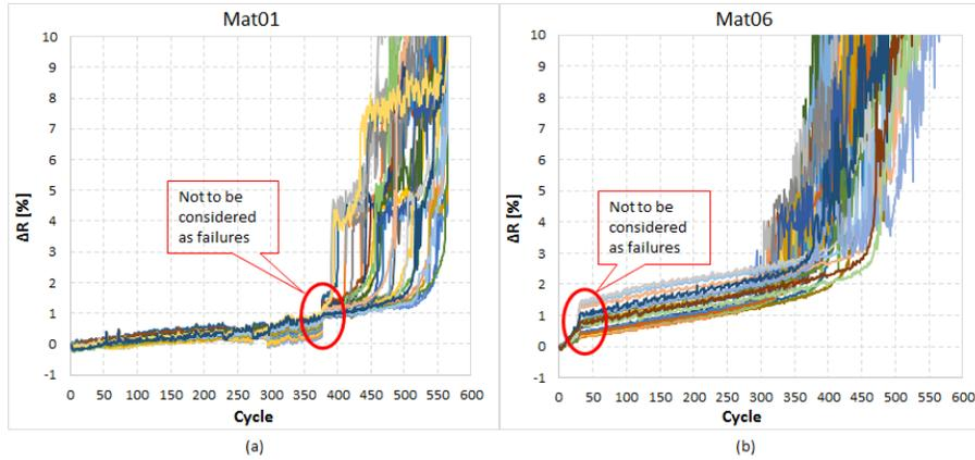
**Figure 3 Resistance change of Mat01 (a) and Mat06 (b) directly calculated based on the online resistance measurement data**
