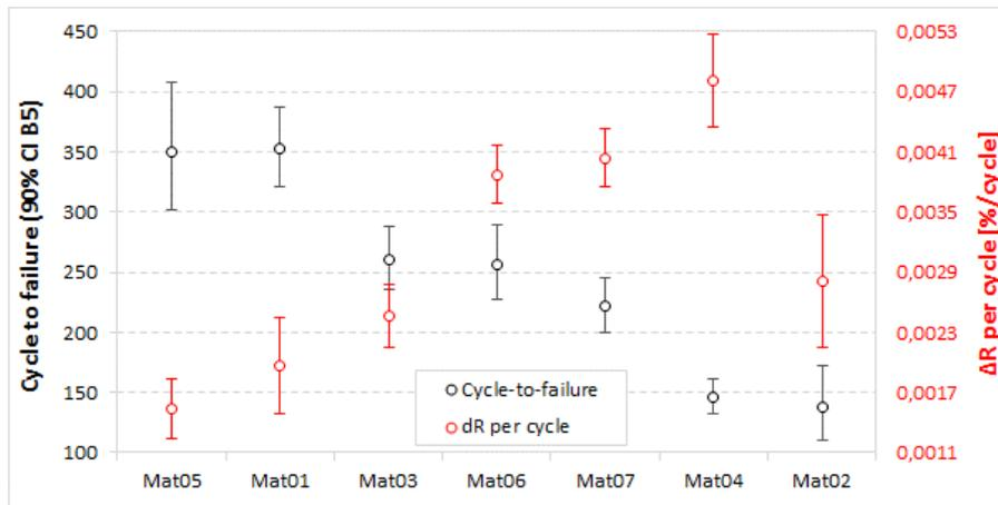
Figure 7 Relationship between cycle to failure and the resistance change rate per cycle
