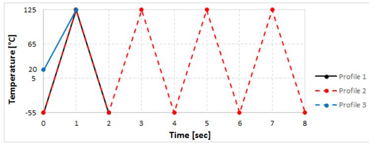
**Figure 9 Temperature profiles used in the simulation**
