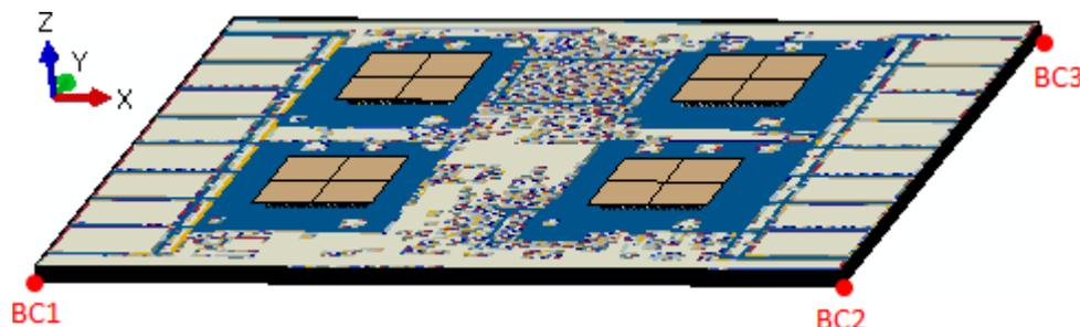
Figure 8 PCBA model in the FEA software with three boundary conditions
