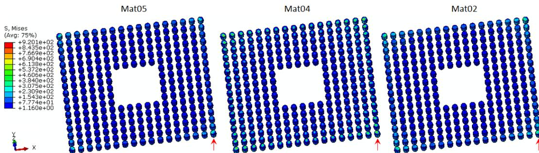
Figure 11 Von Mises stresses of the solder joints on the lower-right area of the PCBA for Mat05, Mat04 and Mat02 (chips are on the top side)
