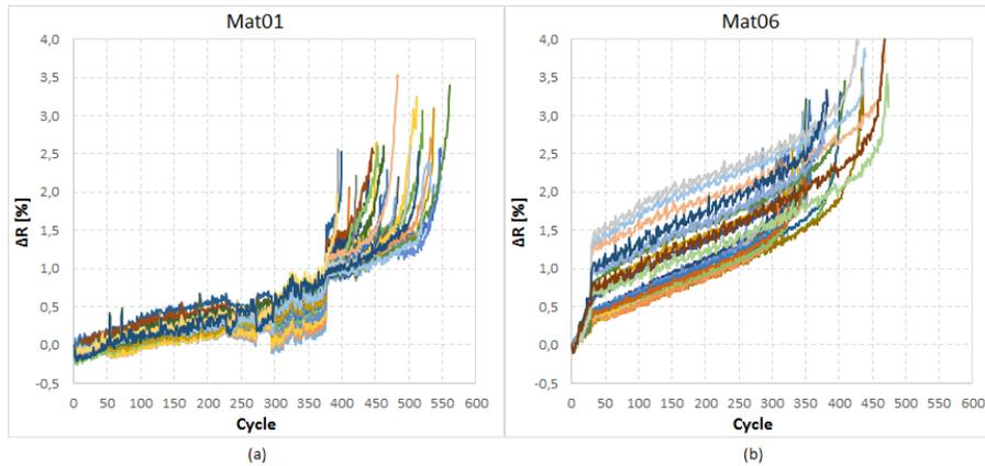
**Figure 4 Resistance change of Mat01 (a) and Mat06 (b) by removing the data after failure so that the cycle to failure (end of each curve) can be visualized**
