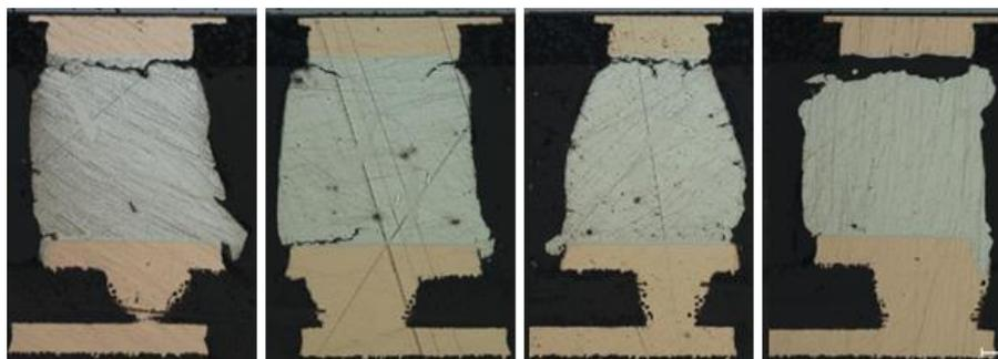
Figure 6 Typical cross-section images for the solder joint failures (chips are on the top side)
