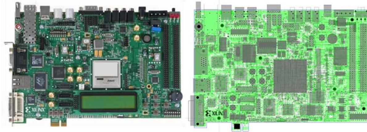
Figure 5. a) Picture of production FPGA board b) Layout of board assembly generated by automated design analysis
