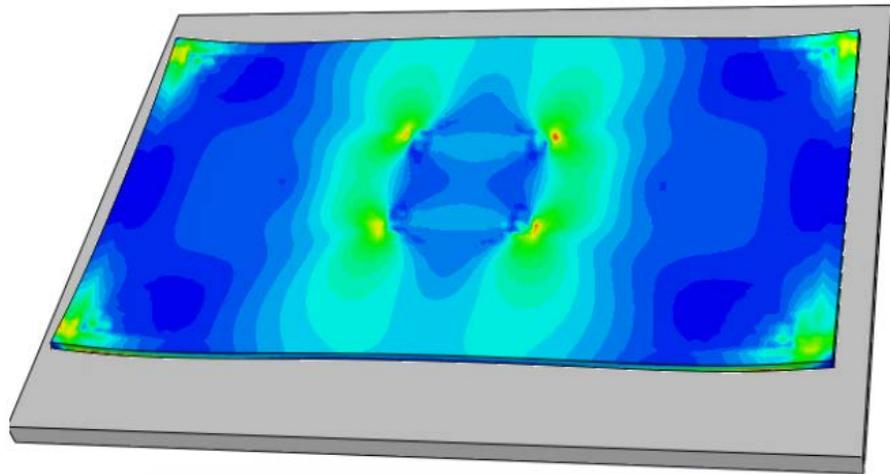
Strain: Board Top Side at 100°C
