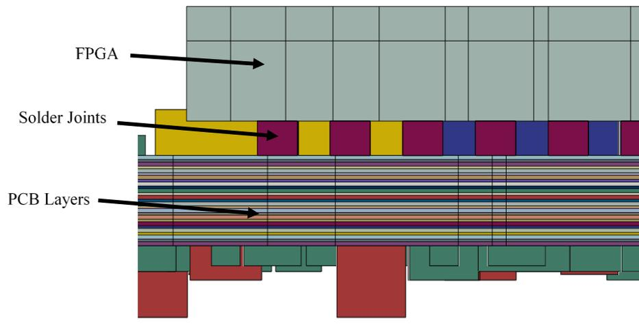
**Figure 7. Close up of FPGA package showing PCB layers and solder joints.**
