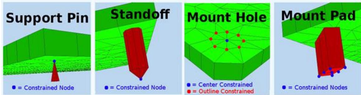
**Figure 8. Predefined Boundary Conditions for mounting points.**
