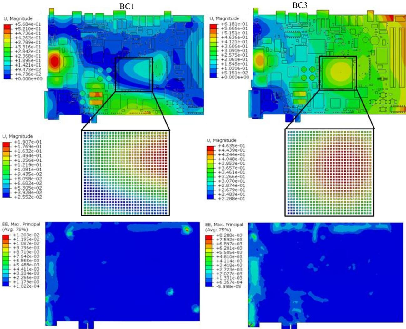
**Figure 11. Equivalent board displacement, FPGA displacement and maximum principal board strain at 125°C for boundary conditions BC1 to BC3.**
