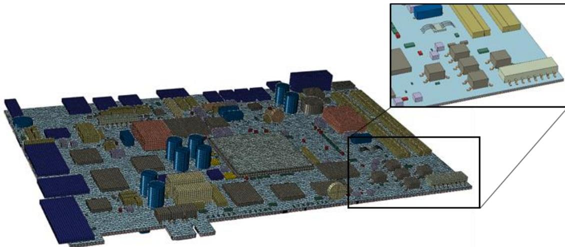
Figure 6. Fully meshed 3D model of production FPGA assembly with 2mm PCB mesh.
