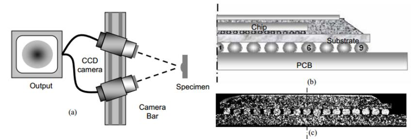
Schematic of 3-D Digital Image Correlation with cross section of test sample
