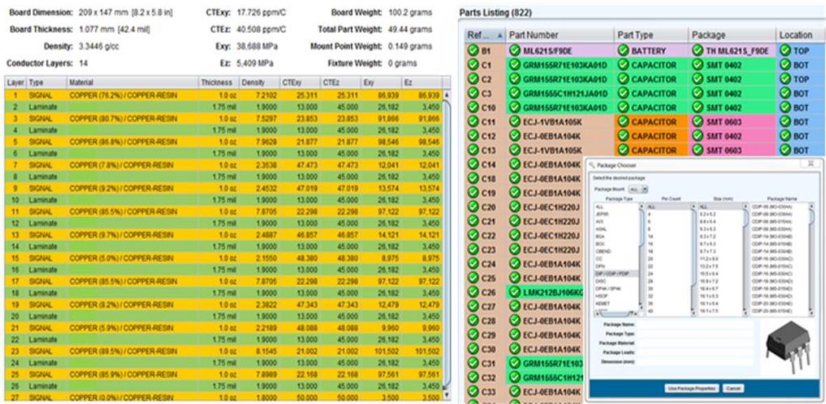
Figure 4. PCB layers and built in package manager
