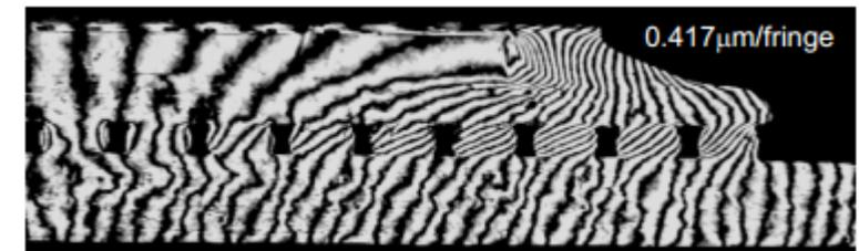
Contour plot of u deformation field of the die-shadow solder joint obtained from Moire Interferometry
