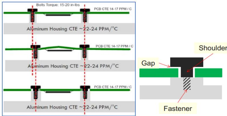
**Figure 1. Effect of CTE mismatch and board constraint on leaded surface mount package**
