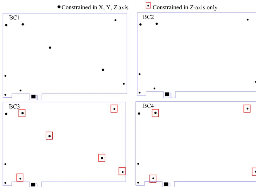
**Figure 9. Boundary Conditions used for production FPGA PCB**
