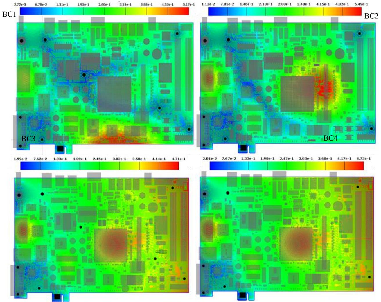
**Figure 10. Equivalent board displacement at 125°C boundary conditions BC1 to BC4 superimposed on first copper layer.**
