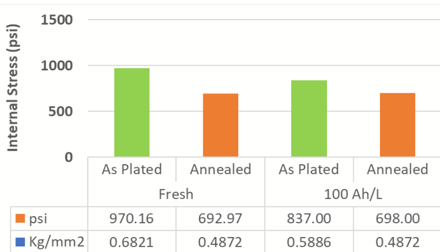
Figure 9. Internal stress of the Cu deposit plated using Process I, both as plated and annealed data for fresh and aged baths.
