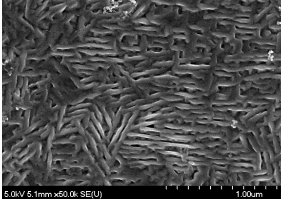
Figure 2a: Bright Polycrystalline Tin on Nanocrystalline Copper – Control Sample (Index 2)
