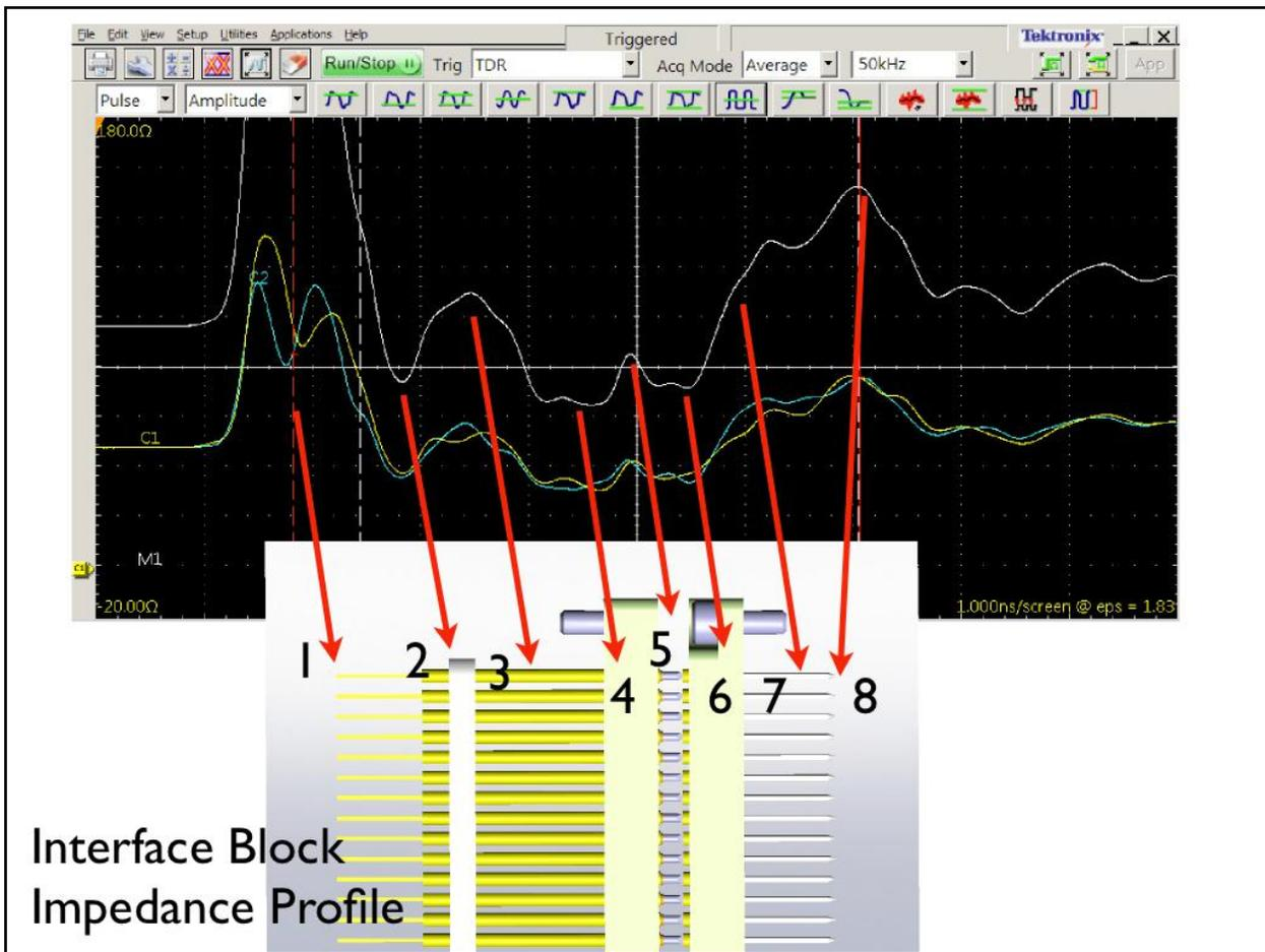
Figure 13 - Impedance profile for a 170 pin interface block
