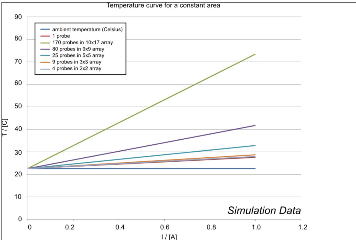
Figure 7 - Temperature (1 probe) for a constant area
