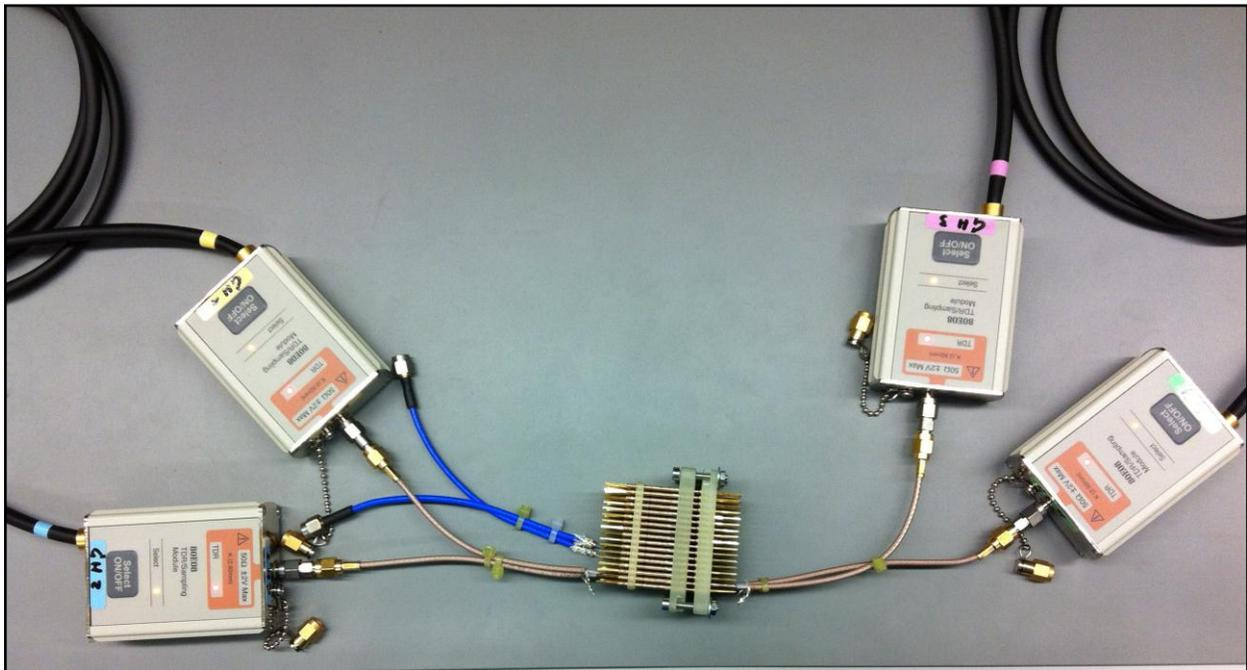
**Figure 11 - Measurement setup with 4 x 30 GHz detector heads**
