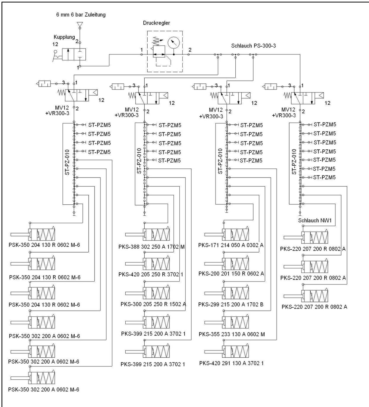
Figure 19 - Schematic for contacting 19 pneumatic probes in 4 groups
