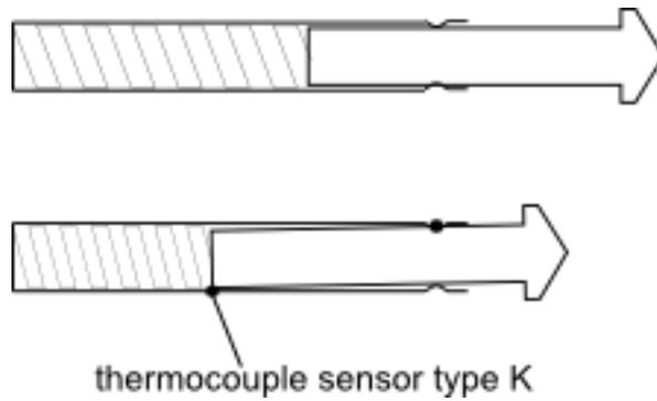
**Figure 5 - Measurement point for the thermocoupler**
