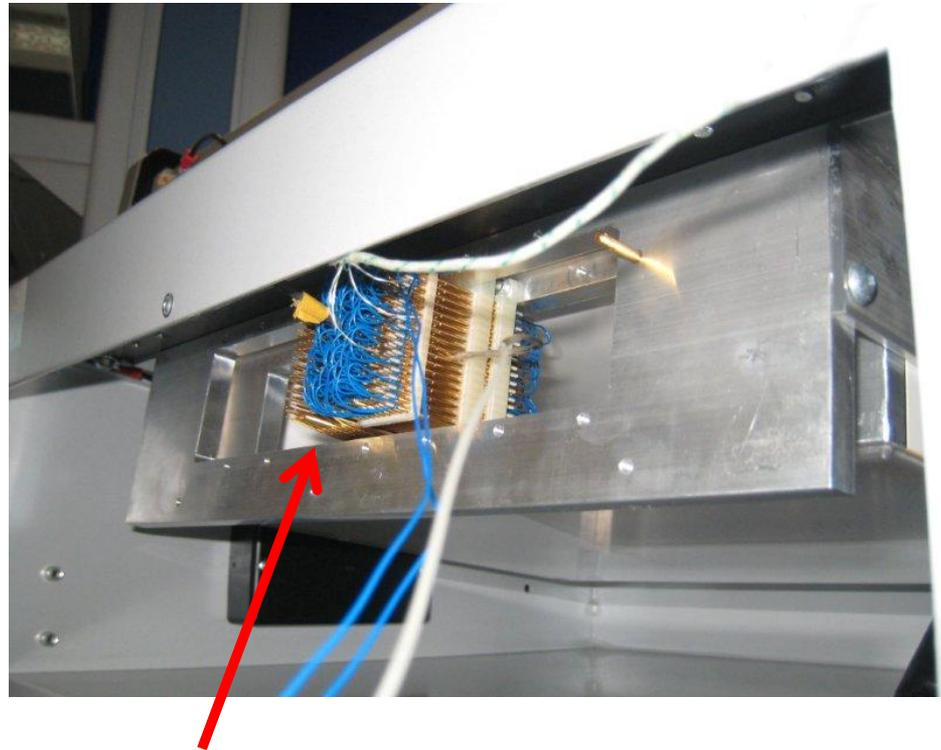
170 pin interface block with thermocouple element in a *real life* test Fixture (no test lab mockup)
