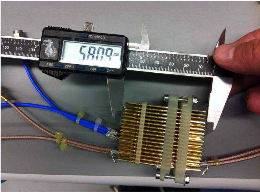
The dielectric value ( $\epsilon_r$ ) can be derived from a measurement of the mechanical length and comparison with the electrical length (using a TDR scope or VNA with IFFT mode)
