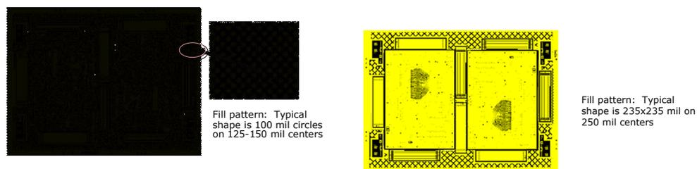
**Figure 12 - Representative Fill Patterns for Signal Layers and Plane Layers**
