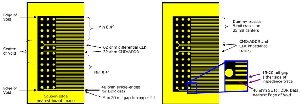
**Figure 10 - Coupon Design for Partial POOL DDR**
