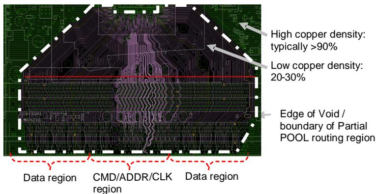
**Figure 4 - Copper Density Change at Edge of Void**
