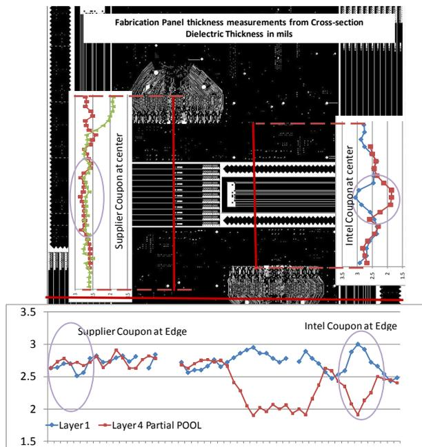
**Figure 8 - Supplier A Impedance Coupon Test Board Results**
