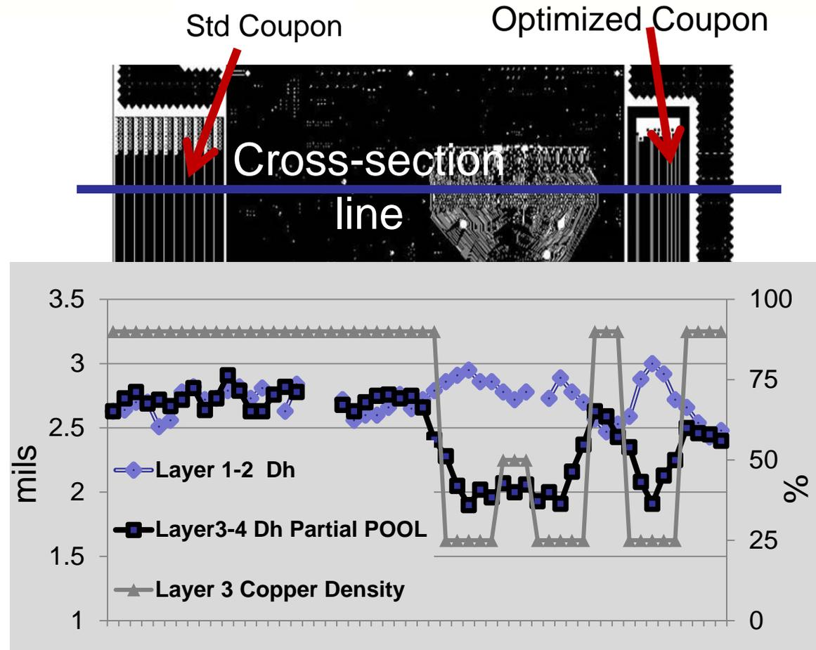
**Dielectric Height vs Copper Density across fabrication panel**
