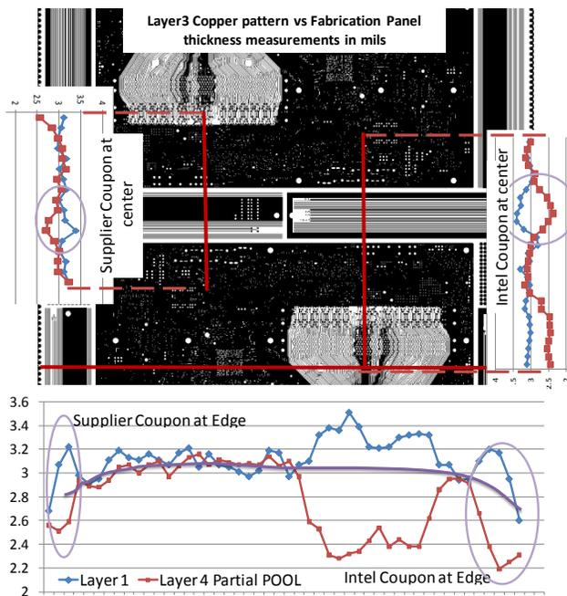
**Figure 9 - Supplier B Impedance Coupon Test Board Results**
