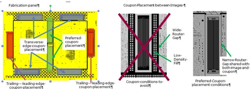
**Figure 11 - BKM Placement of Impedance coupons**
