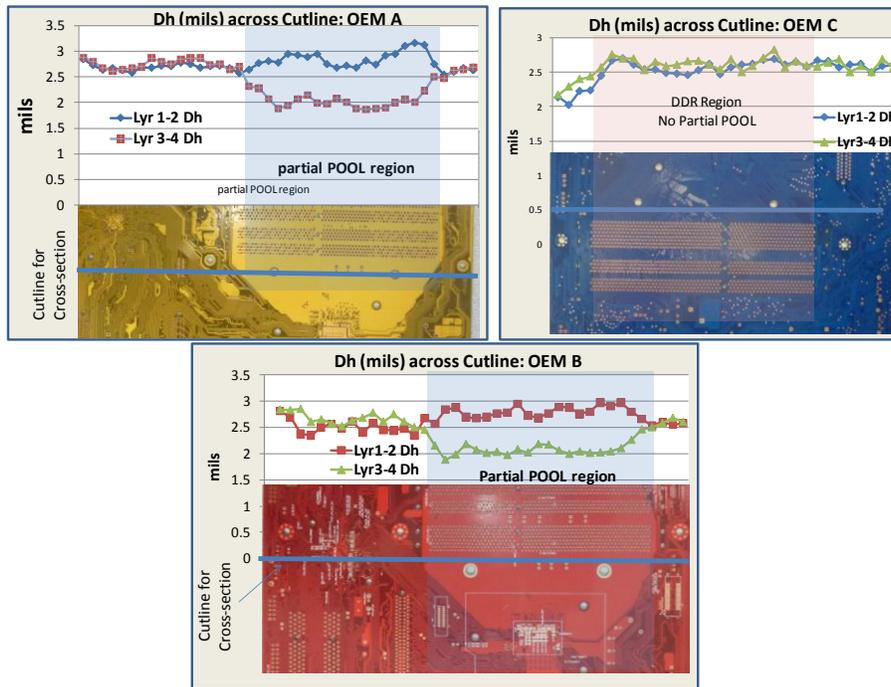
**Figure 6 - Dielectric Height Profile across the Partial POOL DDR Layer**
