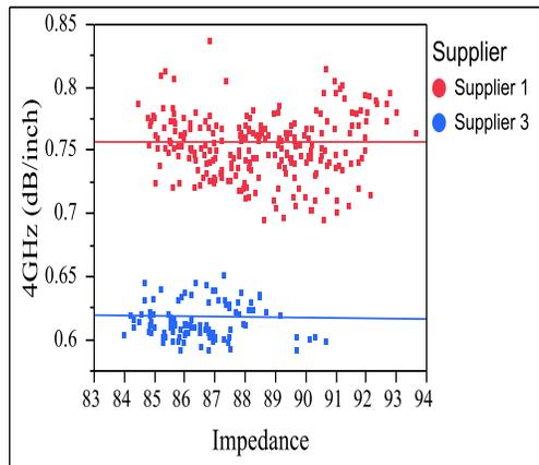
**Figure 16.** Impedance and insertion loss relationship of Product 2 layer 3 at 4GHz.
