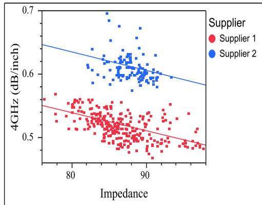
**Figure 15.** Impedance and insertion loss relationship of Product 1 layer 1 at 4GHz.
