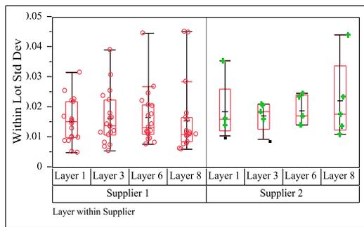
Figure 10. Coupon to coupon loss variation at 4 GHz on Product 1.
