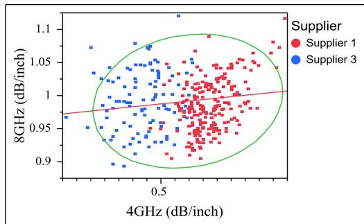
**Figure 13.** PCB insertion loss relationship between 4 GHz and 8 GHz on layer 1 of Product 2.
