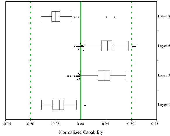
**Figure 4.** PCB construction capability by Supplier 1 on Product 1.
