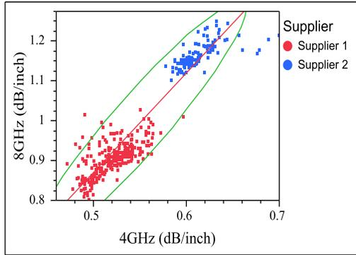
**Figure 11.** PCB insertion loss relationship between 4 GHz and 8 GHz on layer 1 of Product 1.
