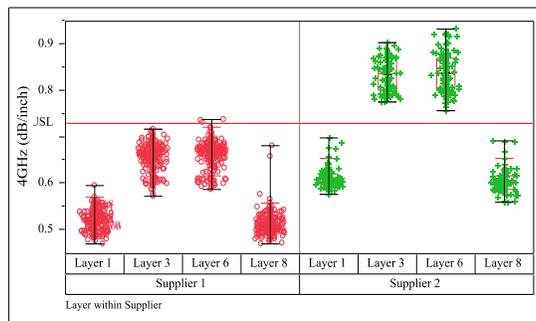
**Figure 7.** PCB insertion loss for Product 1 at 4 GHz.
