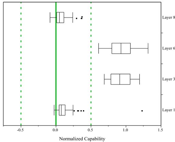
**Figure 5.** PCB construction capability by Supplier 2 on Product 1.
