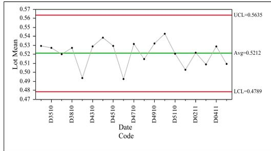
Figure 8. Insertion loss lot mean distribution of Product 1 on layer 1 at 4GHz.
