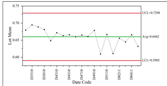
Figure 9. Insertion loss lot mean distribution for Product 1 on layer 3 at 4GHz.
