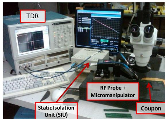
**Figure 3.** SET2DIL measurement setup (courtesy of Introbotix).
