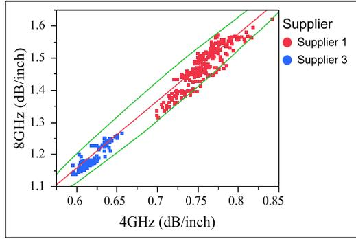
**Figure 14.** PCB insertion loss relationship between 4 GHz and 8 GHz on layer 3 of Product 2.
