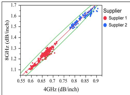
**Figure 12.** PCB insertion loss relationship between 4 GHz and 8 GHz on layer 3 of Product 1.
