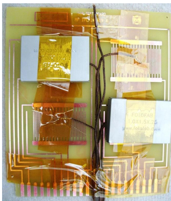
Figure 3 - IPC-B-24 SIR Test Coupon showing location of thermocouples and RF shields
