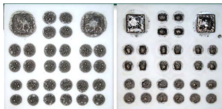
Figure 1 - Wetting of Bi/11Ag (left) and Bi/10Ag/4Sn (right) on Ag/Pd thick film pad Al_2O_3 substrate
