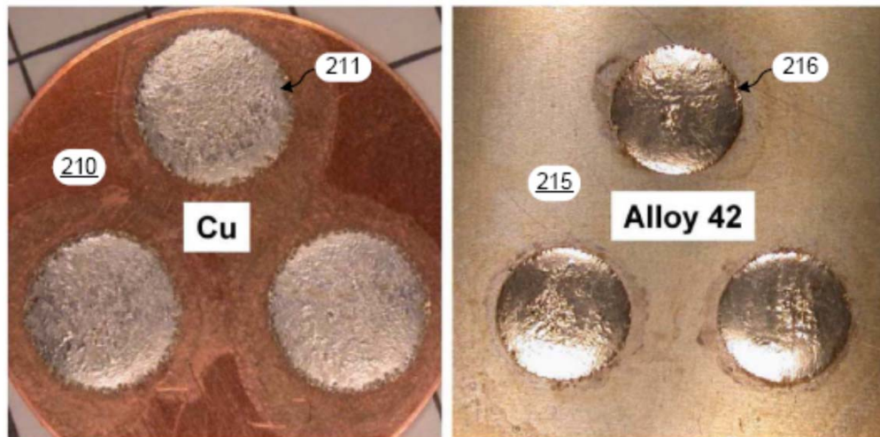
Left: mixed solder paste on Cu Right: mixed solder paste on Alloy 42
