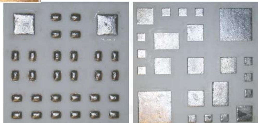
Left: mixed solder paste /Ag-Pd-Alumina Right: mixed solder paste /Ag-Pt-Alumina
