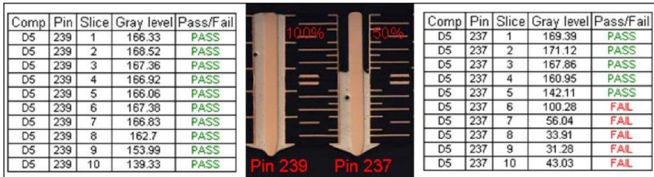
Figure 6. X-ray program validation for component D5
