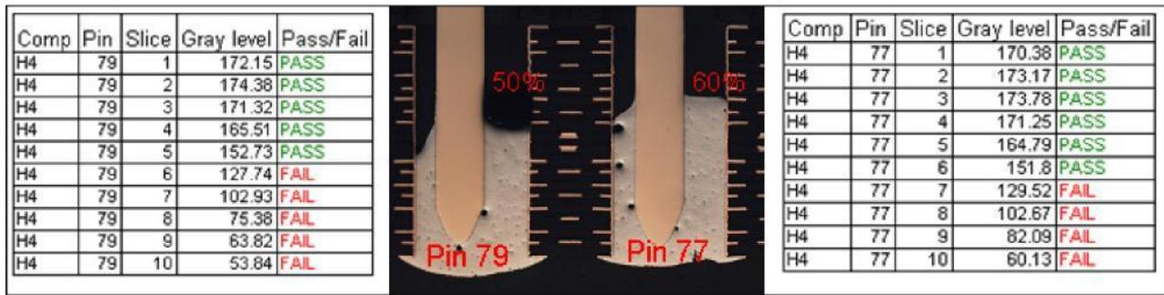
Figure 7. X-ray program validation for component H4
