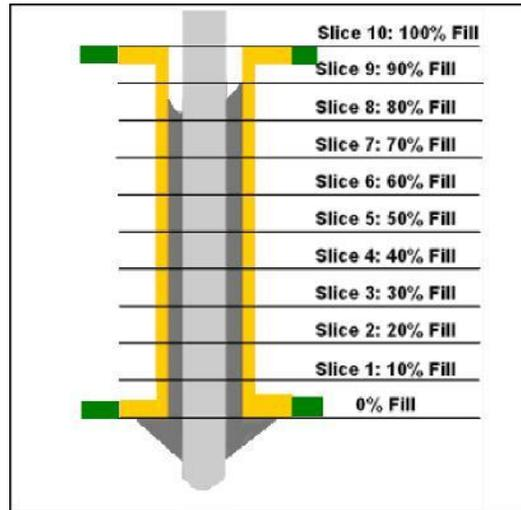
Figure 4. X-ray inspection program: 10 slices
