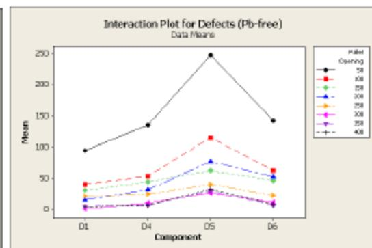
Figure 11. Interaction between pallet opening and DIMM component
