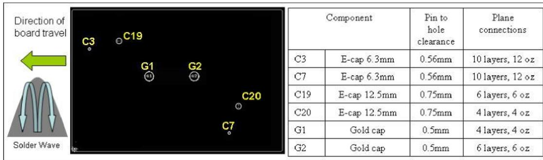
**Figure 20.** Capacitors layout and direction of board travel
