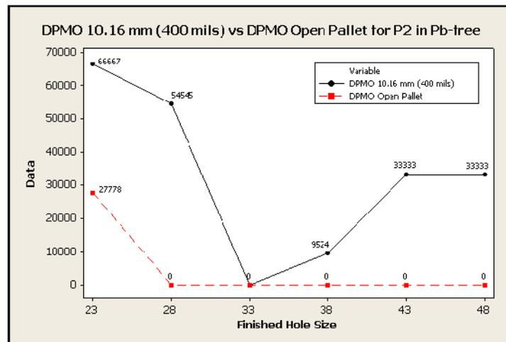
Figure 27. DPMO for P2 with an open pallet
