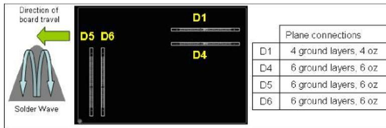
**Figure 12.** DIMM layout and direction of board travel
