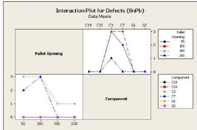
**Figure 23.** Interaction between pallet opening and PTH capacitor.
