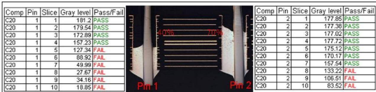
Figure 5. X-ray program validation for component C20
