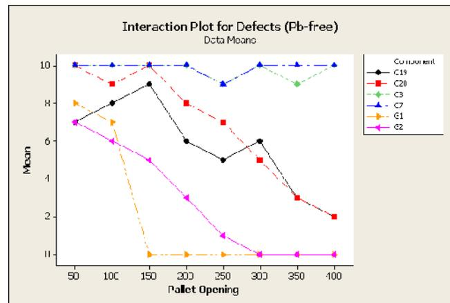
Figure 19. Capacitors, interaction between pallet opening component
