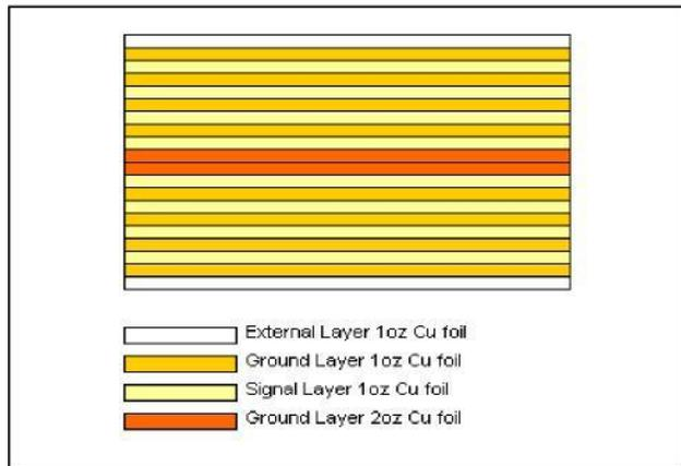
Figure 2 . Board stack-up
