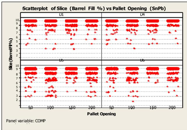
Figure 16. DIMM connector barrel fill results for SnPb
