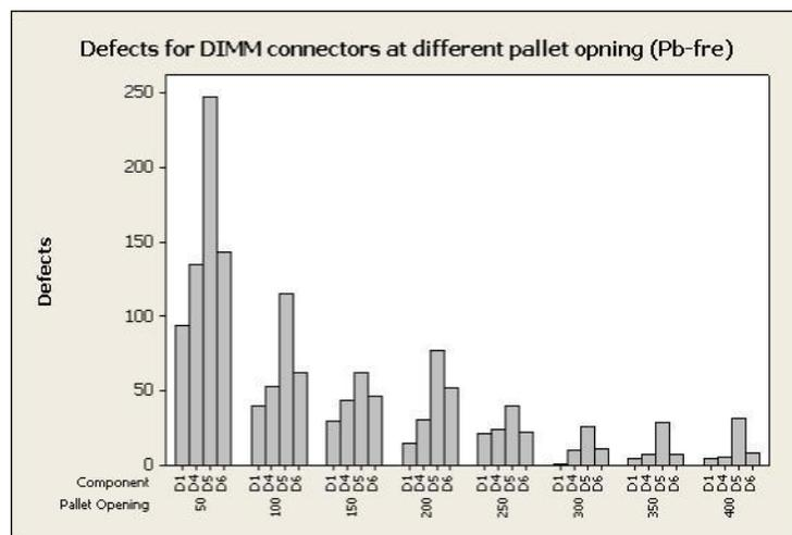
**Figure 13.** DIMM defects at different pallet opening (Pb-free)
