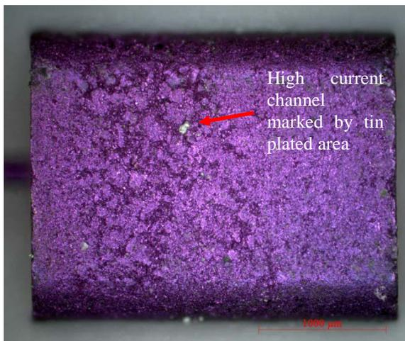
**Figure 4: Decapsulated virgin capacitor from vendor A after tin plating under reverse voltage.**
