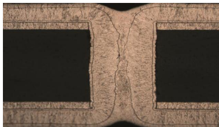
Figure 15 – Filing 200 \mu\text{m} through holes in 400 \mu\text{m} thick substrate
