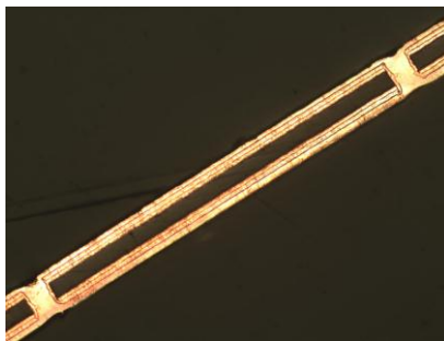
Figure 14 – Through Hole Fill, 50 \mu\text{m} diameter in 50 \mu\text{m} thick flexible substrate
