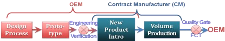
Figure 1: A typical OEM-to-CM product flow
