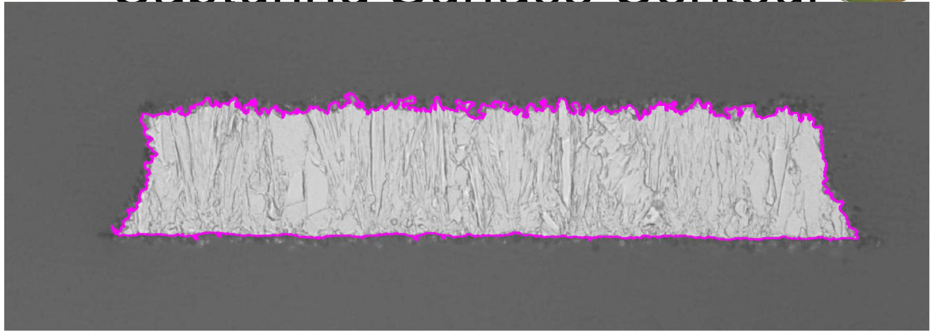
Program performs filtering to clean up optical artifacts and find boundary between Cu and surrounding resin, then creates a pixel map corresponding to perimeter.
