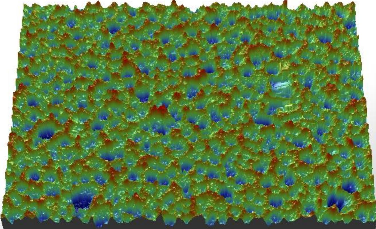
A 3-D contour map of raw 1-oz Standard E.D. foil from laser profilometry of the treatment side:
