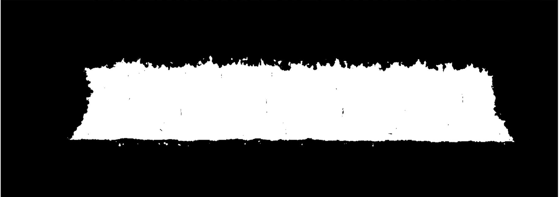
The image is forced to binary black/white so that the tool does not pick up non-homogeneous elements of the dielectric (glass bundles, filler particles).
