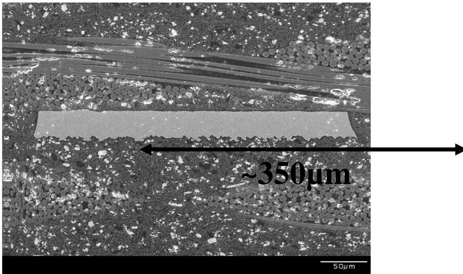
Figure 6: Sample SEM image with  $R_z \approx 9 \mu\text{m}$
