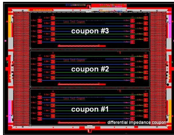
Figure 3 Location of Differential Impedance Coupon
