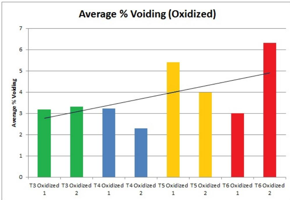
It was our theory that the more oxidation that was present within the powder, and the finer the mesh size, the more voiding that would be present. This would be due to increased outgassing because of the additional oxides being removed by the flux during reflow. Though the trend lines for the graphs above agreed with this speculation, the data is somewhat unclear. The average voiding percentage did not exceed 7% even in the worst-case-scenario solder paste (oxidized Type 6).
