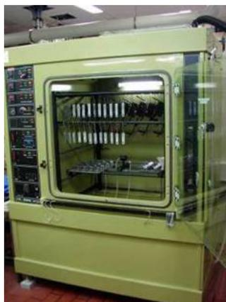
**Fig. 7** Salt-Spray Test Chamber
