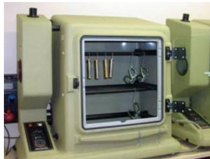
**Fig. 6** Kesternich-test chamber
