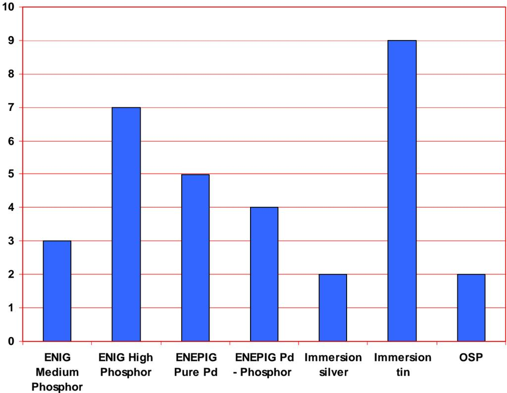
***Immersion Tin, ENIG High Phosphor, and ENEPIG shows the best corrosion resistance for the final product.***
