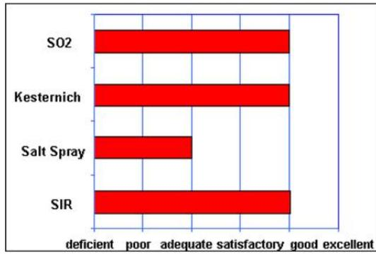
**Fig. 18** Corrosion test results for ENEPIG (Pure Pd)
