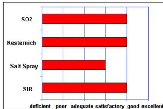
Fig. 17 Corrosion test results for ENIG (High P)
