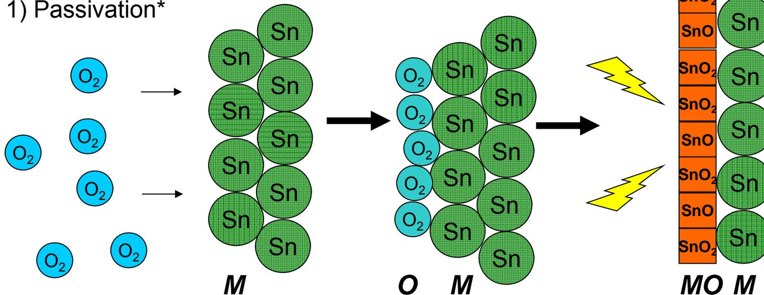
The thin free of pores oxide layer ( $SnO/SnO_2$ ) adds Immersion tin a high corrosion resistance.
