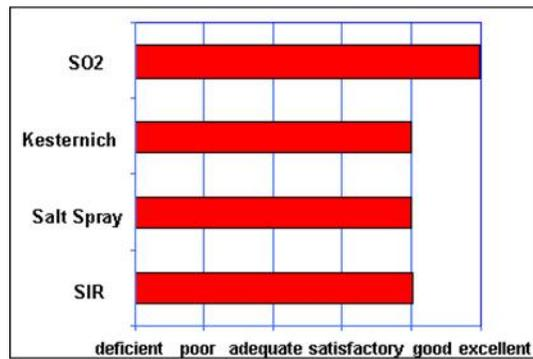
**Fig. 21** Corrosion test results for immersion tin
