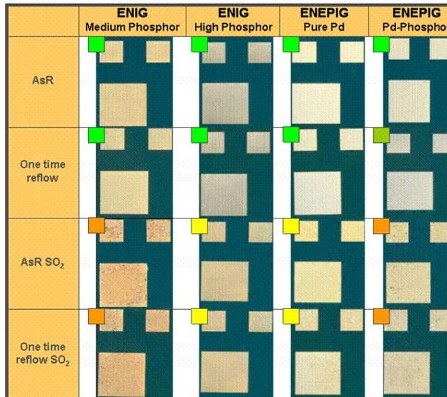
**Fig. 8** SO<sub>2</sub> Gas Test results for ENIG and ENEPIG
