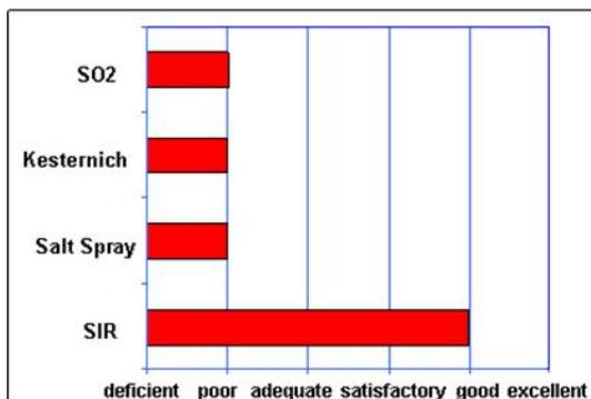
**Fig. 20:** Corrosion test results for immersion silver
