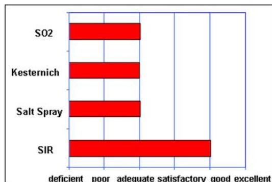
**Fig. 23** Corrosion test results for OSP
