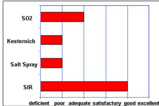
Fig. 16 Corrosion test results for ENIG (Medium P)
