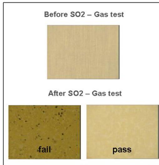
**Fig. 5** Example of pass-fail criteria for the SO<sub>2</sub> Gas Test
