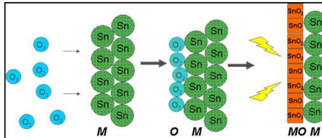
**Fig. 22** Passivation of the immersion tin surface [1]
