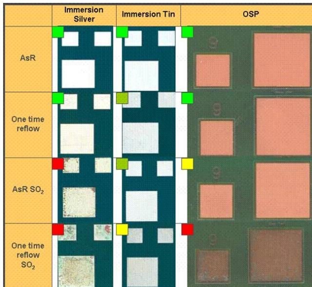
**Fig. 9:** SO<sub>2</sub> Gas Test results for immersion silver, immersion tin and OSP
