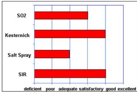
**Fig. 19** Corrosion test results for ENEPIG (Pd-P)
