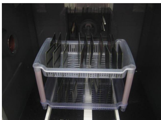
Figure 8. PCB placement for MFG Test
