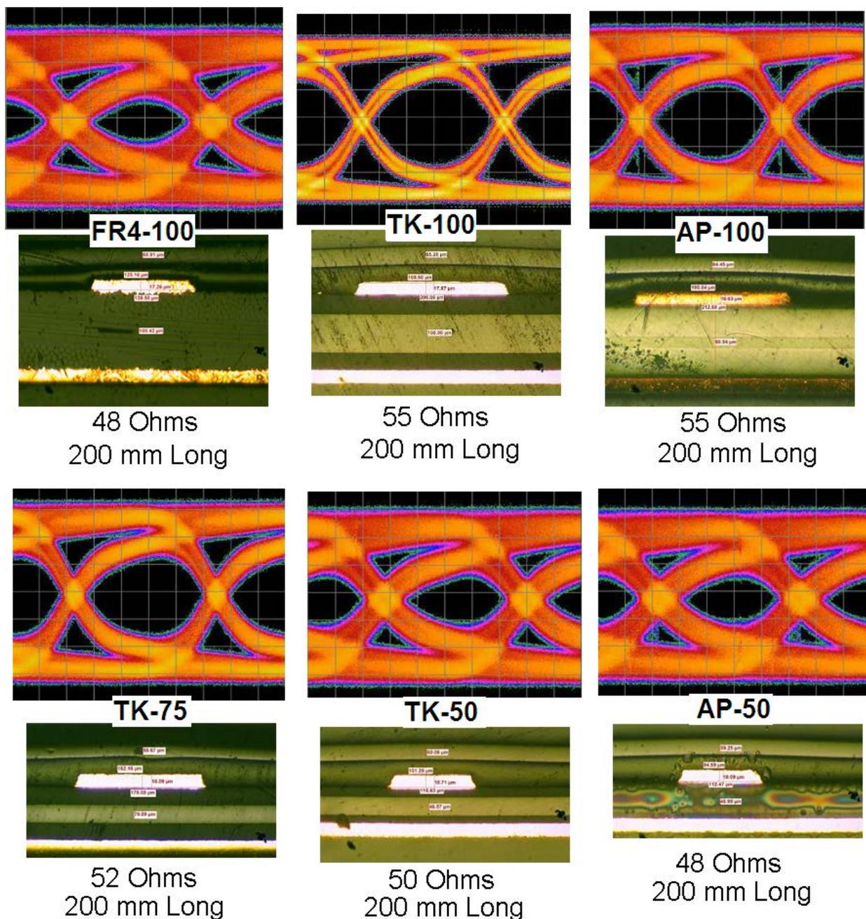
Figure 14 – Effect of ENIG on Loss in Microstrip Structures
