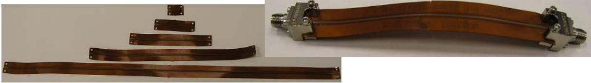
Figure 6 – One Set of Microstrip Lines (5 out of 25), One Enlarged Shown with Connectors
