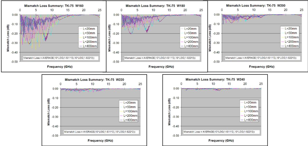
Figure 8 – Raw Mismatch Loss Measurements for the 25 TK-75 Lines
