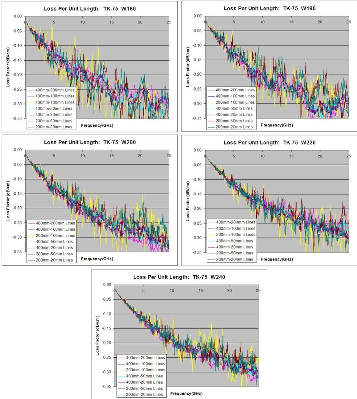
Figure 9 – Loss per Unit Length for the 25 TK-75 Lines
