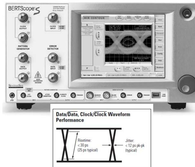
Figure 15 – Test Equipment for Eye Pattern Testing
