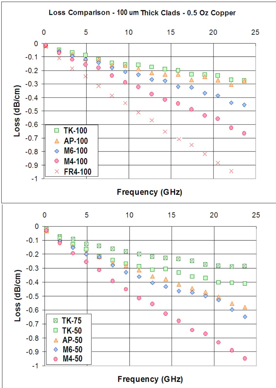
Figure 11 – Summary of Loss Measurements for 100 um Thick Microstrip Samples
