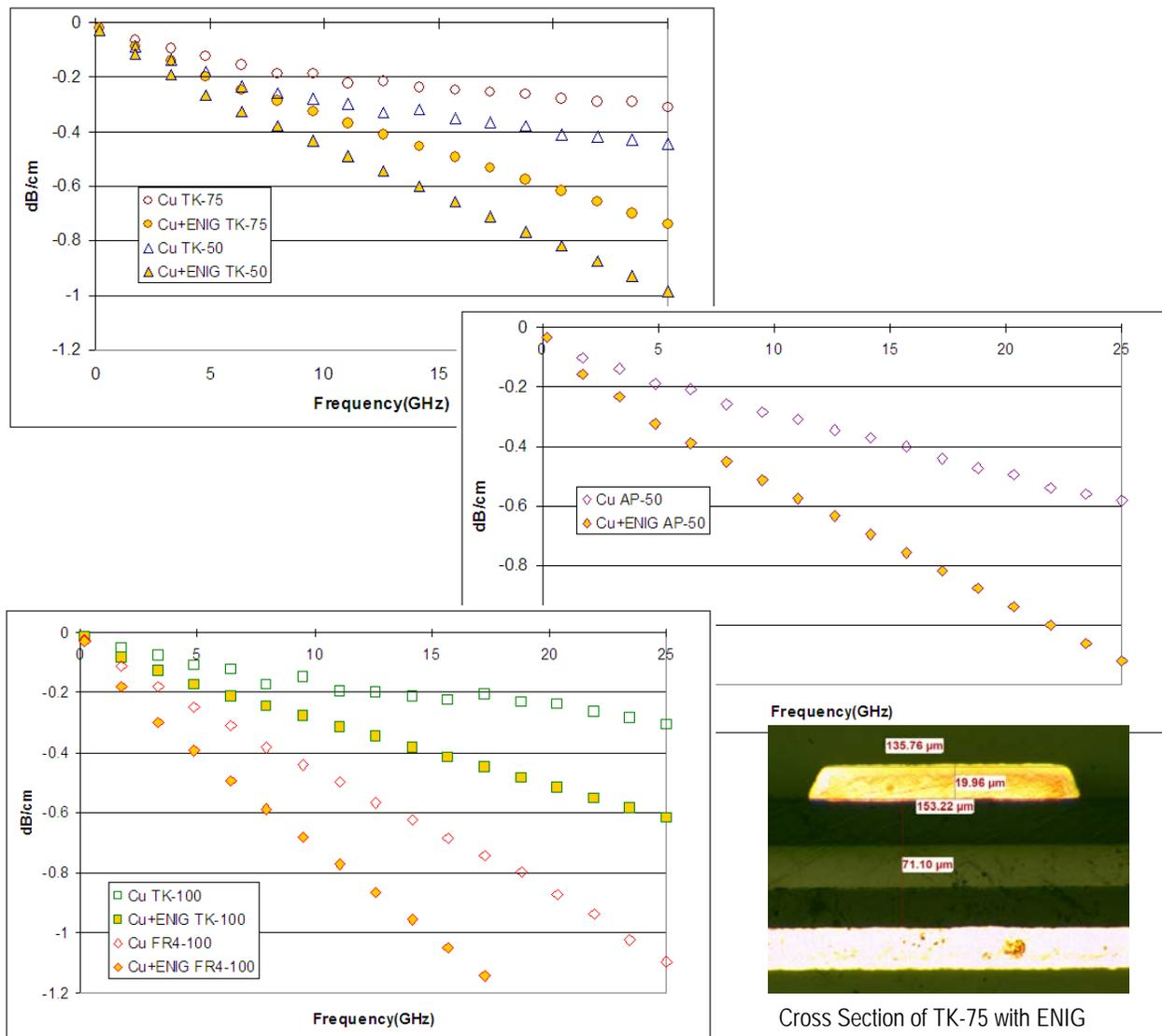
Figure 14 – Effect of ENIG on Loss in Microstrip Structures
