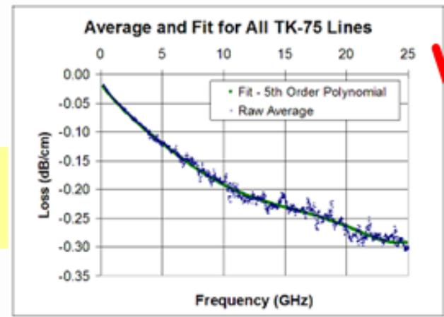
Average of 25 lines (five lengths x five widths) from the TK-75 clad
