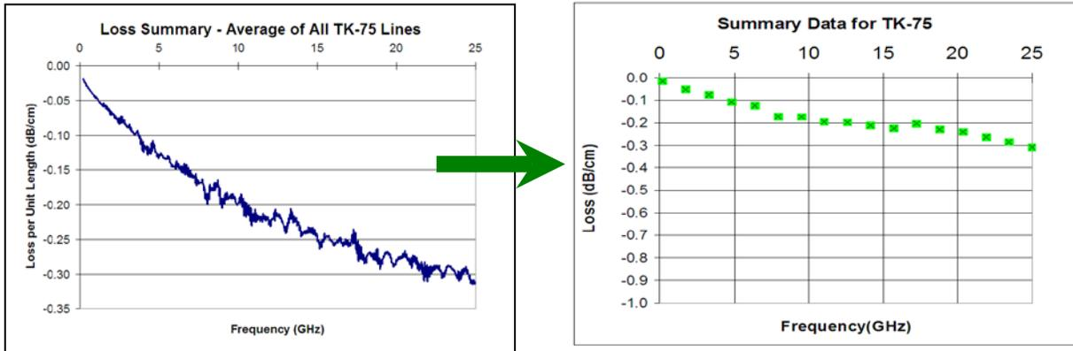
Figure 10 – Development of Summary Plots for the TK-75 Clad
