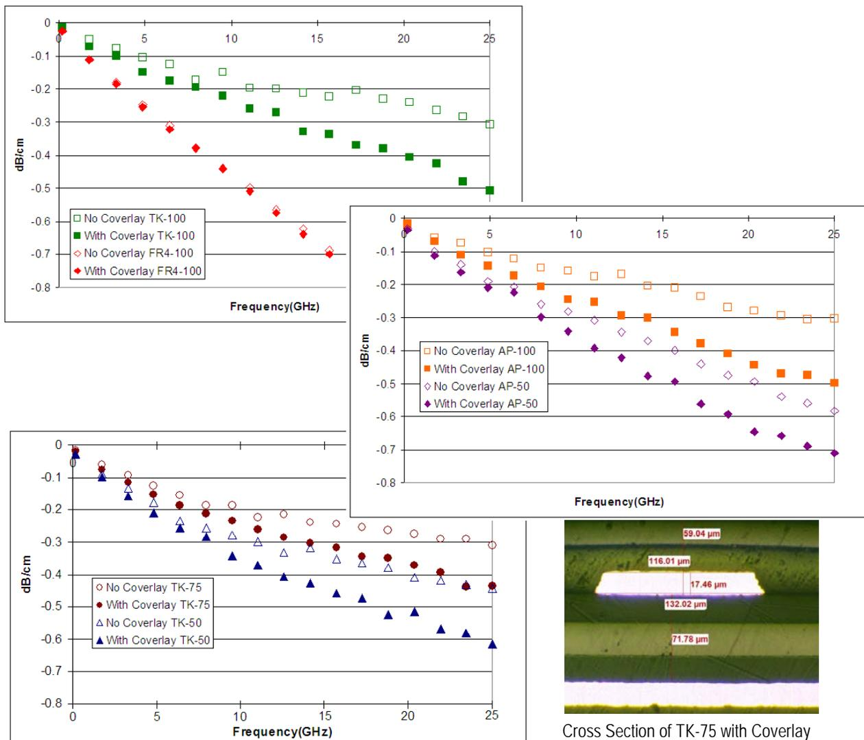
Figure 13 – Effect of Coverlay on Loss in Covered Microstrip Structures
