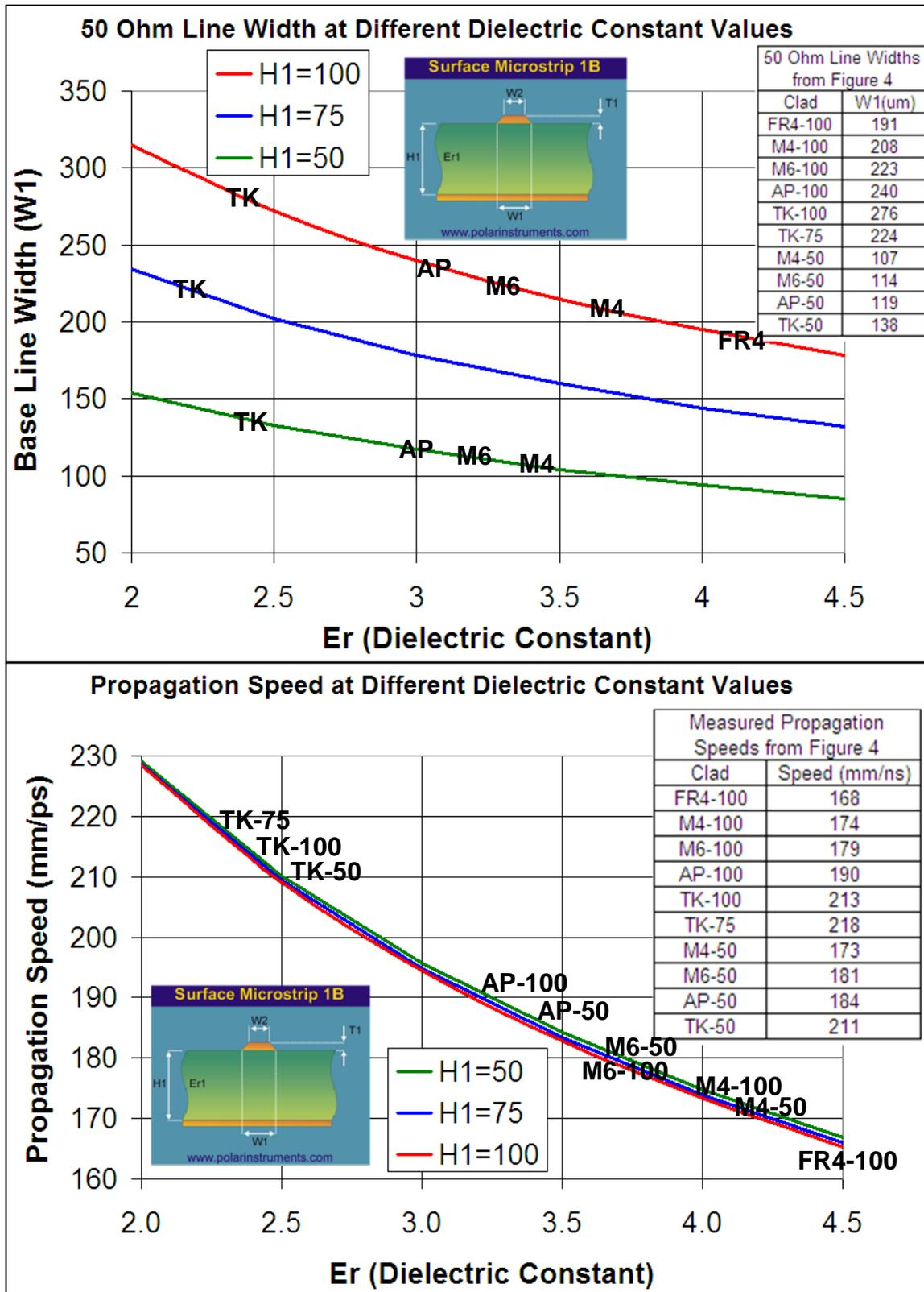
Figure 5 – Measured versus Calculated Line Width (um) and Propagation Speed (mm/ns)
