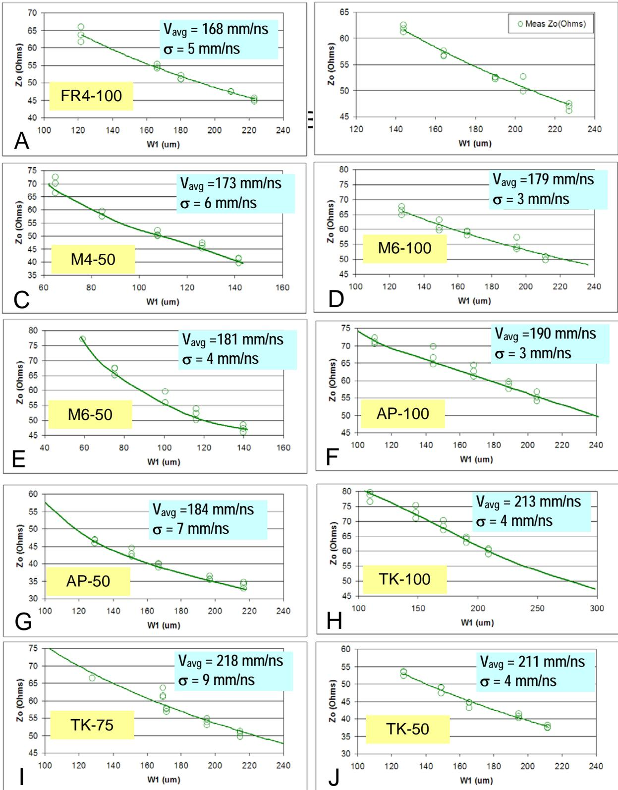
Figure 4 – Propagation Speed and Impedance as a Function of Line Width
