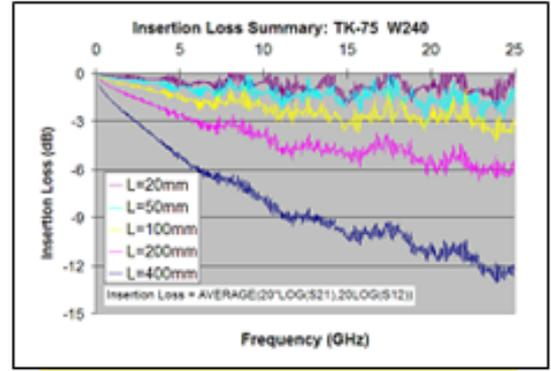
Insertion Loss from S21 and S12 of one width (5 lines)
