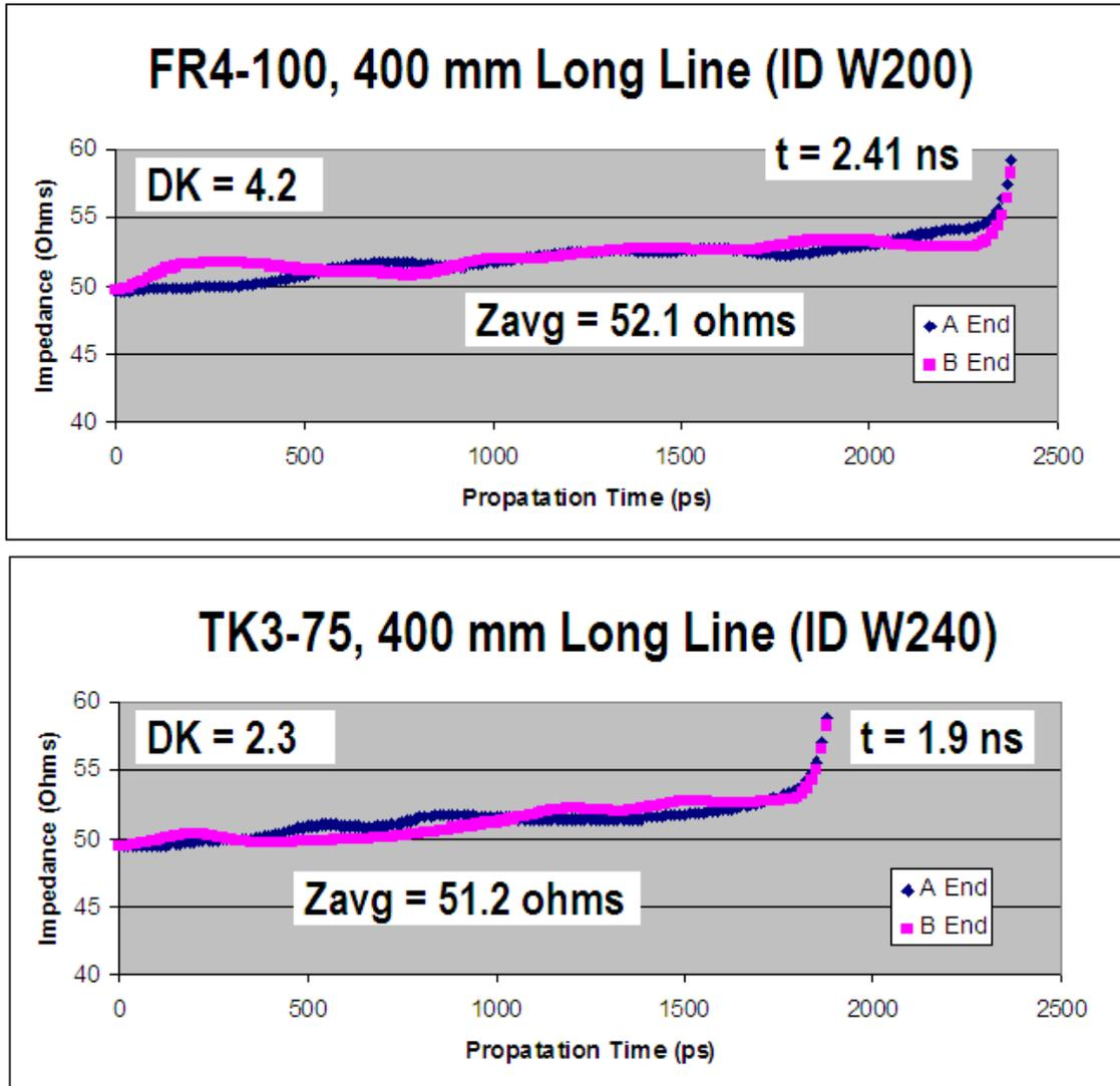
Figure 3 – Examples Showing How Impedance and Propagation Time are Determined
