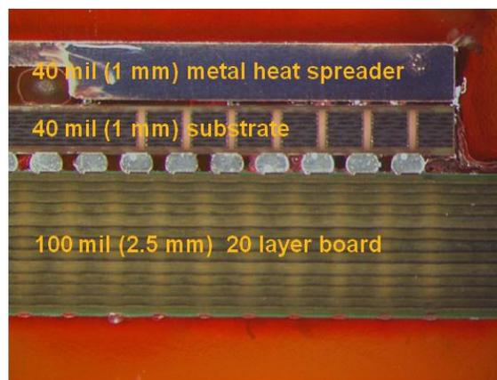
**Figure 4: Typical structure- 40 mm pkg on 20 layer board**
