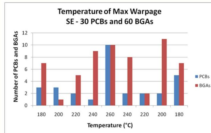
**The Max deformation did not always occur at the highest temperature nor at any one temperature**
