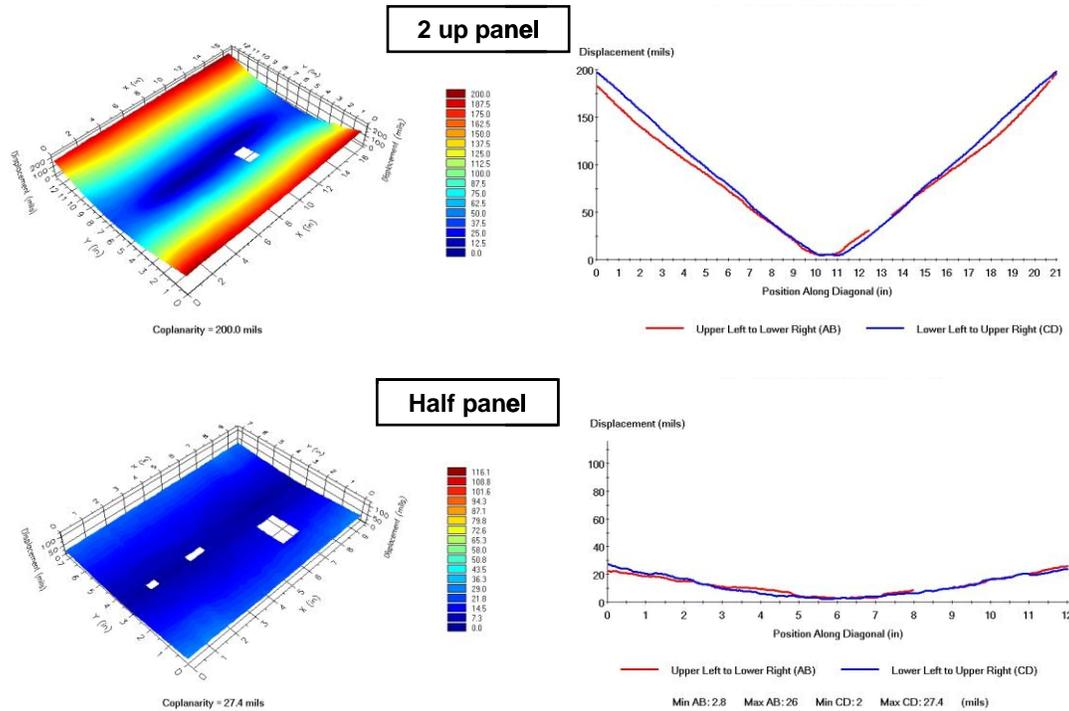
**Figure 03: Effects of Gravitational Sag**
