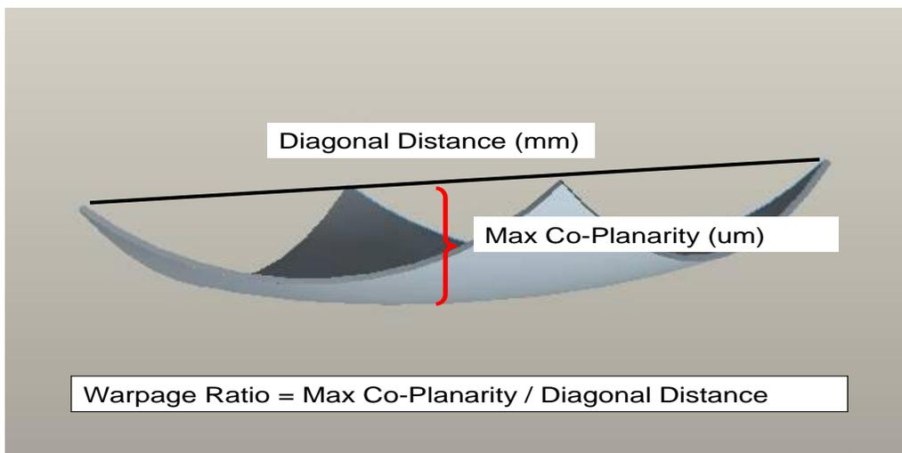
**Figure 02: Coplanarity Ratio Diagram**
