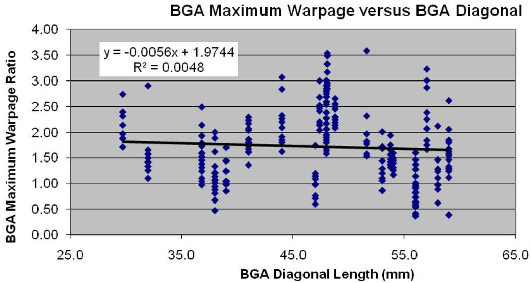
**Figure 09: BGA maximum Warpage as a function of BGA diagonal length**
