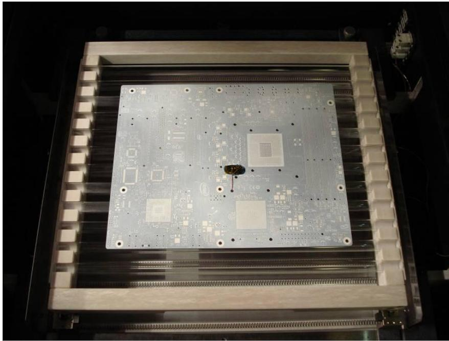
**Figure 01 Painted Sample on UAS Fixture**
