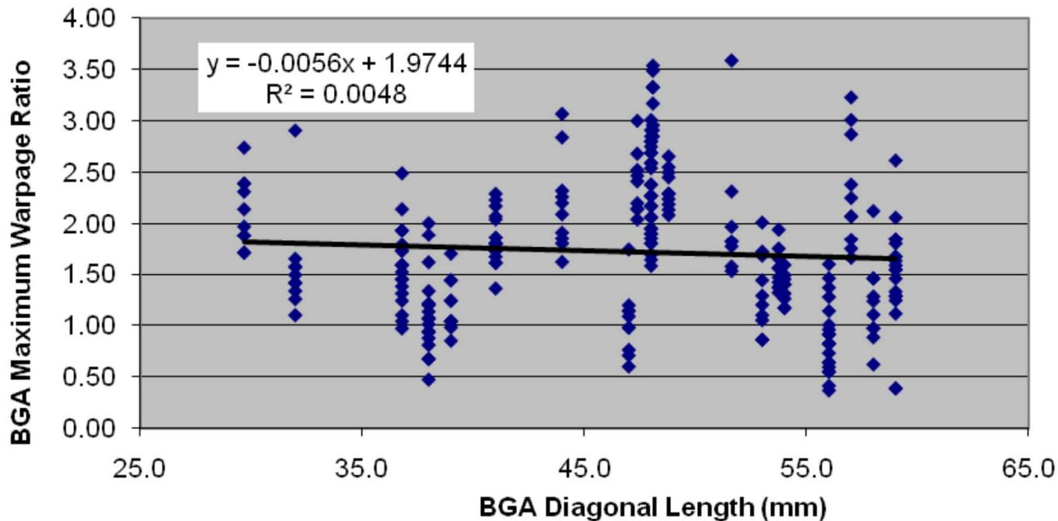
**It would be difficult to use one BGA coplanarity to predict the coplanarity of another BGA size**
