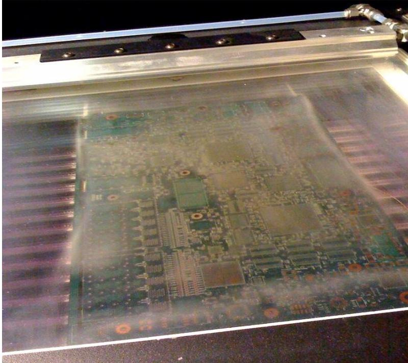
**Figure 05: Outgassing vapors on the grating glass.**
