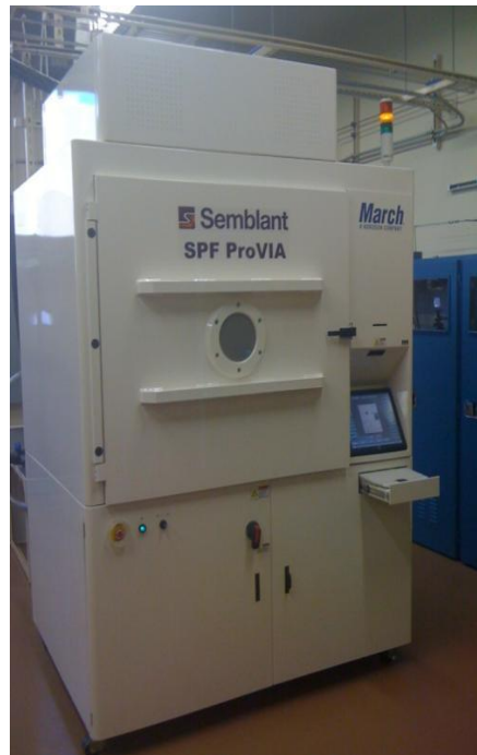
Figure 1- Plasma deposition system suitable for the volume production of plasma finished PCB panels
