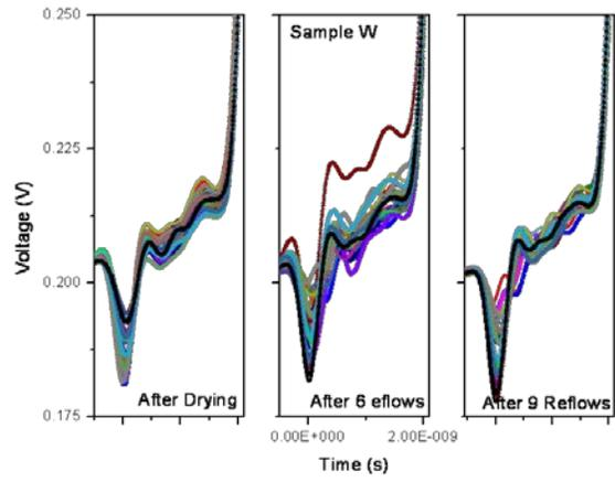
Fig. 14 TDR impedance result for sample W
