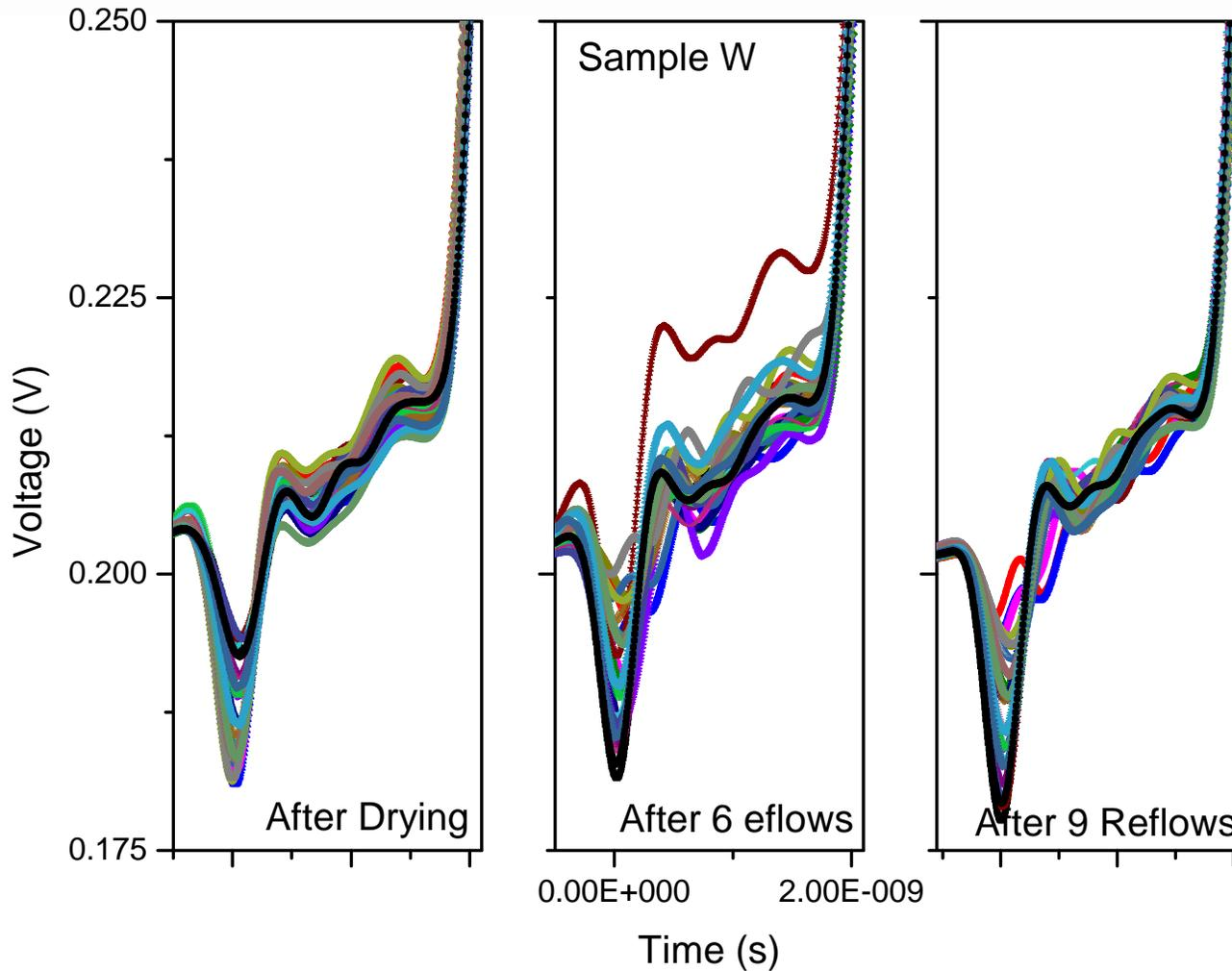
Sample W showed severe delamination but no change in TDR impedance
