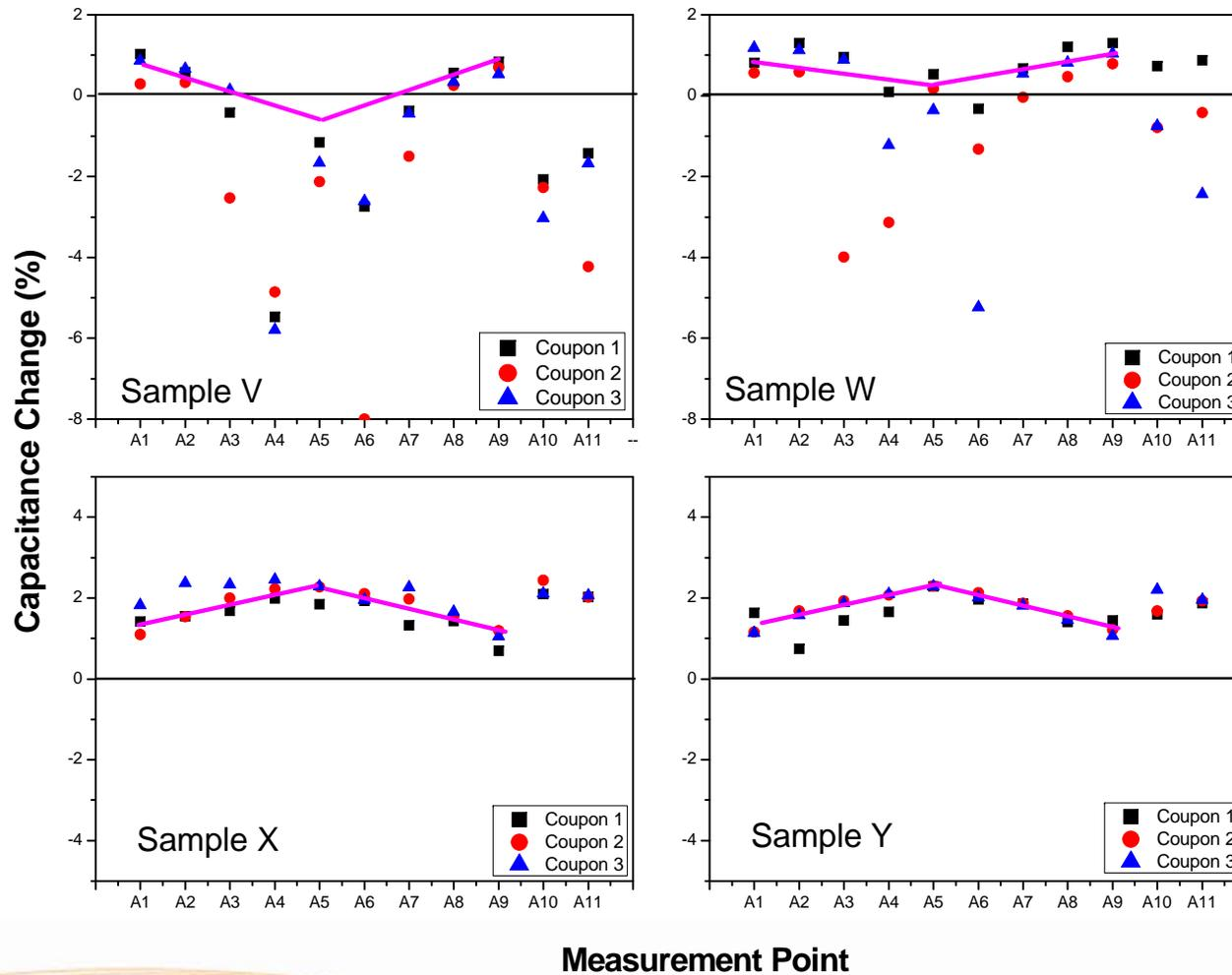
No deviation from magenta lines is see for samples X and Y: no delamination.
