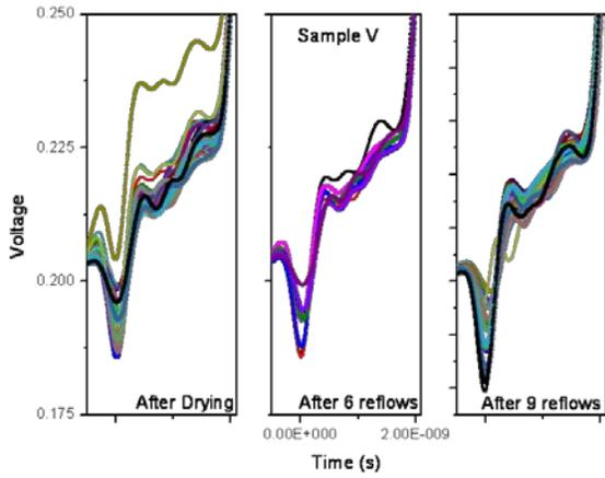
Fig. 13 TDR impedance result for sample V
