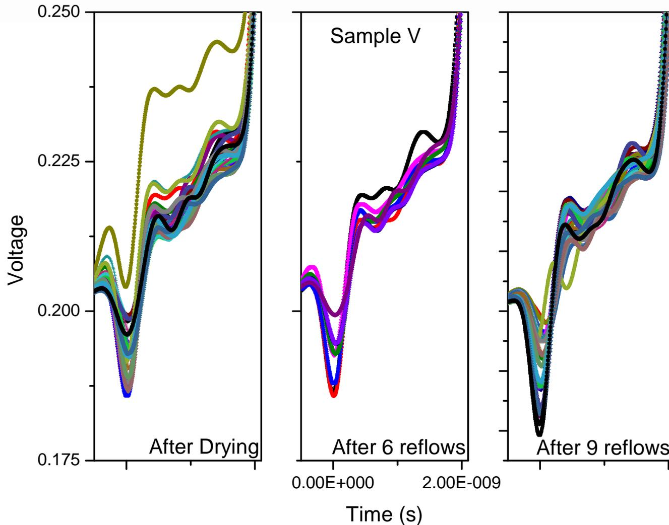
Sample V showed severe delamination but no change in TDR impedance
