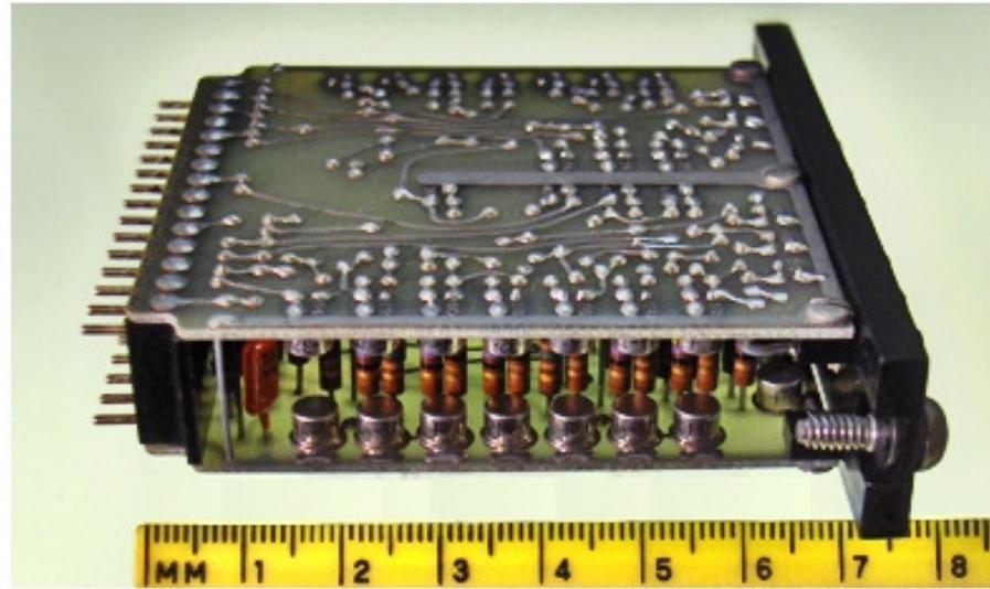
A “cordwood” module built by Control Data Corporation was developed to minimize connecting wire lengths and used a 3D stacked printed circuit arrangement to make electrical interconnections.
