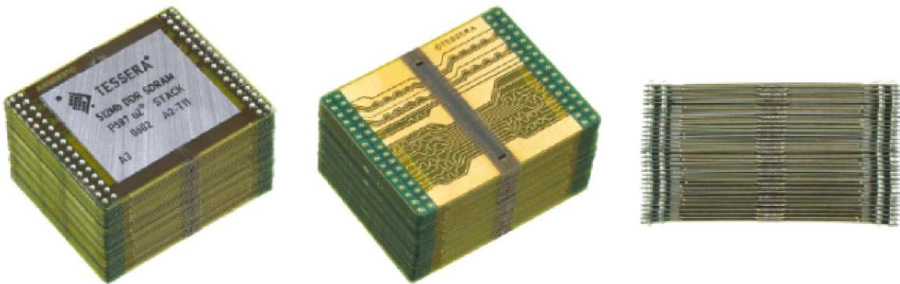
**Figure 4** Top, bottom and side views of an extreme example of package stacking
