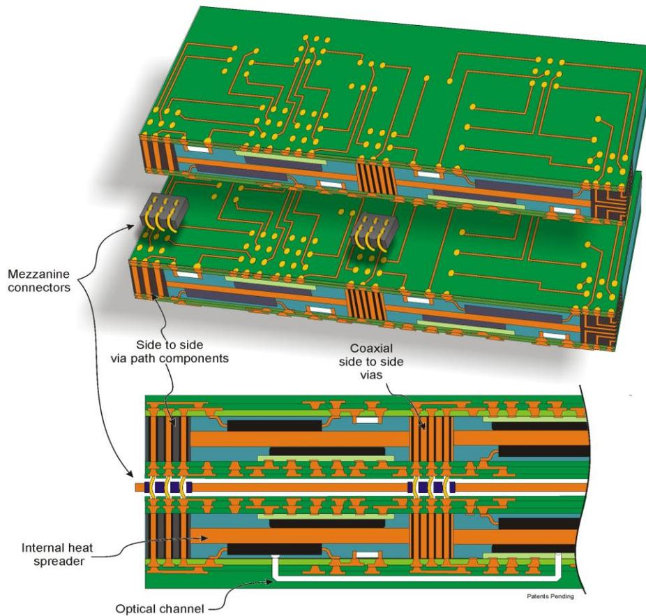
**Figure 9** Solderless assembly of electronics, an “inverted” 3D process is an area of growing interest due to the many advantages that it prospectively presents including optical channels built into the assembly. The assemblies can be joined together in a 3D stacked manner to provide true Manhattan, shortest path routing and the potential to address thermal issues on the front rather than the back end of the design process.
