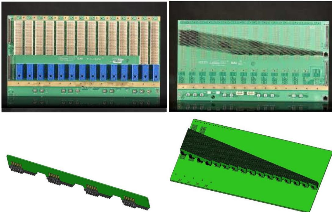
**Figure 5** A newly developed approach to backplane design improves performance by routing high speed channels separately from the rest of the circuits of the board. Top row left and right images are front and back side views respectively and on the bottom left and right show an example of one of the vertical circuits and a perspective view of the back side of an assembly. The overall height is low enough profile for use in many current systems.
