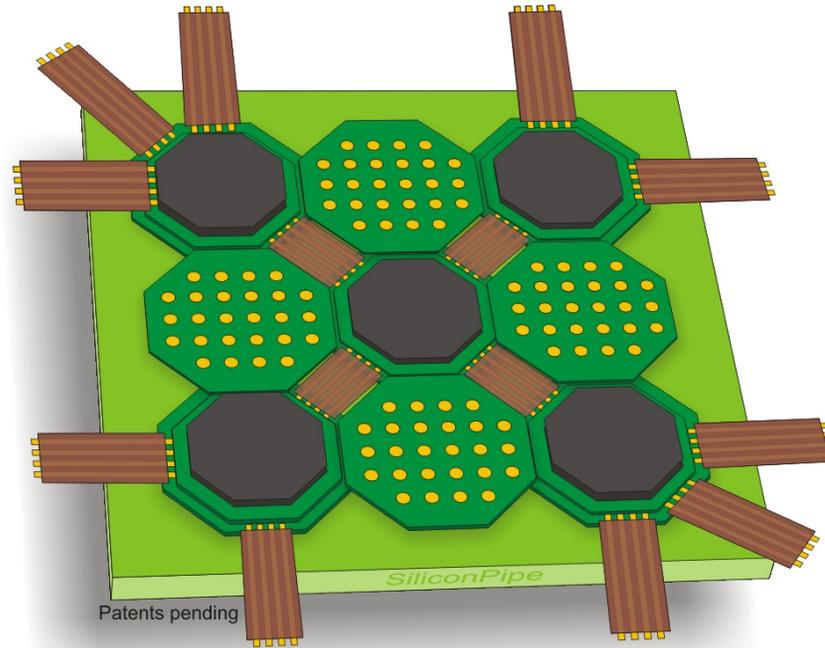
Flex for power, ground and high speed signals
