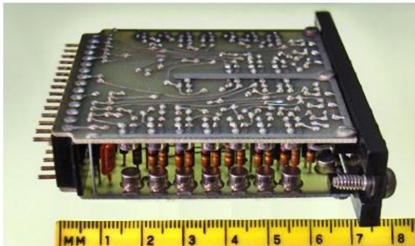
**Figure 1** A “cordwood” module built by Control Data Corporation was developed to minimize connecting wire lengths and used a 3D stacked printed circuit arrangement to make electrical interconnections.
