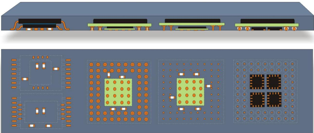
**Figure 8** Overlapping of packages and discretives is another prospective 3D solution which could be employed. Such devices could be either surface mounted as a component or embedded in an inverted or reverse 3D structure. (Source: Verdant Electronics, Inc)
