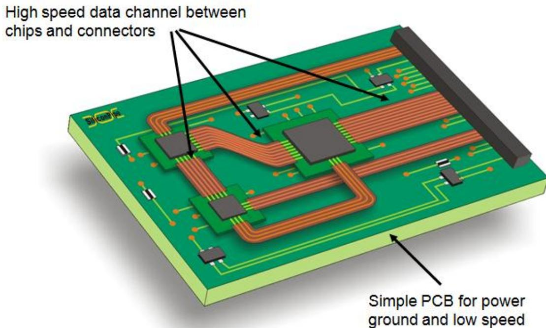
**Figure 7** Making interconnections directly between IC packages has been shown to greatly improve circuit performance while simultaneously reducing system power requirements
