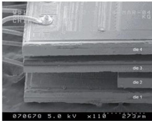
**Figure 3** Stacked chip packages can help significantly conserve PCB real estate and with the use of thinned die, very little penalty in the Z axis, however, die yields must be near perfect. Such structures are commonly employed to create system in package (SiP) alternative solutions to the time and expense of designing a complex chip.
