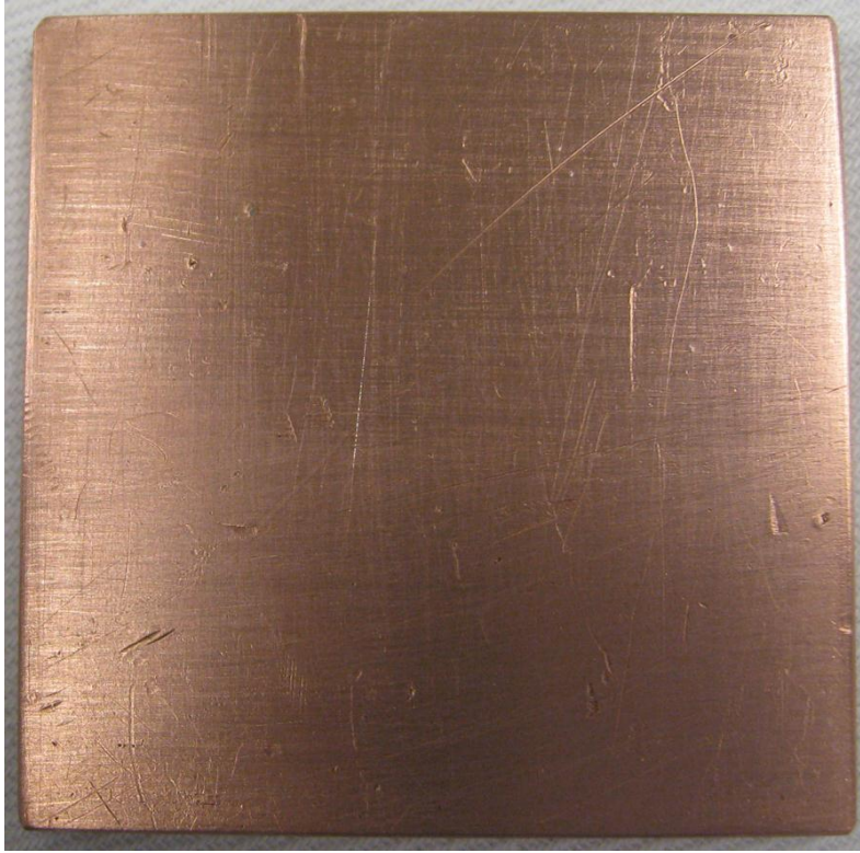
Figure 4: Example of a Cu Block Sample after Cleaning and before Solder Paste Deposit and Reflow.
