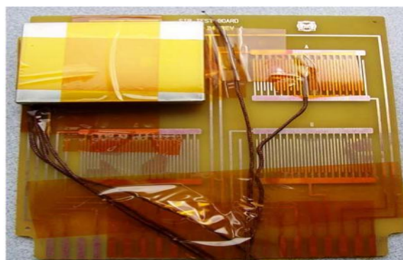
Figure 6 - Location of thermal couples for profiling of SIR board with RF shield
