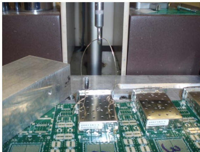
Pulled the press fit connector as shown.
