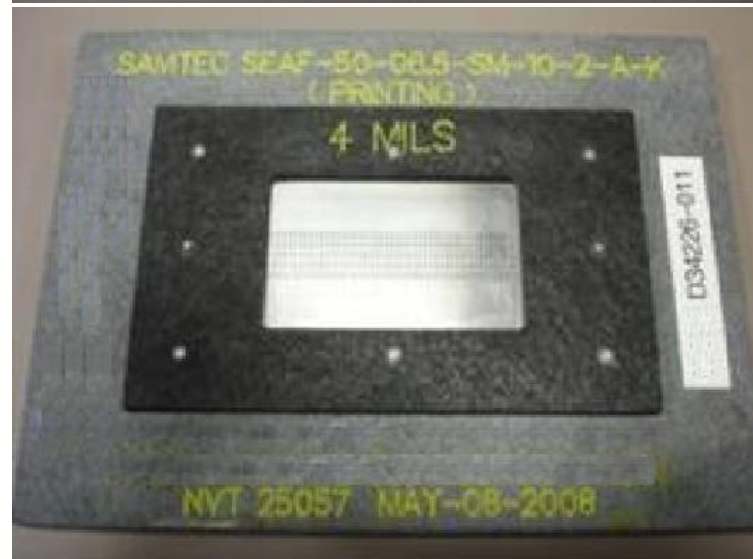
Mini stencil for additional solder for connector (additional 4 mils solder)
