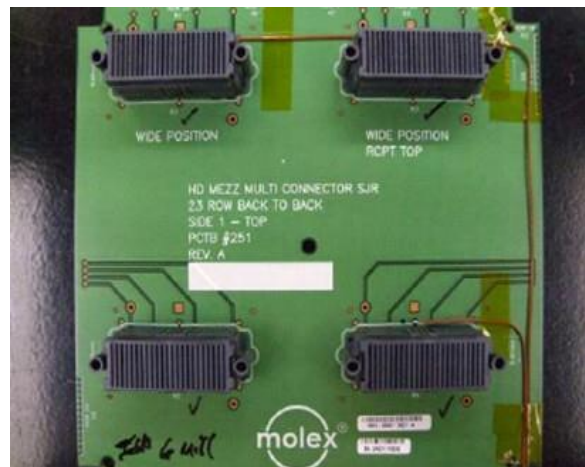
Figure 12: Test Vehicle Layout used for IPC-9701 Testing (Receptacle Side)
