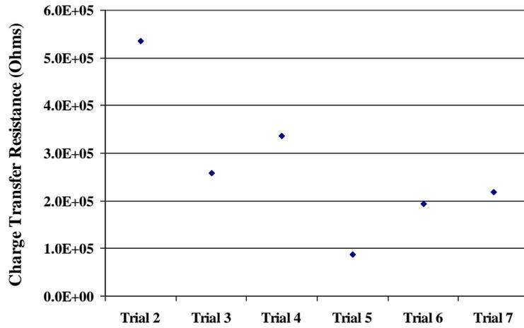
Figure 10: Change of charge transfer resistance  $R_{ct}$  during dendritic growth based on Table 3
