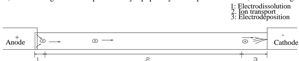
Figure 4: The electrochemical migration processes occurred on the surface of comb structure.
