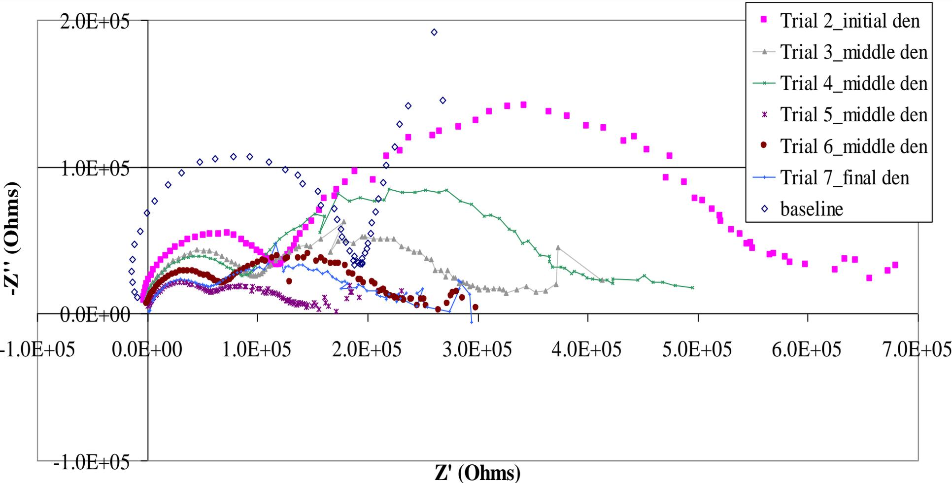
The two semicircles in the plot were shrinking on both real and imaginary axis in general as dendrites grew longer and denser, although in the middle of the process this shrinking trend may have reversed a couple of times.
