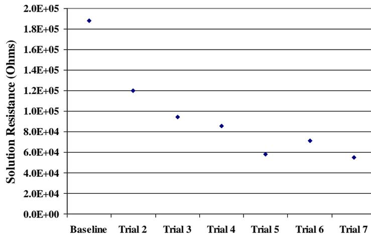
Figure 9: Change of solution resistance  $R_c$  during dendritic growth based on Table 2
