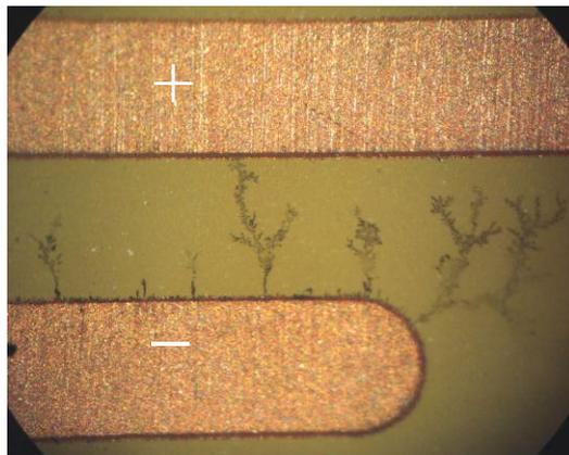
Figure 15: The final dendrites grown after the cyclic DC and AC applications.
