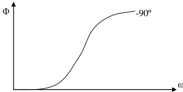
Figure 3: A typical phase shift plot for an R-C parallel circuit.
