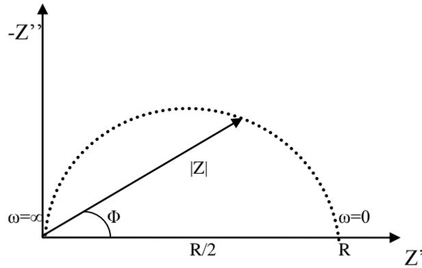
Figure 1: A typical Nyquist plot for an R-C parallel circuit.
