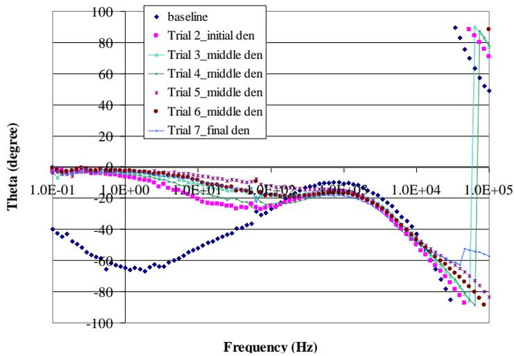
Figure 14: Phase angle plot during dendritic growth
