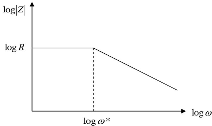
Figure 2: A typical Bode plot for an R-C parallel circuit.
