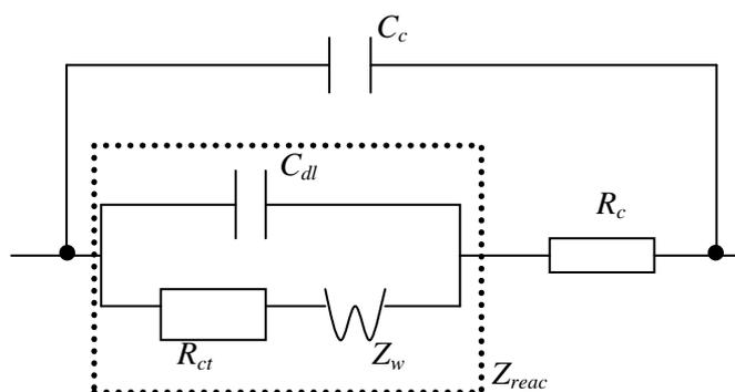
Figure 5: The equivalent circuit corresponding to Figure 4.  $C_c$  is electrical capacitance of the electrodes,  $C_{dl}$  is the double layer charging capacitance,  $R_c$  is the ionic transport resistance,  $R_{ct}$  is the charge transfer resistance, and  $Z_w$  is the Warburg diffusion resistance.
