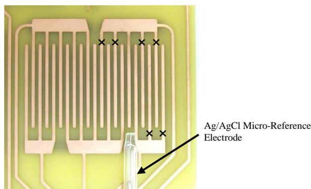
Figure 6: Comb structure and Ag/AgCl micro-reference electrode
