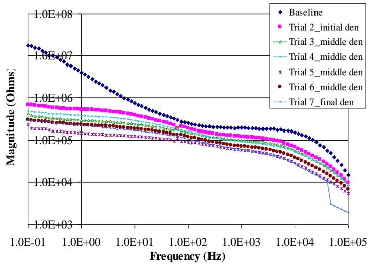
Figure 13: Bode plot during dendritic growth
