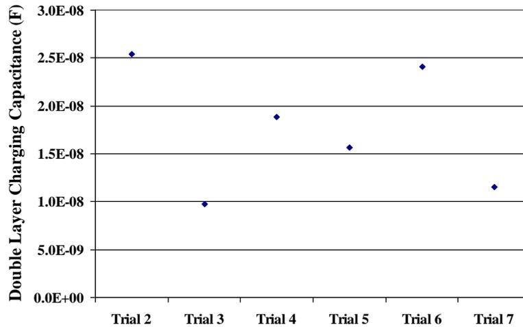
Figure 11: Change of double layer capacitance  $C_{dl}$  during dendritic growth based on Table 5
