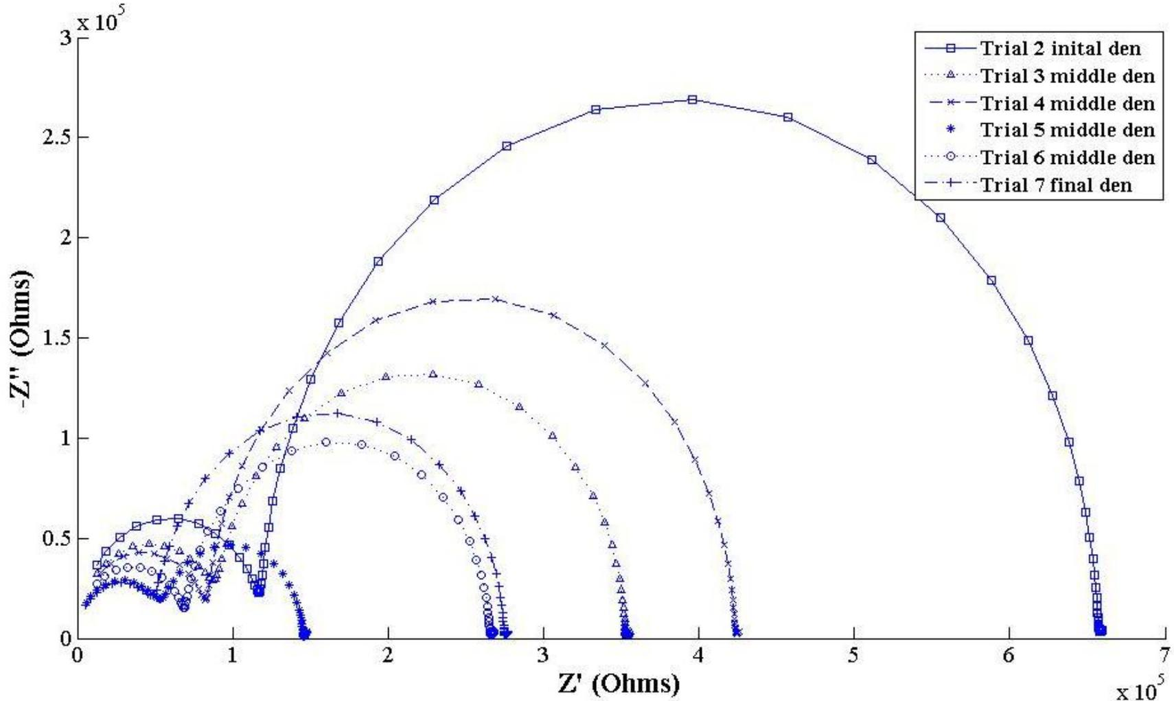
The two semicircles generally shrink although they reverse a little in the middle of the process, which confirms the experimental data.
