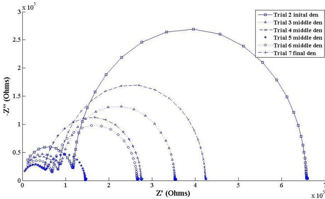
Figure 12: Simulated Nyquist plot during dendritic growth based on the extracted values  $C_c$ ,  $R_c$ ,  $C_{dl}$ , and  $R_{ct}$  from Figure 8
