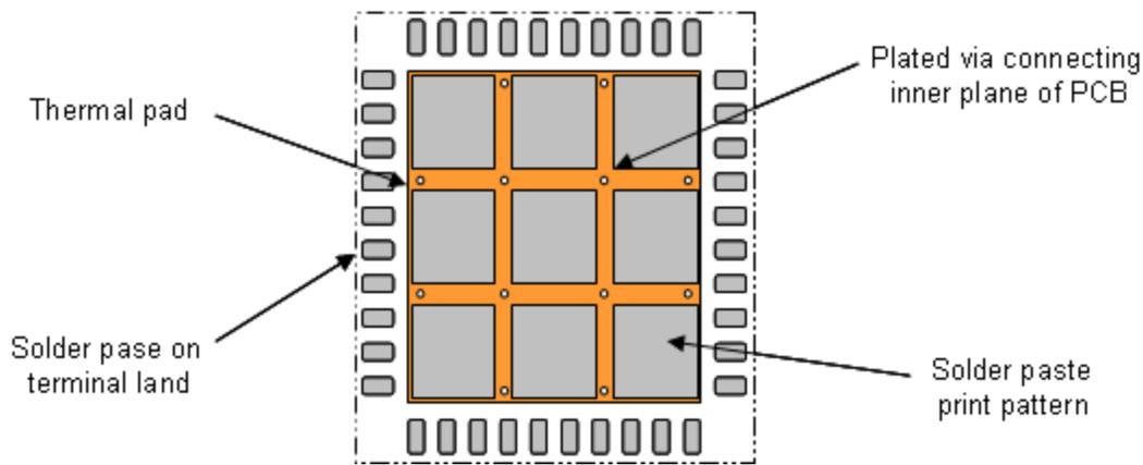
**Figure 9.** Segmented solder paste pattern with plated vias on thermal pad.
