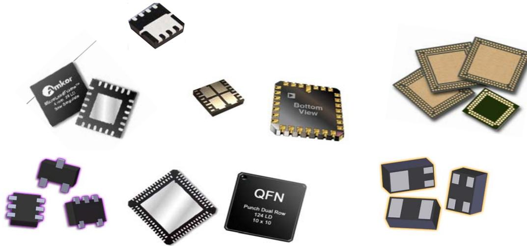
These semiconductor package variations go by such diverse names as Quad Flat Pack No-Lead (QFN), Land Grid Array (LGA), Small Outline No-Lead (SON), Plastic Quad Flat No-Lead (PQFN), Micro Lead Frame Plastic (MLFP™), Micro Lead-Frame Package (MLP™) and many more.
