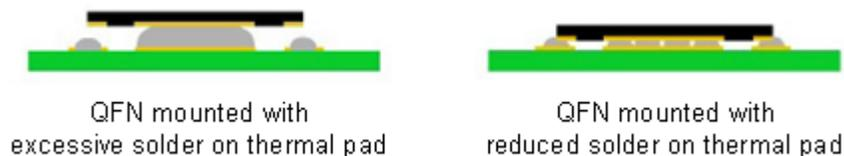
**Figure 8.** The affect of depositing a single solder paste pattern to a segmented pattern on the thermal pad.
