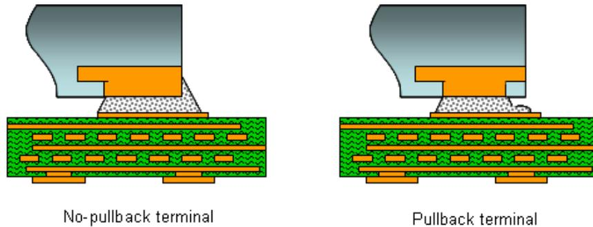
**Figure 4.** Land pattern to terminal alignment.
