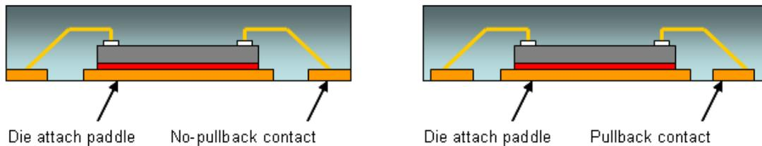
**Figure 2.** Terminal-to-edge variations for BTC semiconductor packaging.
