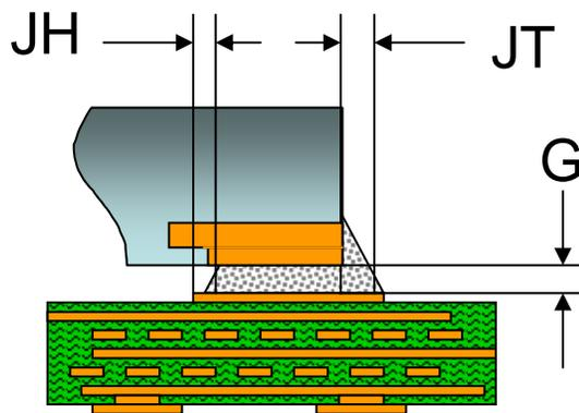
Solder fillet on coated or plated terminal end
