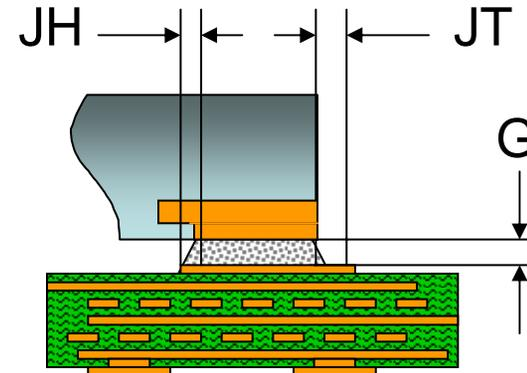
Solder fillet on bare Cu terminal end with oxidation build-up
