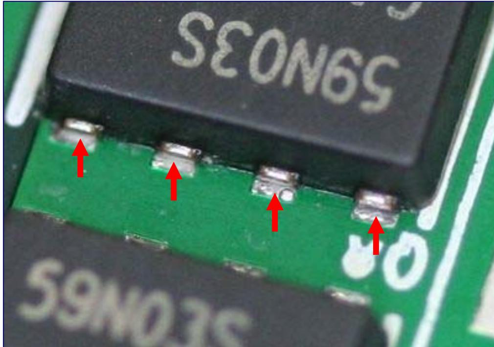
Due to the singulation process, the exposed copper terminal end surfaces are not required to be solderable therefore, a toe fillet is not a requirement.
