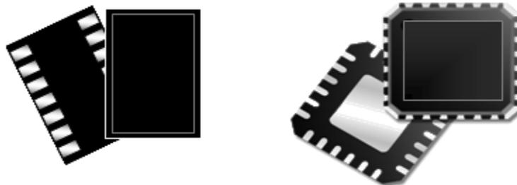
**Figure 1.** Comparing SON and QFN bottom termination semiconductor packaging.
