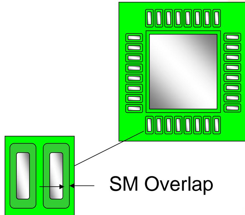
*For SMD applications, the mask opening should be approximately 100 microns smaller than the land and thermal pad to overlap the land and thermal pad on all four sides.*
