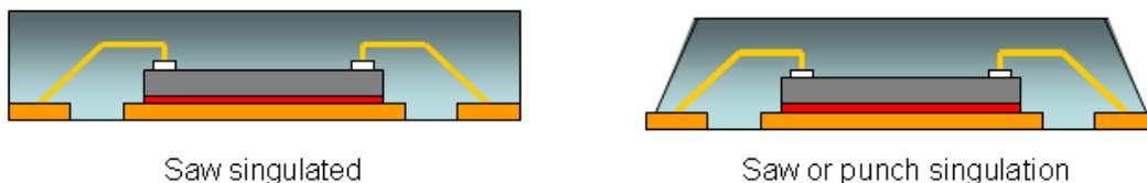
**Figure 3.** QFN/SON monolithic and tapered edge overmold profile variations.
