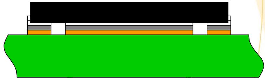
*Rather than coagulating in the center of the thermal pad during reflow soldering, the partitioned solder pattern will maintain a uniform interface between surfaces.*
