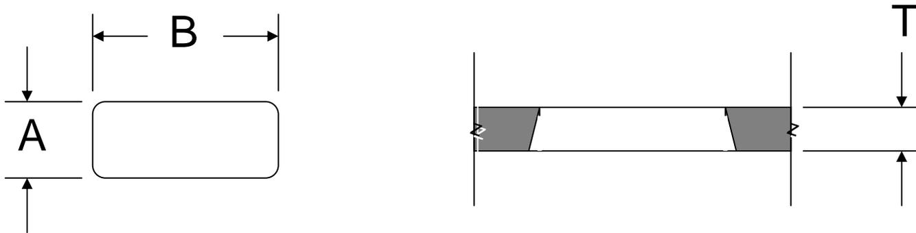
$$(A \times B) \times T = \text{solder paste volume [1]}$$
