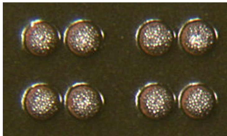
Supplier A Elliptical SMD Pads
