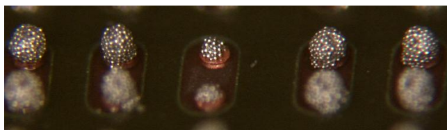
Supplier A (over-etched copper)
