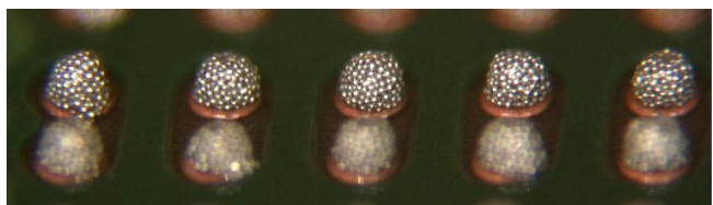
Supplier B (correct copper size)
