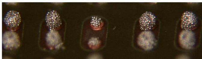
Supplier A (Over-Etched Copper)
