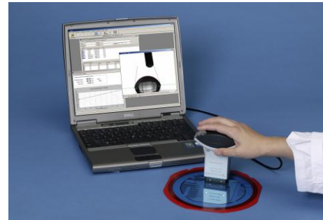
Figure 5 – computer assisted contact angle equipment
