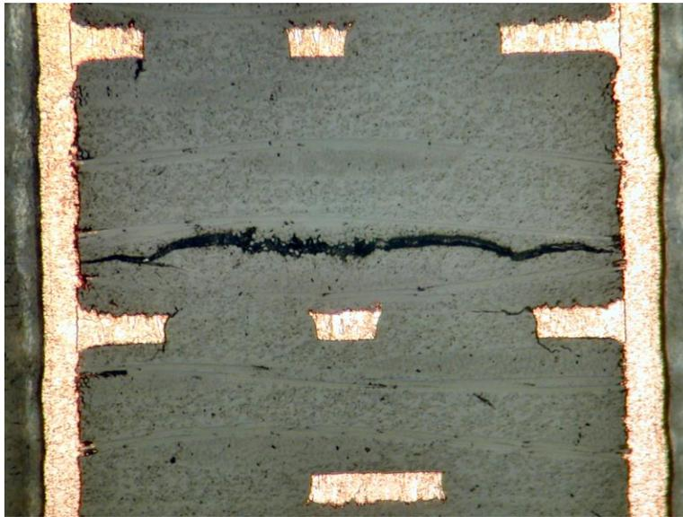
**Figure 9: Example Snake Delamination**
