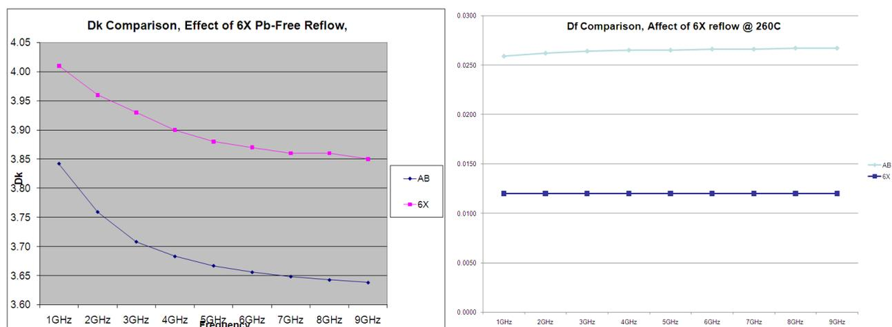
**Figure 9: Typical plot of Dk over frequency (left) and Df over frequency (right). These two plots are shown where the changes in the materials after reflow are major.**
