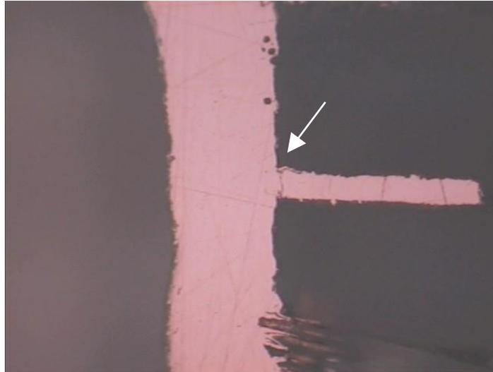
**Figure 11: Example of foil crack through entire width of inner layer**
