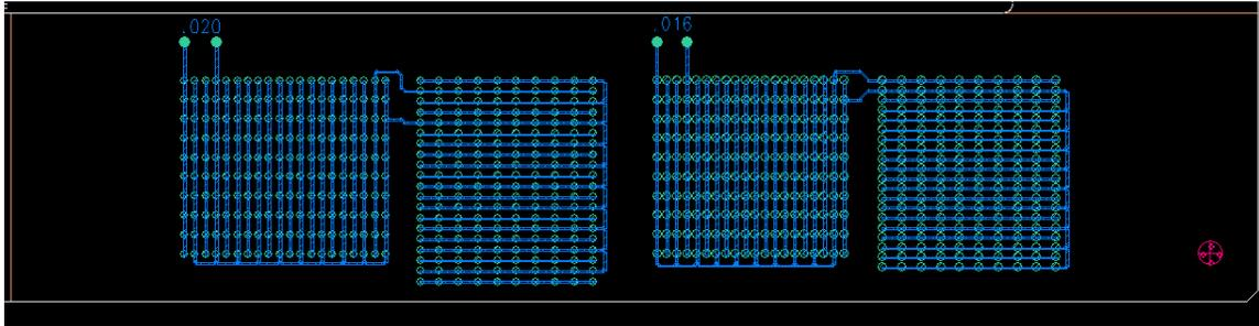
**Figure 22: Through Hole Wall-Wall CAF test section**
