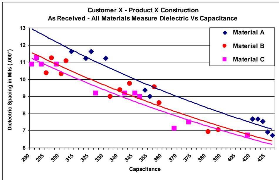
Figure 18: All Materials – Dielectric vs. Capacitance
