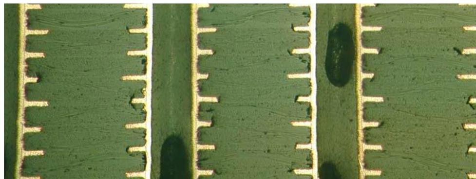
**Edge delamination, Visible internal delamination, Hidden delamination between vias, Vertical Eyebrow cracking**
