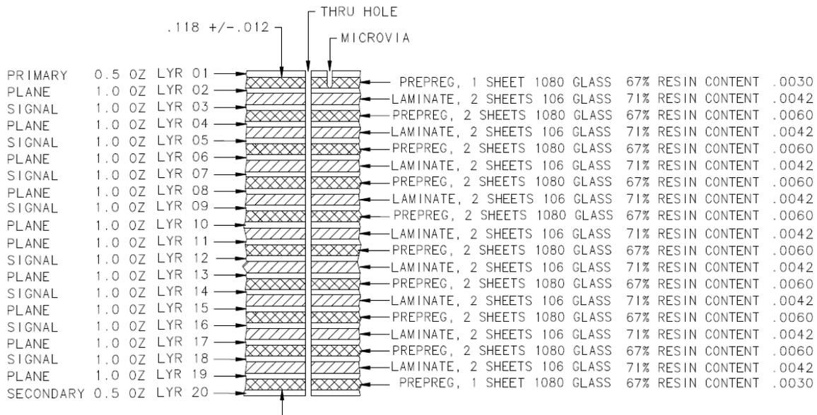
**Figure 3: Figure 3, 20 layer, 69% resin construction**
