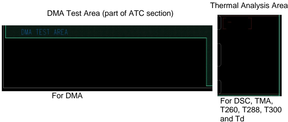
**Figure 25: Close of the DMA and Thermal Analysis Test areas shown in figures 4 and 5. Note that they are void of copper on all layers.**
