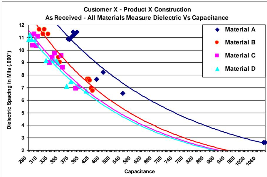
Figure 17: Dielectric vs. Capacitance
