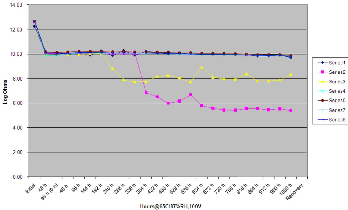
Figure 23: Typical CAF data plot, showing first failures at 240 hours
