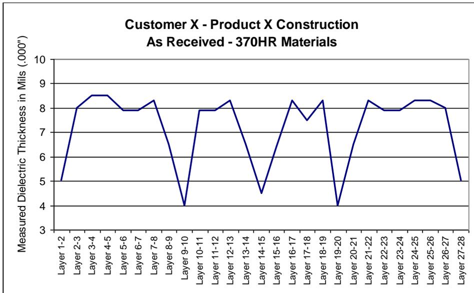
Figure 16: Construction Profile – Estimated Dielectric Thickness
