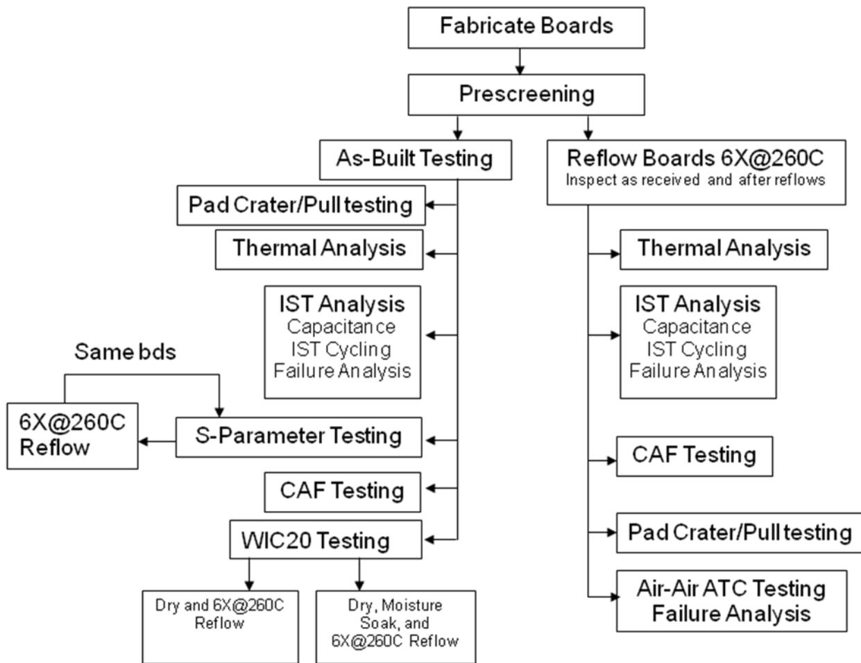
Of the as built boards, one entire board is dedicated to thermal analysis. The remaining nine are separated into their various sections and the following sections/coupons are required for each test:
