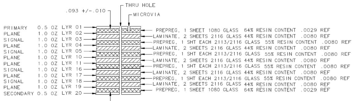
Figure 1: 12 layer, 50% resin construction
