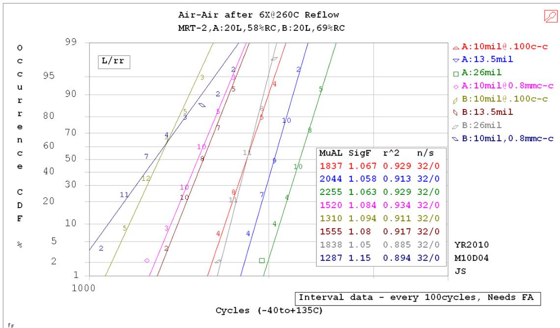
**Figure 12: Log Normal plots of air-to-air failure data showing a slope change on the 0.8mm pitch construction with 69% resin content**
