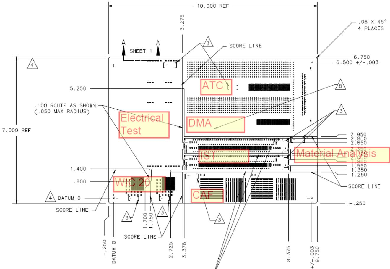
Figure 4: Plan view from the fabrication drawing with added identification showing each of the seven different sections on the test board.
