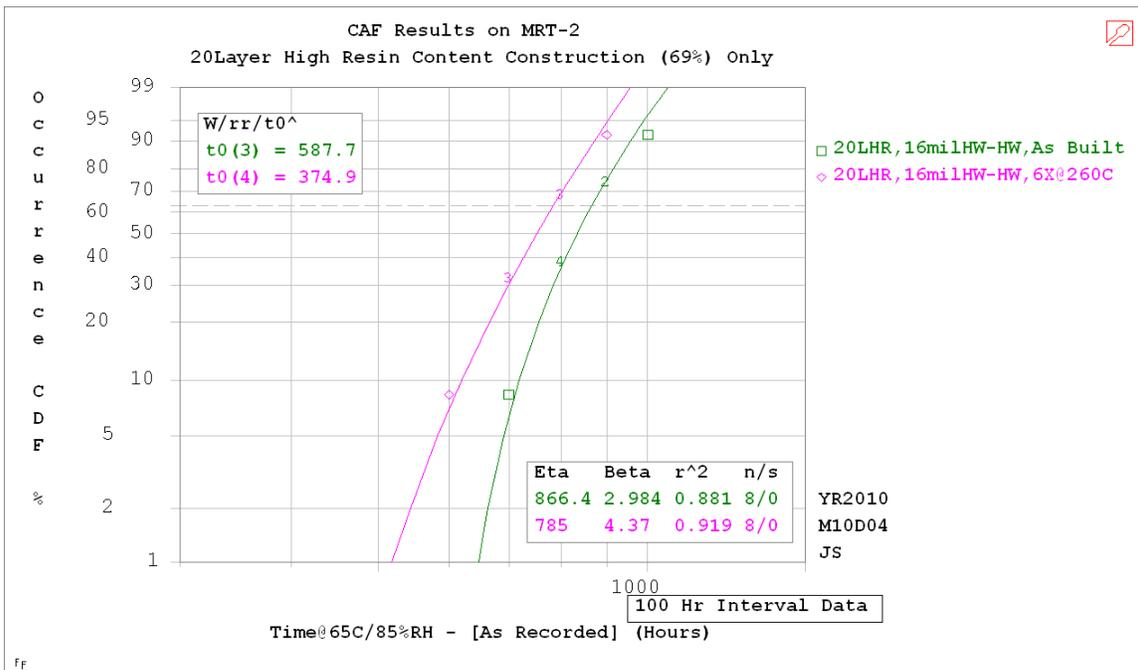
Figure 24: 3 parameter Weibull plot of CAF data showing degradation of CAF performance after Pb-free reflow.
