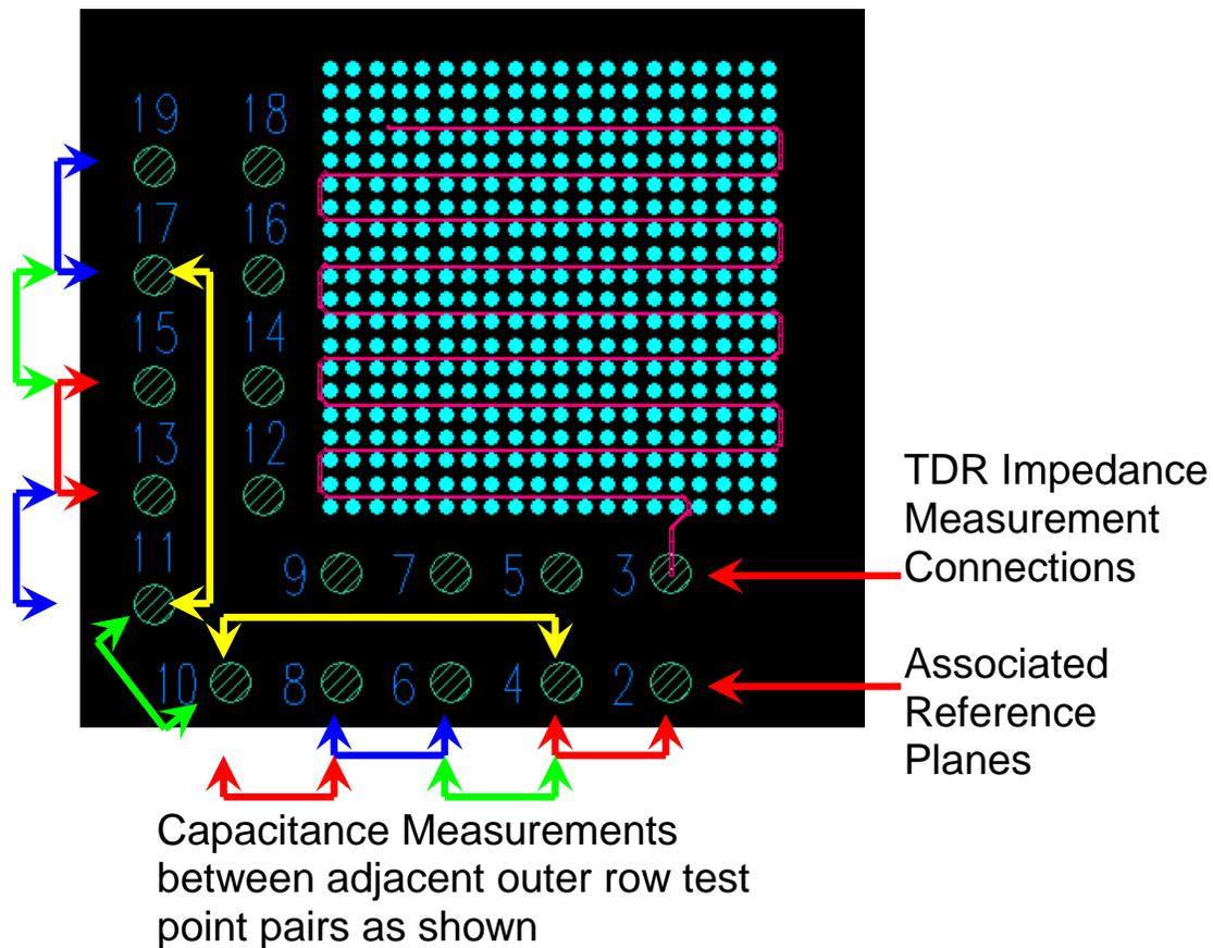
Figure 26: Example of WIC-20 Coupon. Layer 1 and Layer 3 shown.
