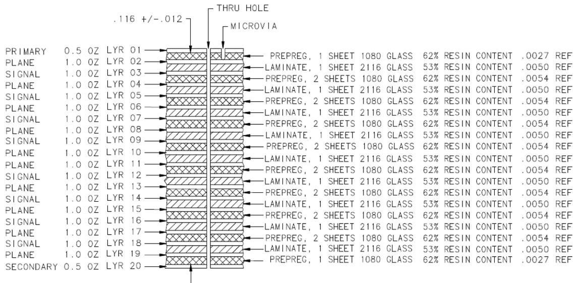
**Figure 2: 20 layer, 58% resin construction**
