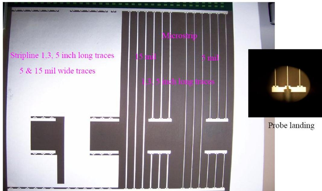
**Figure 8: Electrical Test Section of the Test Board**
