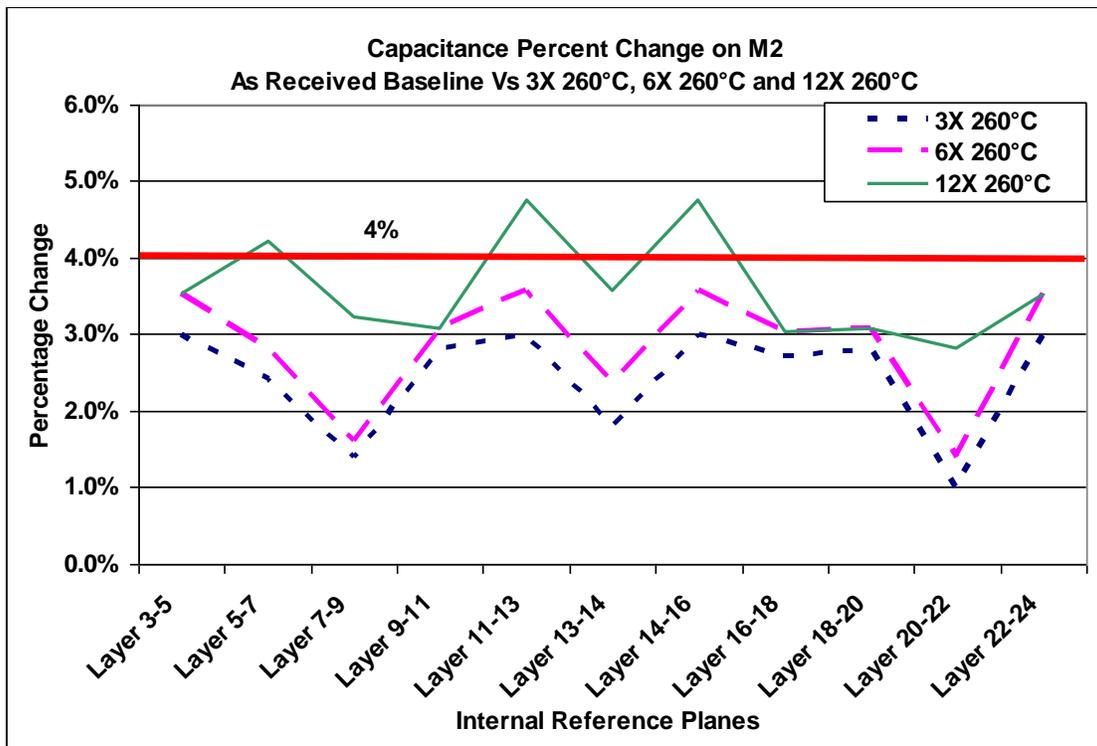
Figure 20: Example of Capacitance change on the M2 circuit with reflow, showing material degradation.
