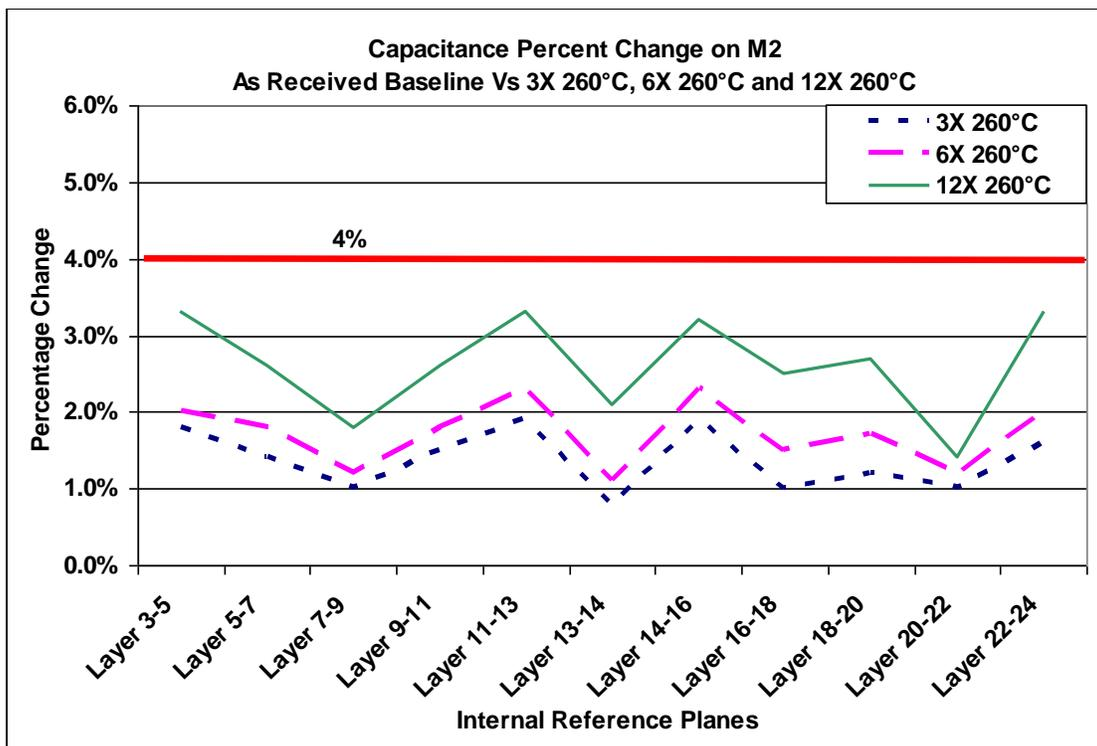
Figure 21: Example of Capacitance change on the M2 circuit with reflow, showing excellent performance.
