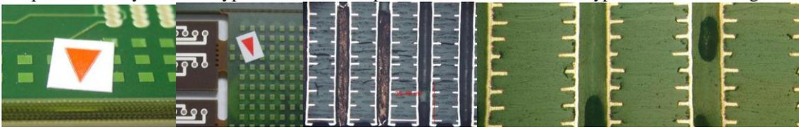
**Figure 7: Left-to-right: Edge delamination, Visible internal delamination, Hidden delamination between vias, Eyebrow cracking**
