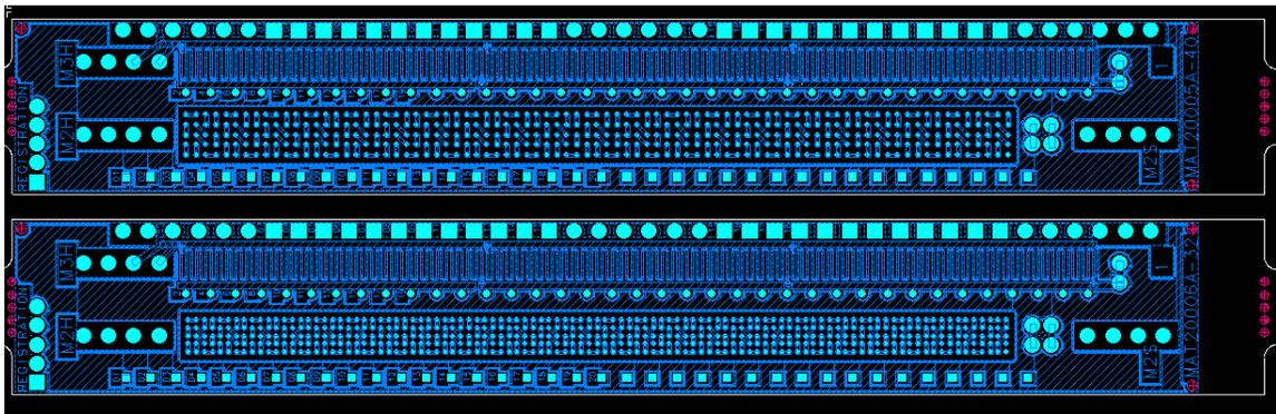
Figure 13: The two IST coupons used on the MRT-5 design.
