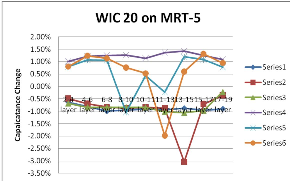
**Example plot of capacitance changes after reflow compared to before reflow. In the above example, Series 1,2 and 3 are “dry” (after 24 hours @125° C° ) and then reflowed, and Series 4, 5, and 6 are “wet” (after 168 hours of 85° C/85%RH). Series 2, 5 and 6 are clearly indicating internal material damage.**
