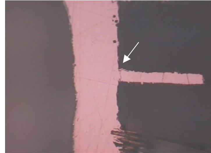
Foil Crack Failure Mode
