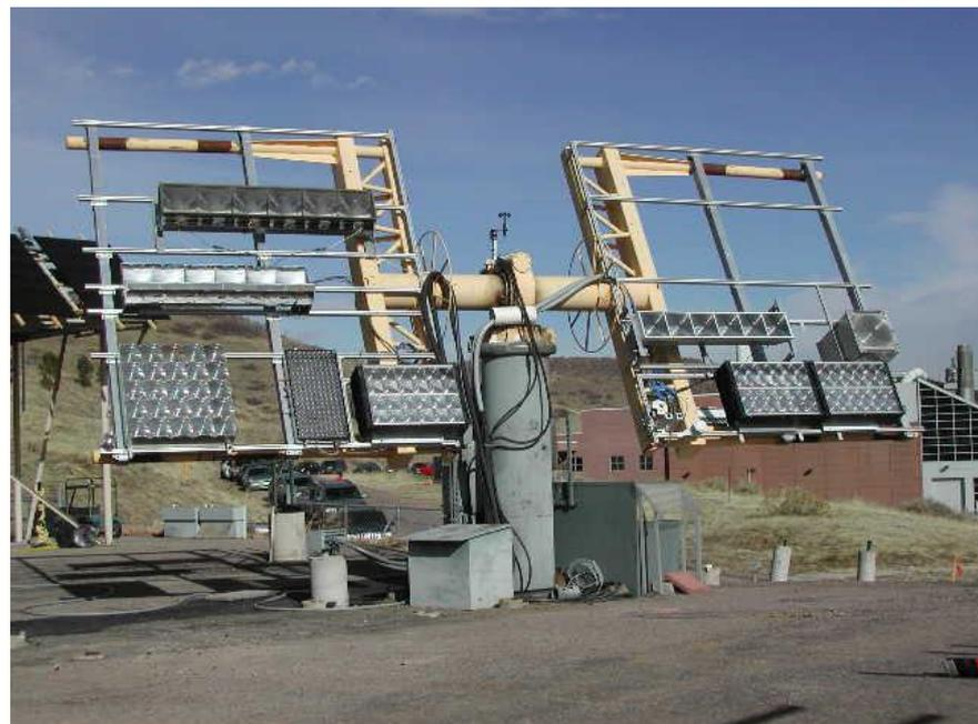
Two-axis tracker at NREL with CPV modules from Boeing, Concentrix, GreenVolts, Arima, and Opel.
