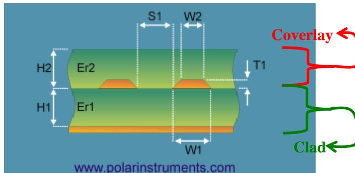
**Figure 1** – Basic differential microstrip structure used.
