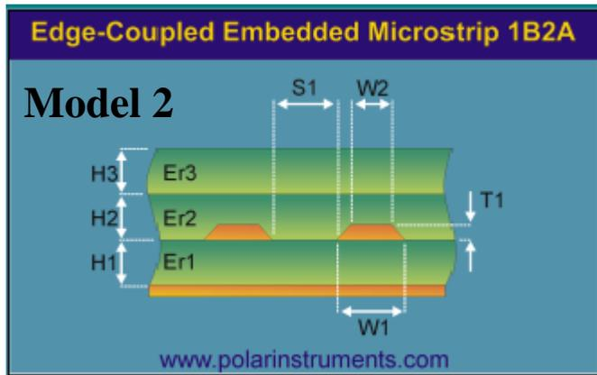
**Figure 3** – Polar SI9000 models used to evaluate impedance.
