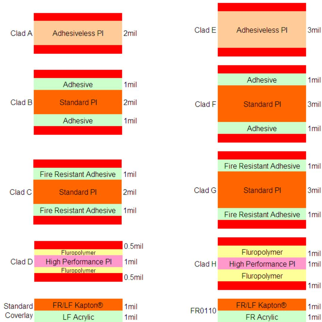
**Figure 2** – Detailed descriptions of copper clad laminates and coverlays used in test
