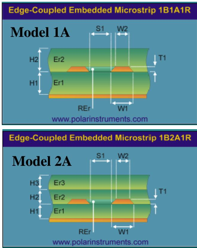
**Figure 8** – Alternate Models for Boards Using Non-Acrylic Laminates
