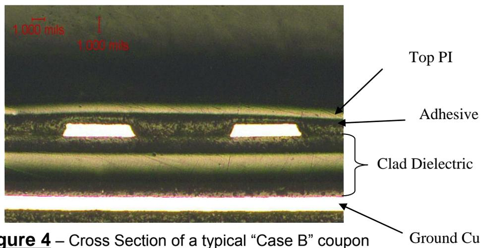
**Figure 4** – Cross Section of a typical “Case B” coupon
