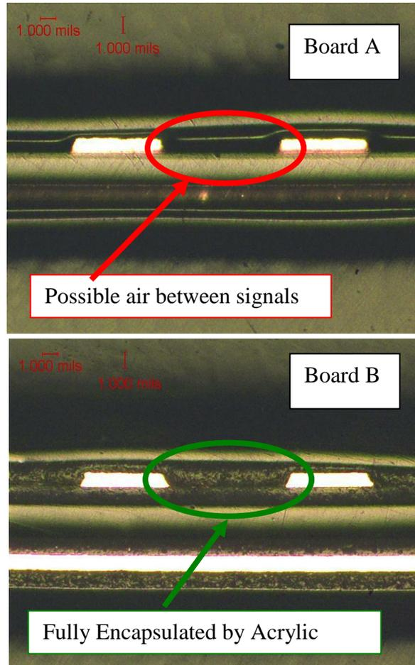
**Figure 7** – Cross Section Comparison of All Polyimide versus Acrylic Based Laminates
